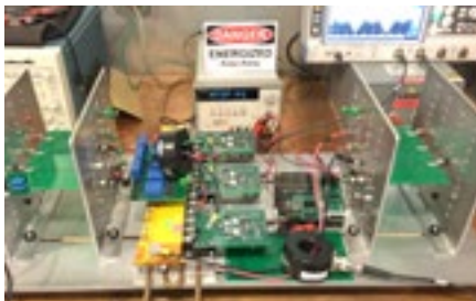
Three-phase inverter system used for validating EMI models.
