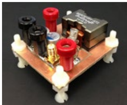
Double pulse tester for DrGaN
