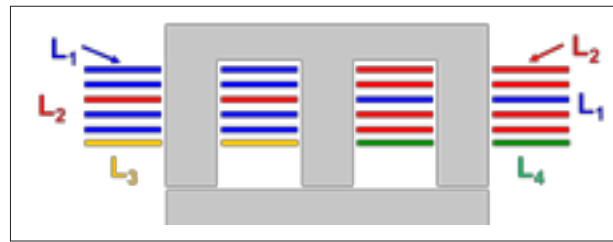
Fig. 1. Inductor core structure (principle drawing).
