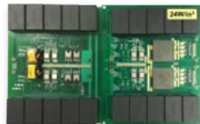
A 6.6kW 500kHz Level 2 on board battery charger is built using a novel variable DC-link voltage structure.
