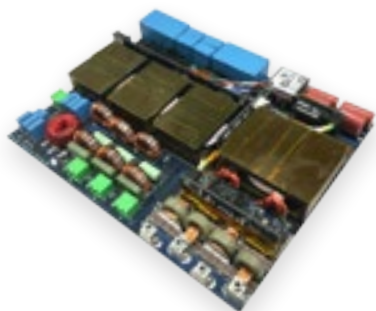
Prototype of a 1.2 kW three-phase isolated AC/DC converter with 97% efficiency and 22W/in 3 power density.
