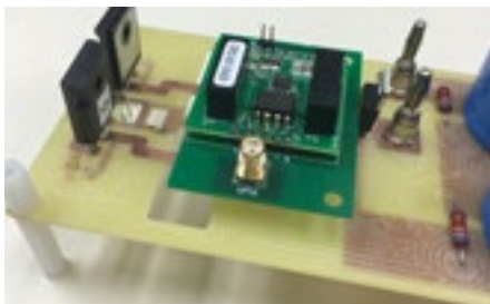
Double-pulse tester for current balancing
