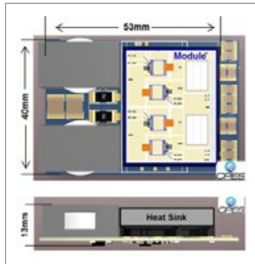
Fig. 2. New design of PFC rectifier with a highly integrated MCM including 4 cascode GaN devices and 2 low-speed Si MOSFETs.
