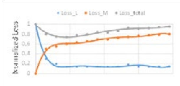
Fig. 2. Calculated inductor loss with different coupled inductance M (normalized to total loss without coupled inductor).
