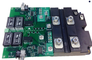
Gate Driver for 3.3 kV 400 A Full SiC MOSFETs
