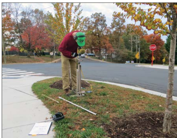
At a street tree planting site in Arlington County, Virginia, former master's student David Mitchell uses a specialized probe to extract a column of soil 1 meter deep. Soil carbon was analyzed at sites with and without remediation.
