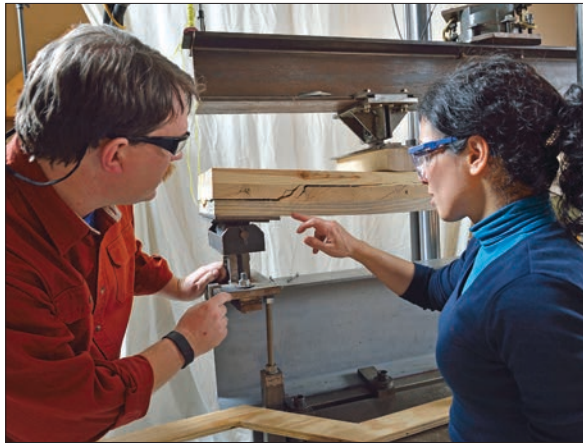
Daniel Hindman (left) and doctoral student Hourli Sharifniay examine failures in a southern pine cross-laminated timber beam during testing.
