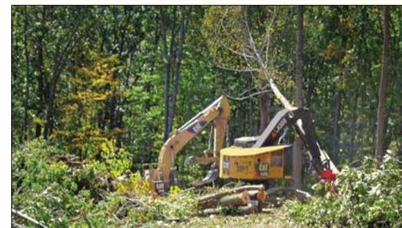
Extension Agent Bill Worrell helped plan the first-ever tour in Lee County in the far southwest corner of the state, where participants got to see a low-impact feller buncher (pictured) cut trees and move them to a log landing for loading onto a truck for transport. Also on the tour was a visit to the B.J. Fortner Hardwoods mill, where the family-owned business demonstrated its commitment to sustainable forestry and showed how high-quality logs are cut into lumber and graded for the veneer export market.
