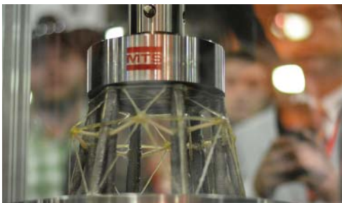
MS&T: The Geodesic Dome Competition winner, an aluminum and fiberglass composite, maxxed out the compression testing machine, supporting 55,000 N.
