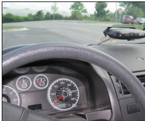
Figure 2. Photo. MiniDAS installation location.
