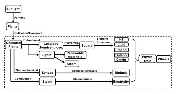
Figure 1. Different pathways for biofuels production from lignocellulosic biomass. The current energy efficiency analysis focuses on the delivered biomass-to-wheel efficiency related with conversion, transportation and power train systems. doi:10.1371/journal.pone.0022113.g001
