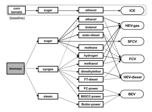
**Figure 3. Scenarios of the production of fuels from biomass and their respective fuel power train systems.** Solid lines represent the scenarios that we analyzed; the dotted lines represent possible scenarios that we did not analyze. doi:10.1371/journal.pone.0022113.q003
