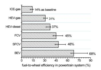
Figure 6. Comparison of fuel-to-wheel (FTW) efficiency for different powertrain systems. doi:10.1371/journal.pone.0022113.g006
