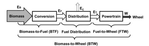
Figure 2. The scheme of energy efficiency analysis for biomass-to-wheel efficiency calculation --  $\eta_{BTW} = \frac{W}{E_B} = \eta_{BTF} * (1 - \eta_{DL}) * \eta_{FTW}$ . doi:10.1371/journal.pone.0022113.g002
