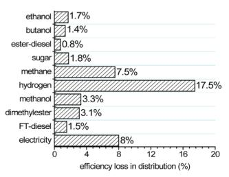
Figure 5. Comparison of transport and distribution loss efficiency for different fuels. doi:10.1371/journal.pone.0022113.g005
