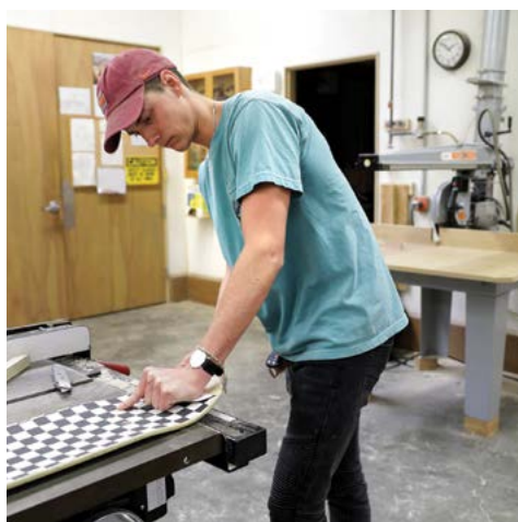
Dylan Willard sanded the decks of old skateboards to remove paint, dirt, and other stains, and cut off the protruding nose and tail.
