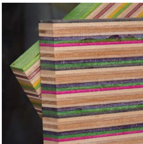
By cutting the skateboard decks into strips and turning them 90 degrees, the colored layers of plywood are exposed.
