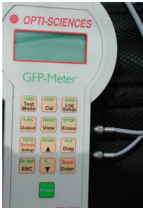
Figure 2: A potato leaf clipped into the GFP Meter (top) and the control panel where results are displayed (bottom).
