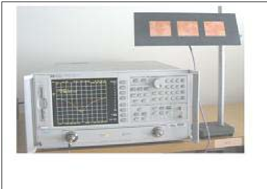
Fig 3.22:Array connected to the network analyzer
