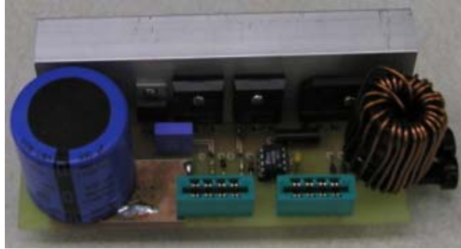
Figure 3. 26 Hardware for single-phase CCM PFC converter.
