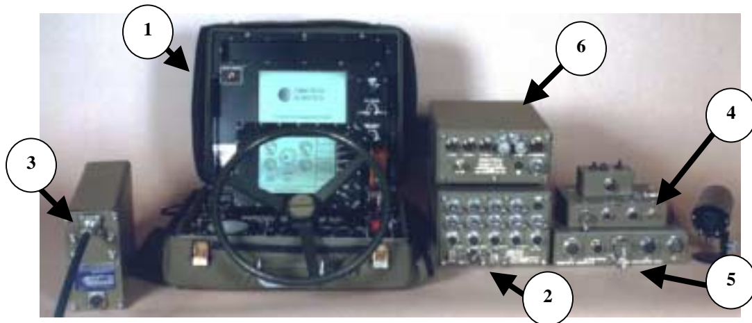
Figure 2.3: ORILLC Standard Teleoperation System (STS). (1) Operator Control Unit ; (2) Vehicle Control Unit ; (3) High Integration Actuators ; (4) Safety Radio Transmitter ; (5) System Input/Output ; (6) Video Transmitter Unit [6].
