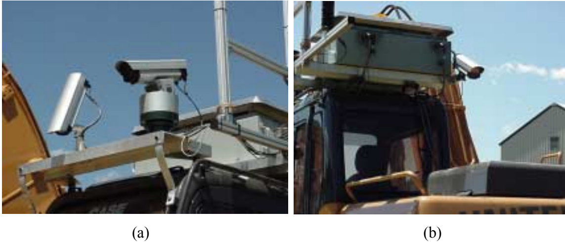
Figure 3.12: Remote cameras on teleoperated CX-160. (a) stationary and pan/tilt/zoom front camera; (b) stationary rear camera
