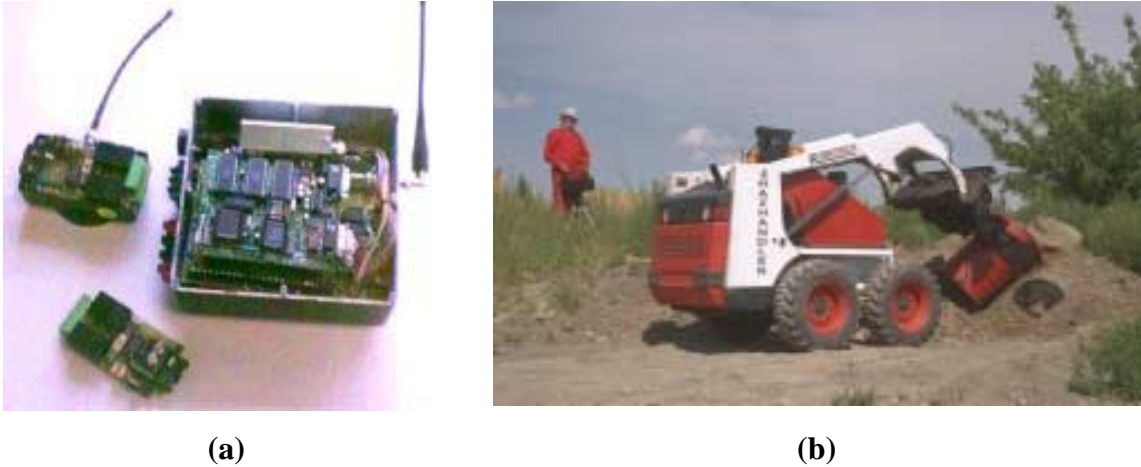
Figure 2.5: Robotec teleoperated systems. (a) Vehicle Network for Unmanned Systems (VeNUS); (b) Robotech Industries HazHandler [7].
