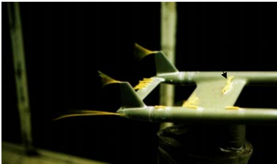
Figure 34: Small Model Tuft Test (High AOA)
