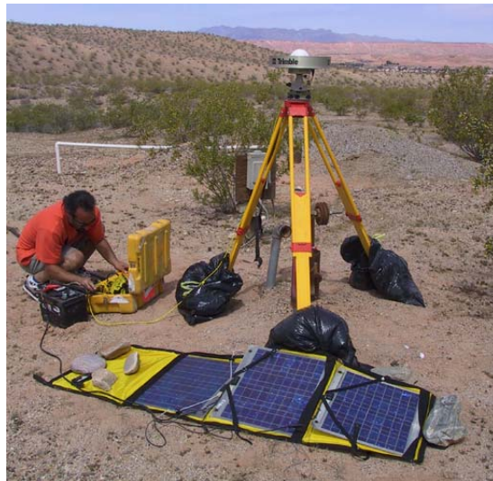
Figure 10: Antenna and receiver set up at VTex well
