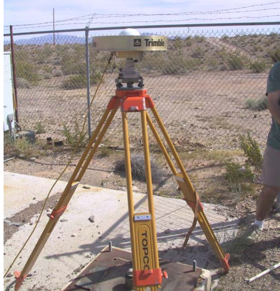
Figure 9: Tripod and antenna at well site 5 and 9 enclosed by fences
