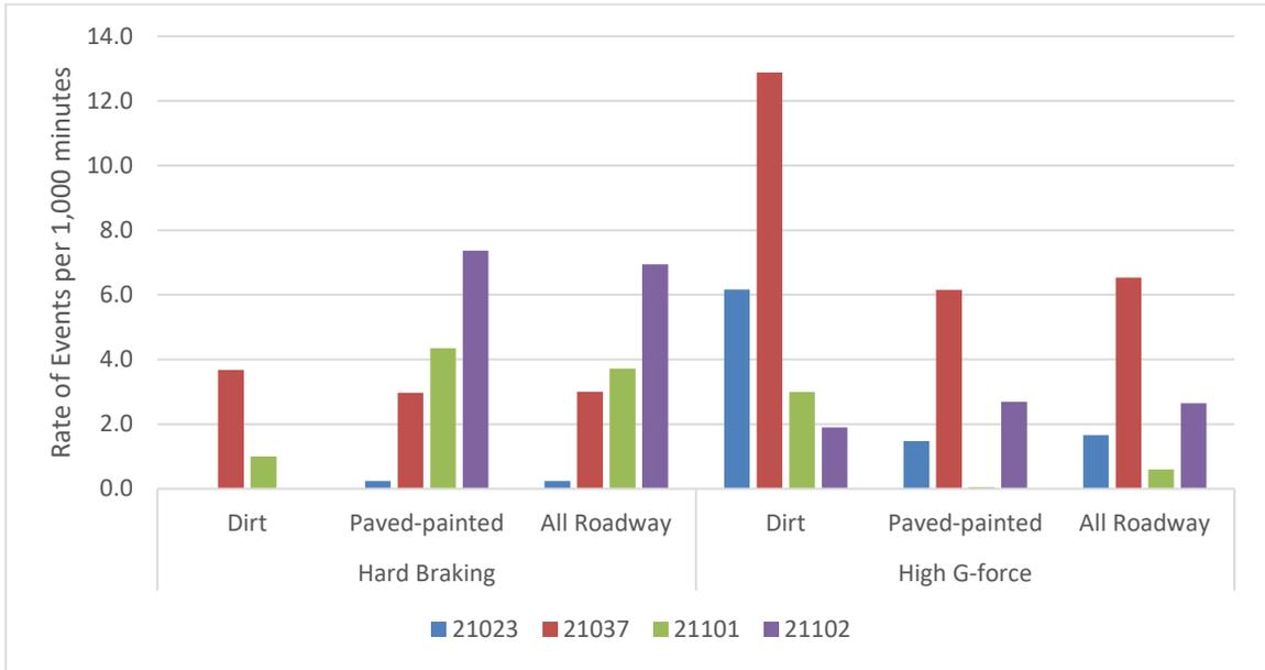
**Figure 14. Graph. Rate of hard braking maneuvers by participant ID and road type.**
