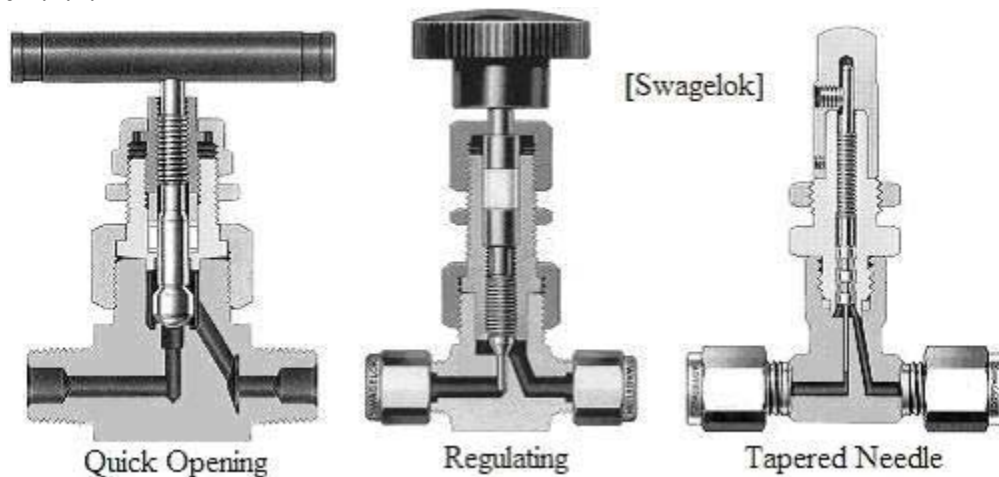
Figure 2.2.2: Diagrams for three types of Swagelok valves.
