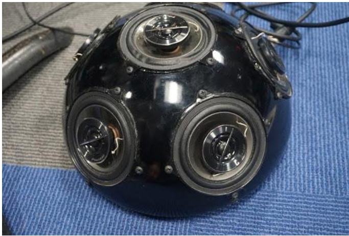
Hemispherical speaker innovatively constructed out of an IKEA salad bowl.
