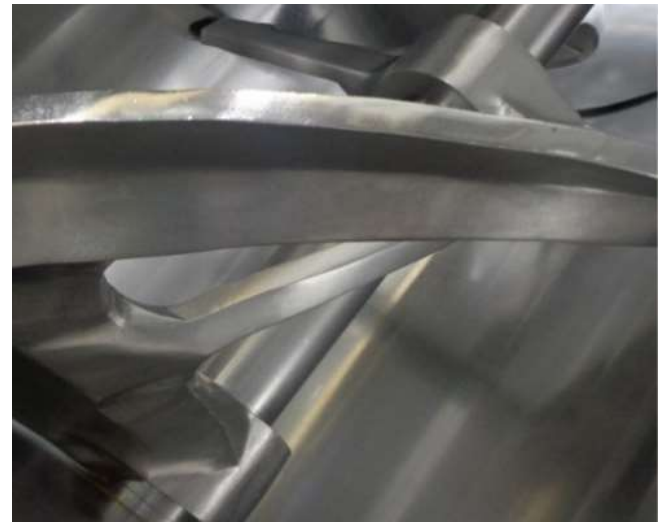
Pic.6 Mixer Blade After Cleaning
