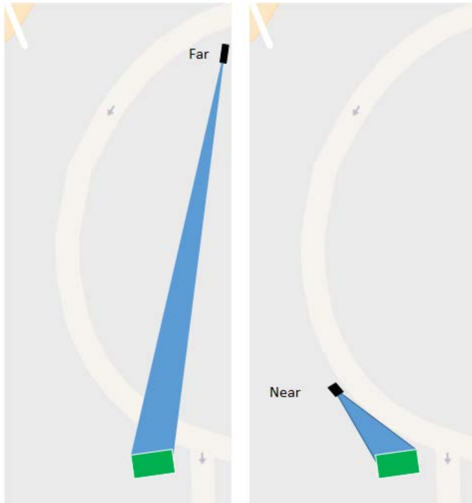
Figure 9. Illustration. Curve sign luminaire locations.
