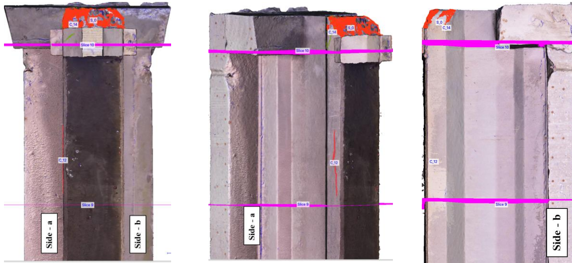
Figure B.20. Damage Clusters in the IW considered for Strength Estimation at Slice-10
