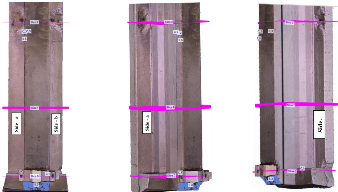
Figure B.2. Damage Clusters in the IW considered for Strength Estimation at Slice-0 and Slice-1
