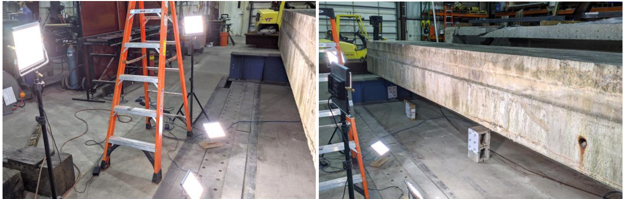
Figure 3.2. LED Lights Used to Capture Images of the Girders in an Indoor Setting
