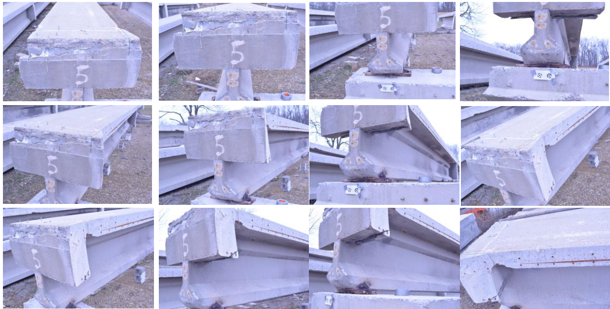
Figure 3.4. A Sequence of Images from Consecutive Locations Captured for Point Cloud Reconstruction of I-Beam 5
