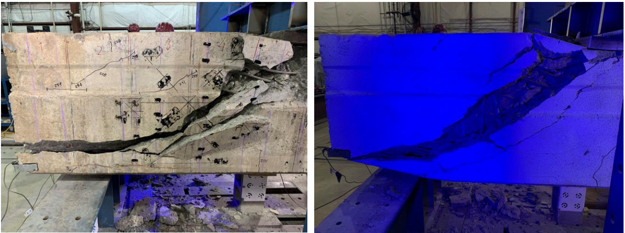
Figure 3.19. Shear Failure in Test-1 on Aden Road Bridge Box Beam-3
