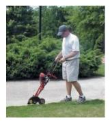
Electric Powered: The smaller electric edgers weigh approximately three pounds and they generate about 1/10-1/8 horsepower. The cutting diameter it can handle range from 7 to 12 inches. Models with 0.75 horsepower electric motors may weigh around four to eight pounds and they have the capacity to handle larger cutting lines (0 .06 inches). They are capable of cutting swaths up to 16 inches wide. These larger units come with a second adjustable assist handle to permit use of
