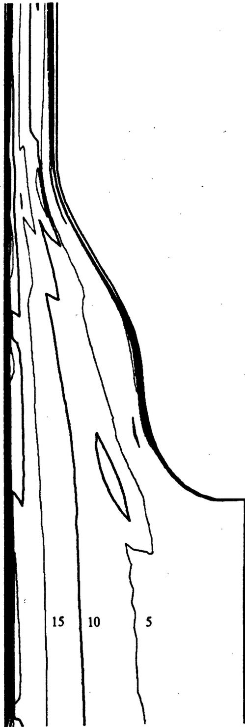
Figure 34. Meridional calculation: total pressure loss distribution,  $P_0 - P^*(Pa)$ .
