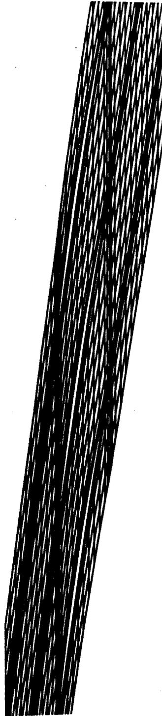
Figure 27. Blade-to-blade calculation: repeated grid with three blades and actual angles.
