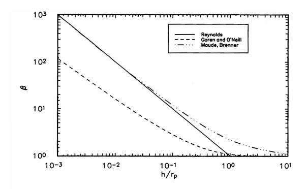
Figure 2.3 Relationship between film thinning resistance factor,  $\beta$ , and dimensionless distance, h/r<sub>p</sub> (after Luttrell, 1986).
