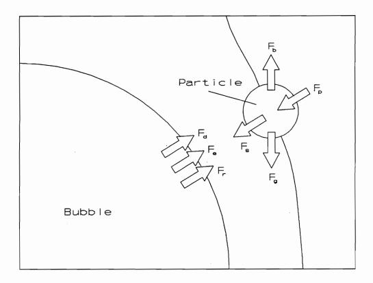
Figure 2.2 Schematic of hydrodynamic and surface forces involved in bubble-particle interaction.
