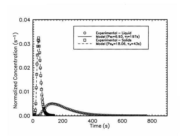
Figure 3.5 Normalized liquid and solid residence time distributions for 48 x 65 mesh silica sample.
