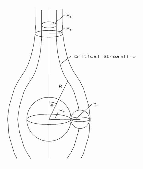
Figure 2.1 Coordinate system used to characterize bubble-particle interaction.
