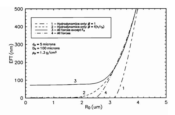
Figure 2.4 Simulation results for various force combinations.
