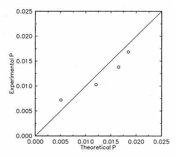
Figure 2.16 Comparison between experimental and theoretical values for the probability of particle collection.
