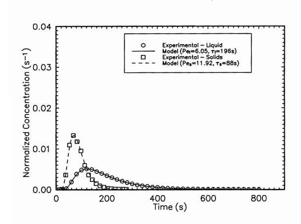
Figure 3.4 Normalized liquid and solid residence time distributions for 48 x 65 mesh coal sample.
