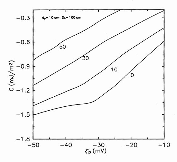
Figure 2.17 Contour plot of equilibrium film thickness showing viable regions of flotation as a function of the structural constant and the particle zeta potential.
