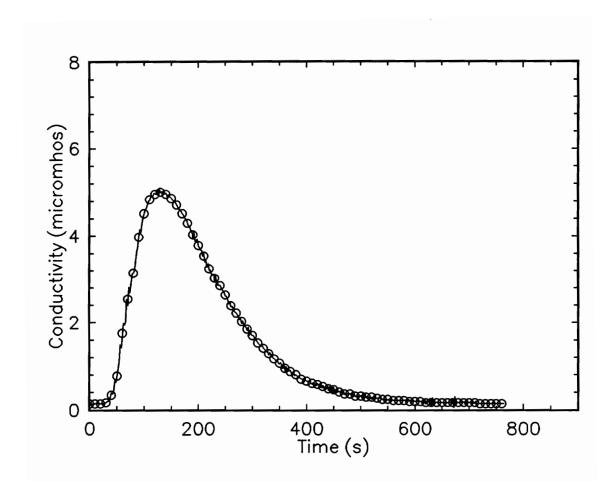
Figure 3.2 Liquid residence time distribution as constructed from time-stamped conductivity values.
