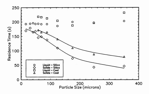
Figure 3.9 Relationship between residence time and particle size for coal and silica samples.
