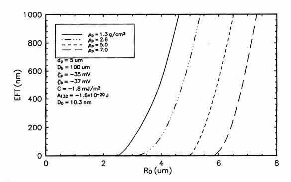
Figure 2.7 Simulation results illustrating the effect of particle density on bubble-particle interaction.
