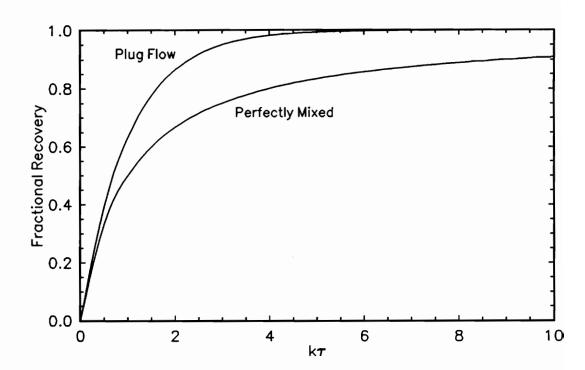
Figure 3.12 Relationship between recovery and  $k\tau$  as a function of the mixing conditions.
