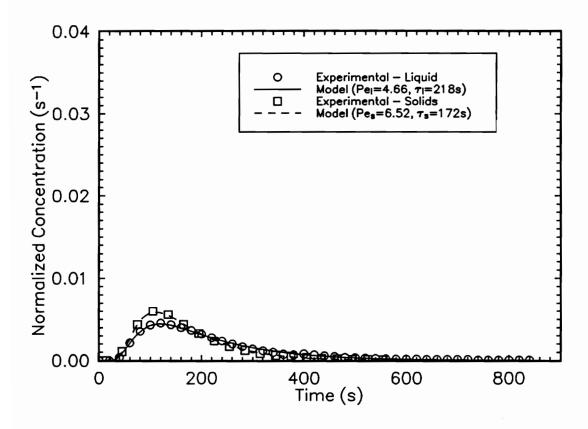
Figure 3.6 Normalized liquid and solid residence time distributions for 250 x 270 mesh coal sample.
