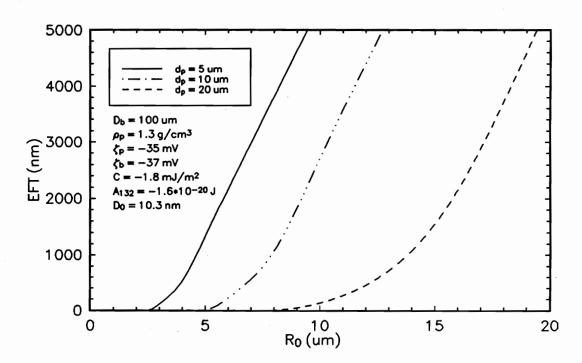
Figure 2.5 Simulation results illustrating the effect of particle size on bubble-particle interaction.
