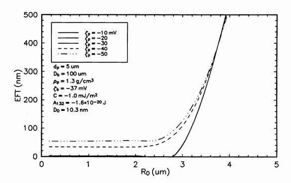
Figure 2.9 Simulation results illustrating the effect of particle charge on bubble-particle interaction for  $C = -1.0 \text{ mJ/m}^2$ .
