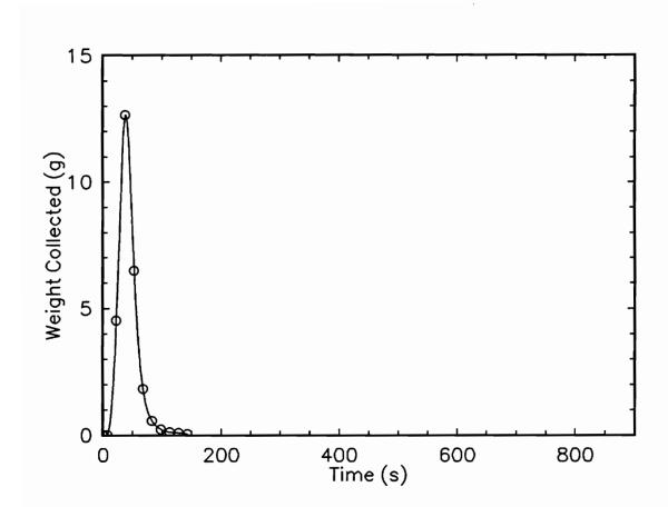
Figure 3.3 Solids residence time distribution for 48 x 65 mesh silica size fraction from tailings discharge sample collection weights.
