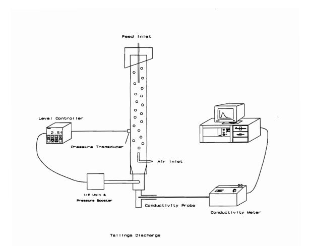
Figure 3.1 Schematic of experimental apparatus used for determining solid and liquid residence time distributions in a flotation column.
