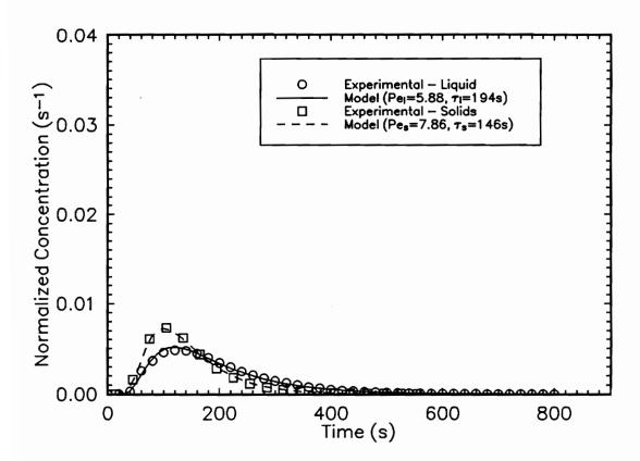
Figure 3.7 Normalized liquid and solid residence time distributions for 250 x 270 mesh silica sample.
