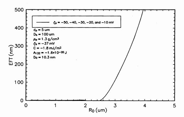
Figure 2.8 Simulation results illustrating the effect of particle charge on bubble-particle interaction for  $C = -1.8 \text{ mJ/m}^2$ .
