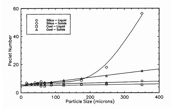
Figure 3.8 Relationship between Peclet number and particle size for coal and silica samples.
