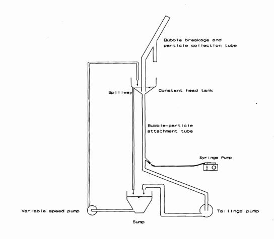
Figure 2.11 Schematic of apparatus used for bubble-particle attachment experiments.
