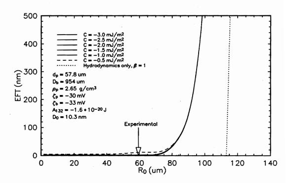
Figure 2.14 Simulation results for 250 x 270 mesh silica sample used in bubble-particle attachment experiments.
