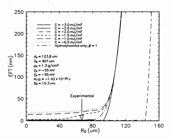
Figure 2.12 Simulation results for 100 x 150 mesh coal sample used in experiments.
