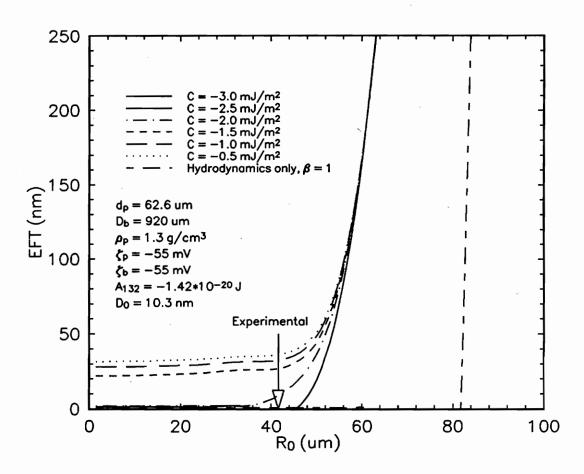
Figure 2.13 Simulation results for 200 x 270 mesh coal sample used in experiments.
