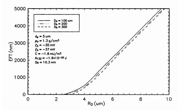
Figure 2.6 Simulation results illustrating the effect of bubble size on bubble-particle interaction.
