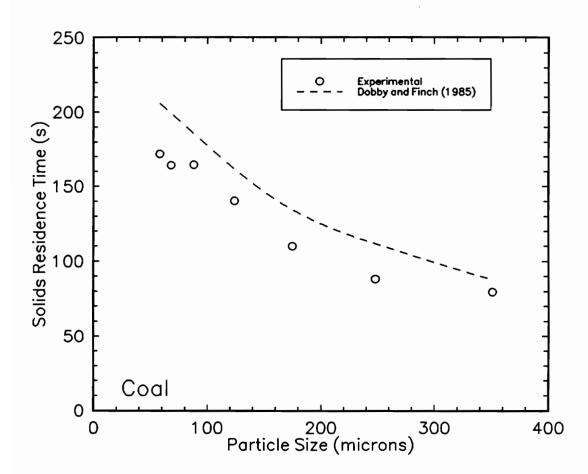
Figure 3.11 Comparison between experimental and theoretical solids residence time for coal.
