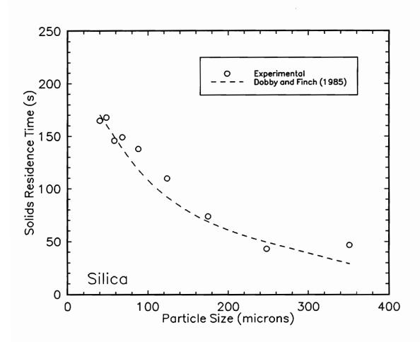
Figure 3.10 Comparison between experimental and theoretical solids residence time for silica.
