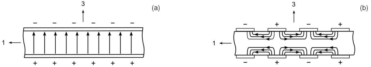
Figure A.3: The figures show the electric fields in: (a) a conventional piezoceramic wafer; (b) an MFC actuator [adapted from Bevan (2000)].
