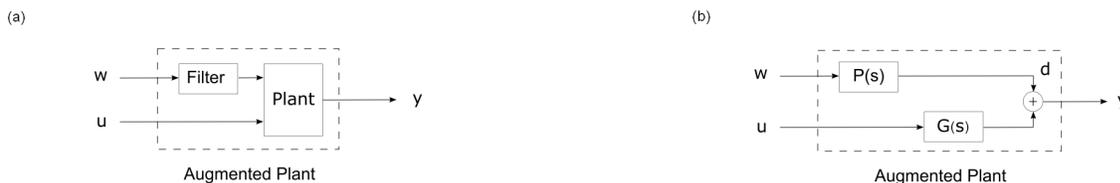
Figure 3.5: Diagram of an augmented plant model used to shape the disturbance path. The figures show: (a) a general block diagram; and (b) a diagram expressed in terms of the disturbance model and control path.
