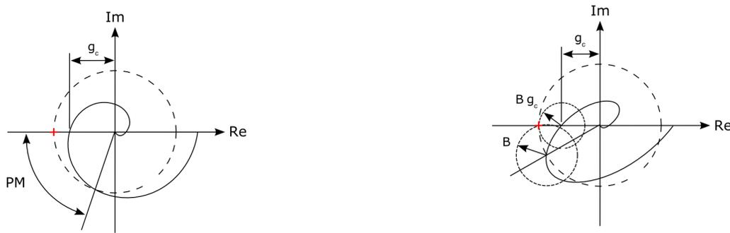
Figure B.2: The figures show: (a) a simple Nyquist diagram illustrating the concepts of gain and phase margins; and (b) an example demonstrating the relationship between multiplicative uncertainty and the required stability margins.
