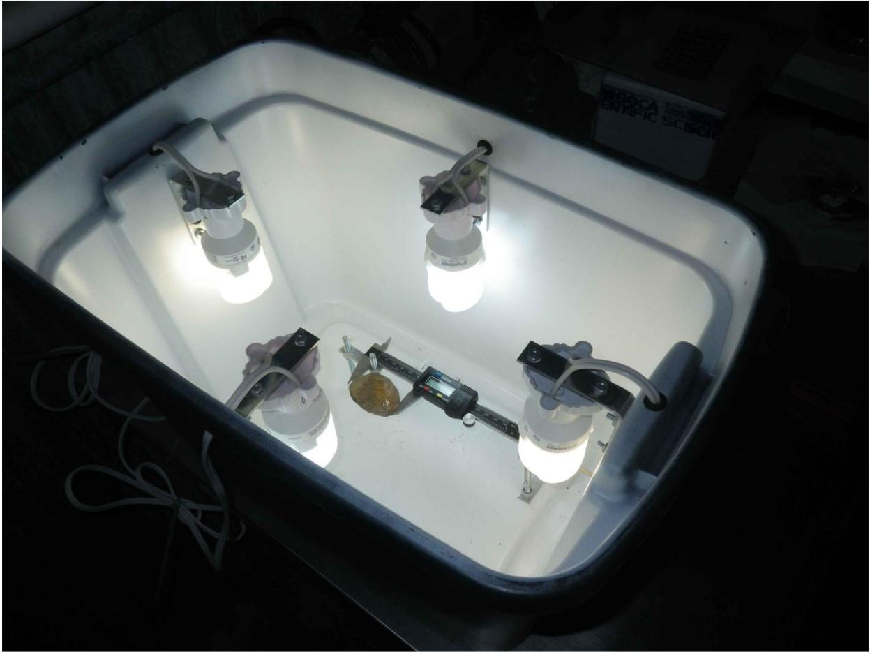
Figure 3. Light-box used to hold specimens while photographs were taken; lid not shown.
