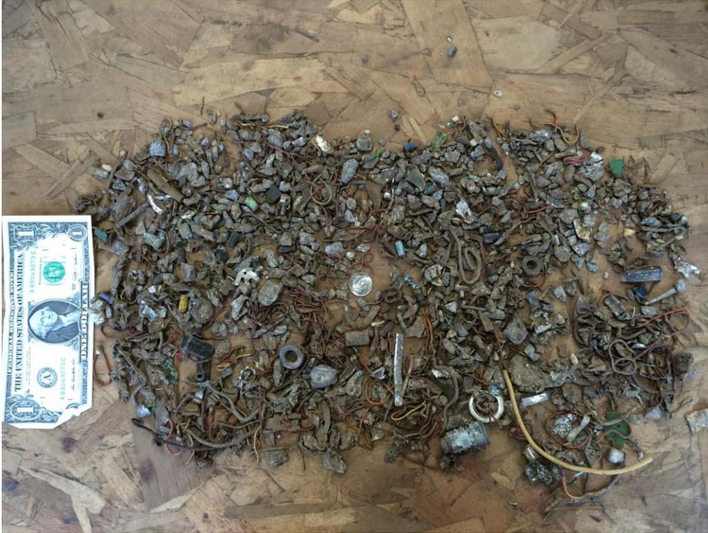
**Fig. 1.2: Zorba from an eddy current separator. Currency shown for scale.**
