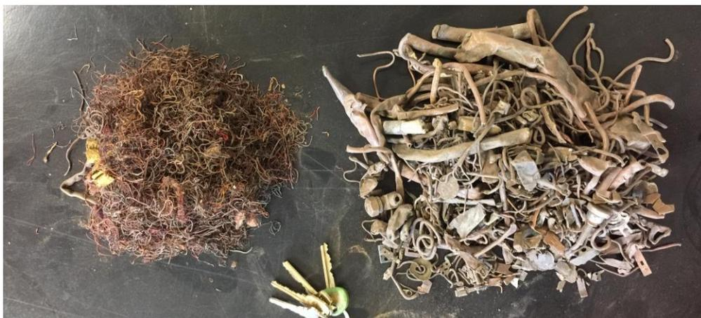
**Fig. 3.5: Copper found in the concentrate (right), and copper found in the tailings (left)**
