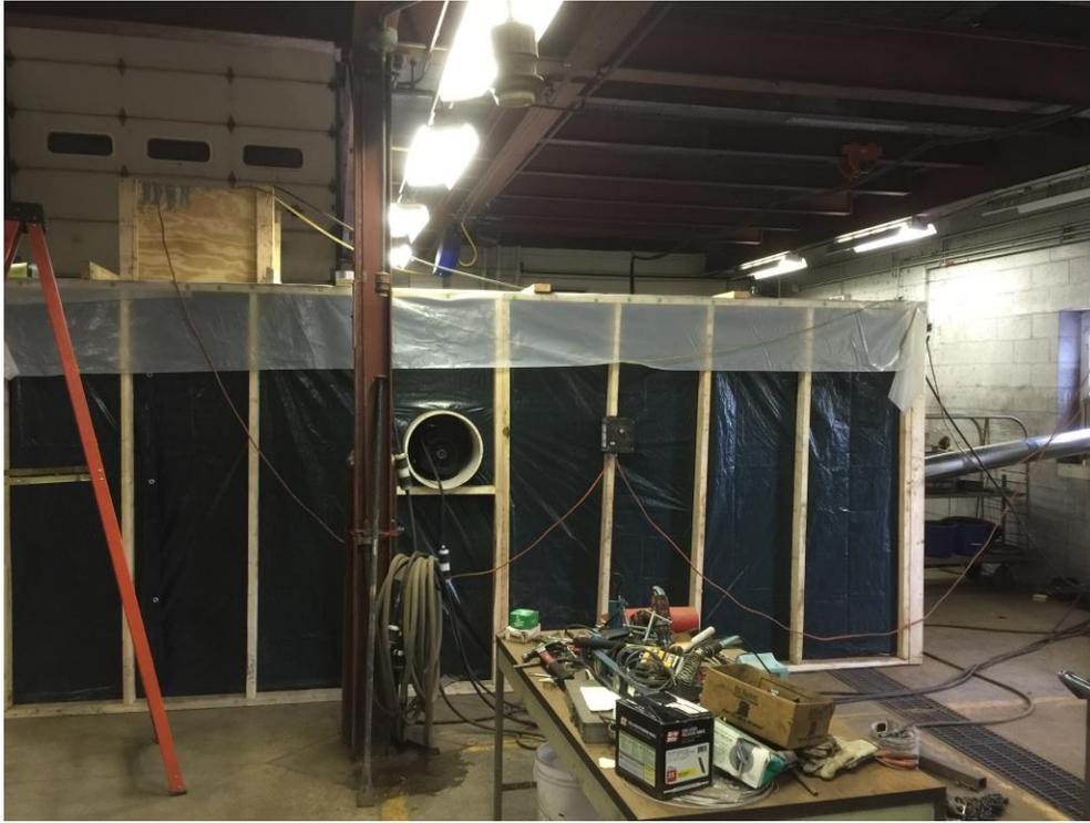
**Fig. 3.4: Showing the enclosure for the eddy current separator.**
