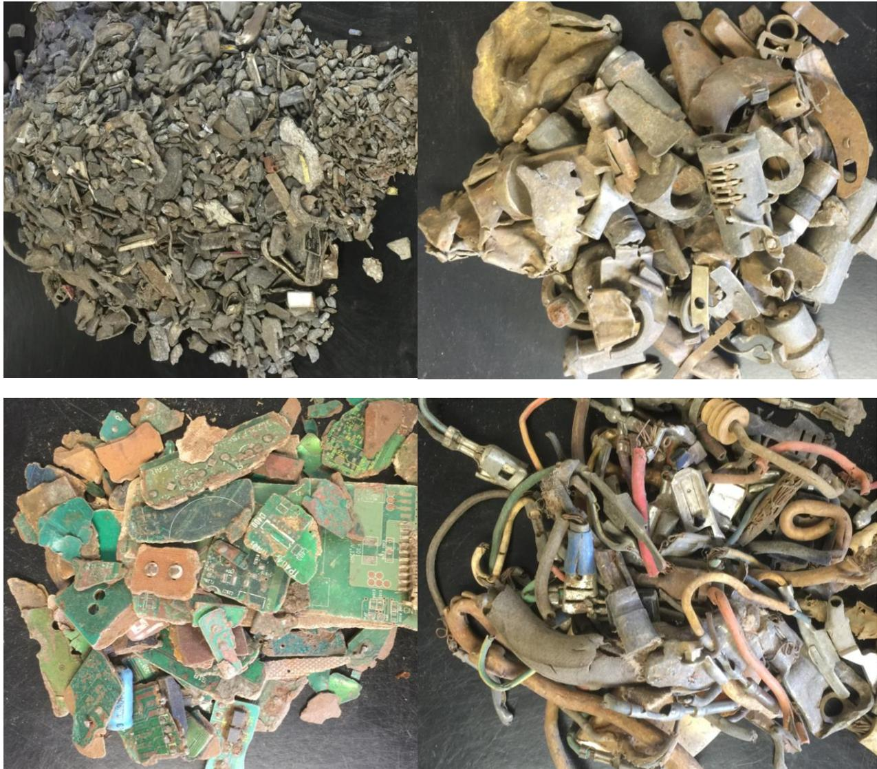
**Fig. 3.6: Constituents of the feed tested including aluminum (top left), brass (top right), ICW (bottom right), and circuit board (bottom left).**
