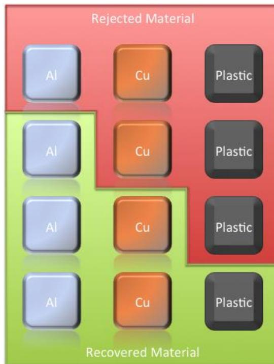
Fig 1.9: Feed sample showing split by eddy current separator.
