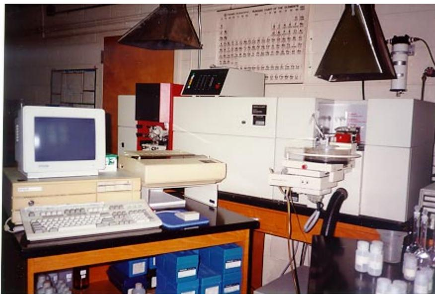
Figure A1. Perkin-Elmer Atomic Absorbtion Spectrophotometer
