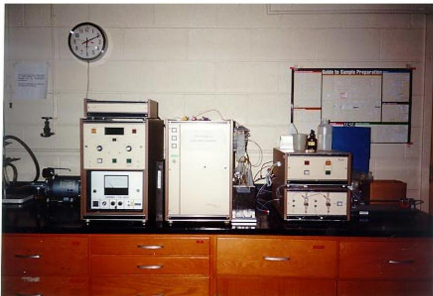
Figure A2. Dohrmann Carbon Analyzer Used for TOC Analysis
