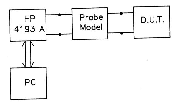
Figure (3.17). RF measurement setup.
