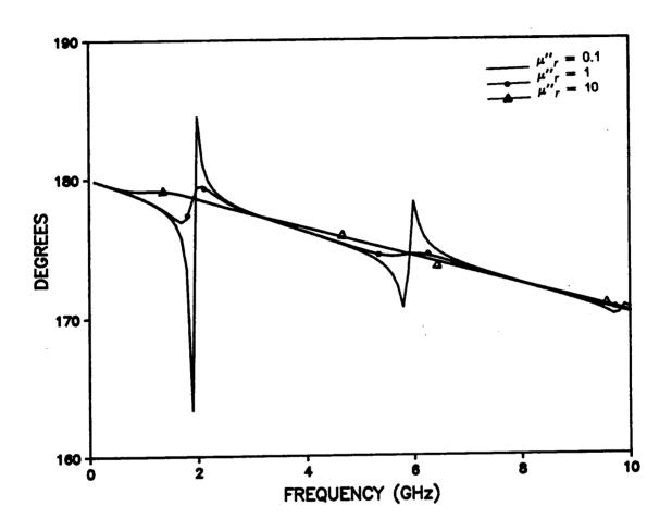
Figure (4.6). Effect of varying the magnetic loss,  ${\mu^{\prime\prime}}_r$ , on the phase of  $S_{11}$
