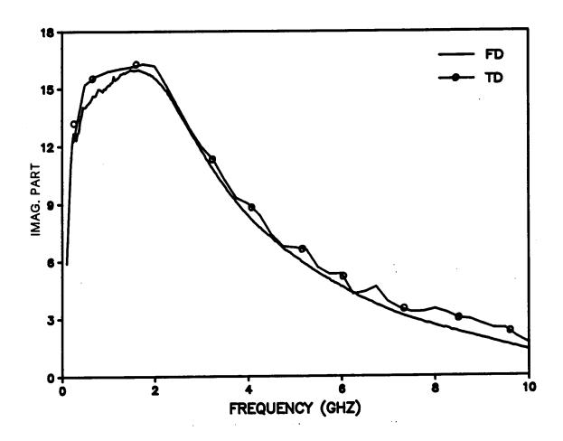
Figure (4.19). Relative magnetic loss,  $\mu''_{r}$ , of the Remex 4920 thick film ferrite paste.
