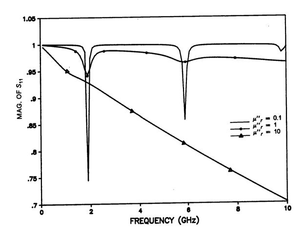
Figure (4.5). Effect of varying the magnetic loss,  $\mu^{\prime\prime}_{r}$ , on the magnitude of  $S_{11}$
