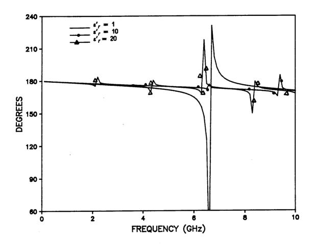
Figure (4.3). Phase of  $S_{11}$  corresponding to different values of real part of permittivity  $\epsilon'_{r}$ .
