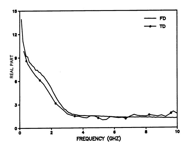
Figure (4.14). Real part of relative permeability,  $\mu'$ ,, of the ESL EX-2000 thick film ferrite paste.
