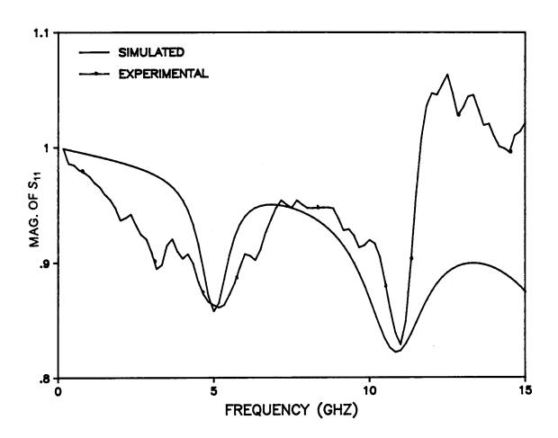
Figure (4.21). Simulated and experimental magnitude of  $S_{11}$  of the 2 cm cavities.
