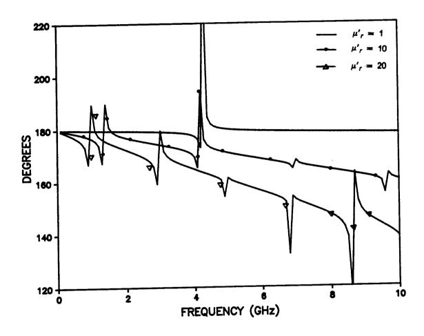
Figure (4.4). Phase of  $S_{11}$  corresponding to different values of real part of permeability  $\mu'_{f}$ .
