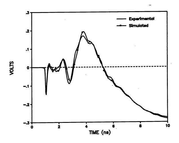
Figure (3.14). Experimental and simulated response waveforms for the multilayer inductor with dielectric material.
