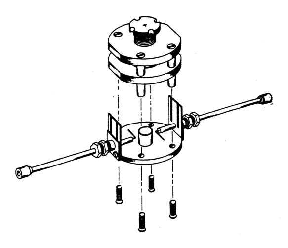
Figure (2.4). Exploded view of the ferrite post resonator showing the sample and the probes in position.
