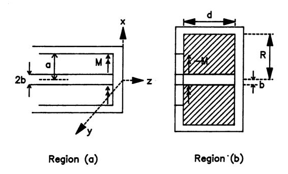
Figure (4.2). Model for the cavity structure after applying the equivalence principle.
