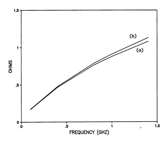
Figure (4.23). Imaginary part of impedances from (a) measured  $S_{11}$  and (b) measured  $\mu_r^{\Lambda}$ .
