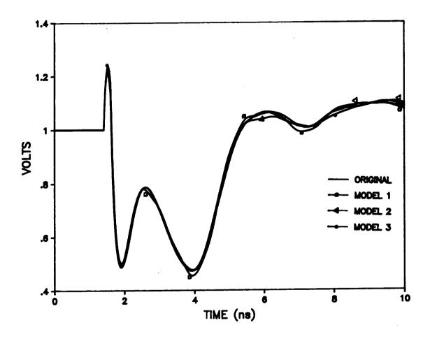
Figure (3.23). Comparison between the original response waveform and the models response waveform. 0.39 ns ramp excitation.
