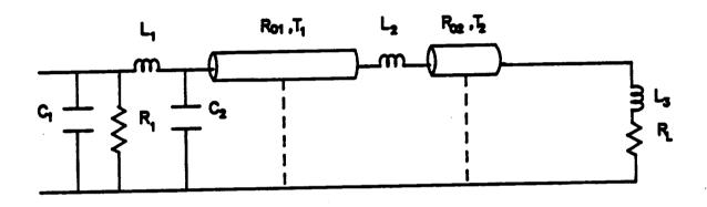
Figure (3.13). Electrical model for the multilayer inductor with dielectric material.
