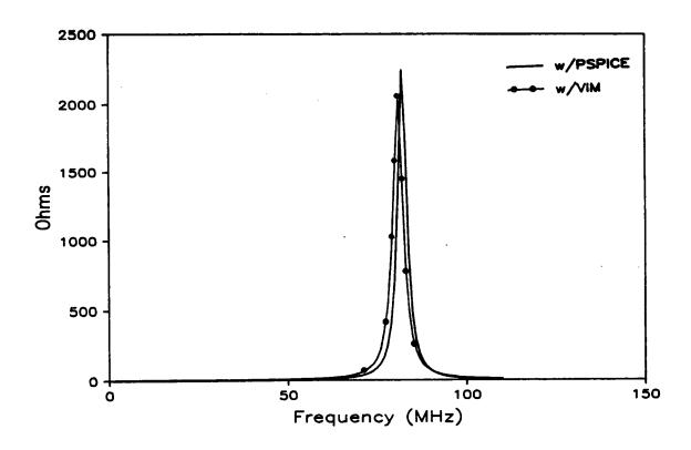
Figure (3.18). Comparison between the real component of impedance calculated from PSPICE and the one measured on the VIM.
