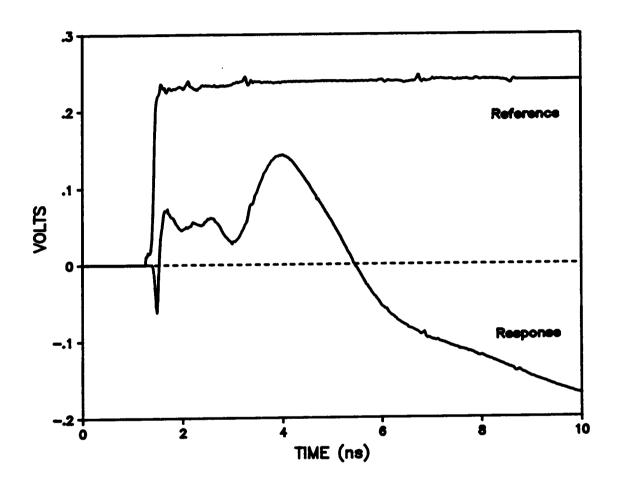
Figure (3.5). Reference and response waveforms for a multilayer inductor separated by ferrite material.
