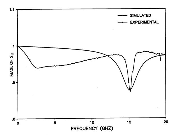
Figure (4.20). Simulated and experimental magnitude of  $S_{11}$  of the 1 cm cavities.
