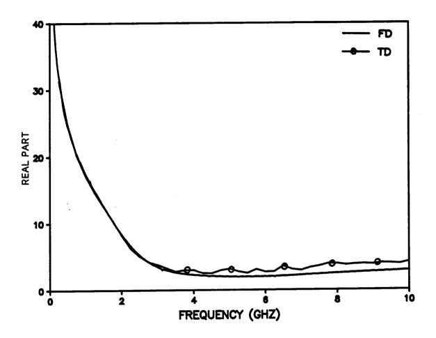
Figure (4.18). Real part of relative permeability,  $\mu'$ , of the Remex 4920 thick film ferrite paste.
