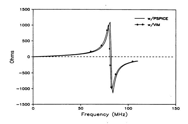
Figure (3.19). Comparison between the imaginary component of impedance calculated from PSPICE and the one measured on the VIM.
