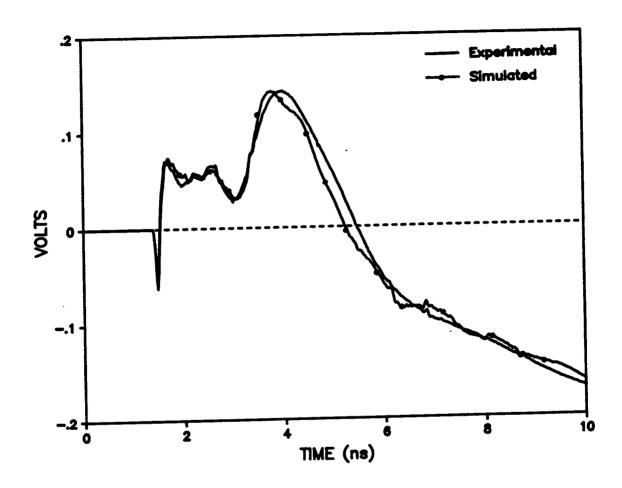
Figure (3.16). Experimental and simulated response waveforms for the multilayer inductor with ferrite material.
