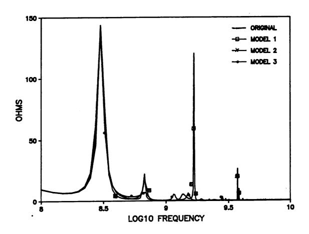
Figure (3.27). Comparison between the impedance real component of the original circuit with the impedance real components of the models.
