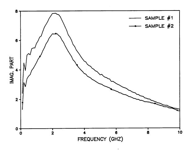
Figure (4.17). Relative magnetic loss,  $\mu''$ , of two different samples where ESL EX-2000 ferrite paste was used.
