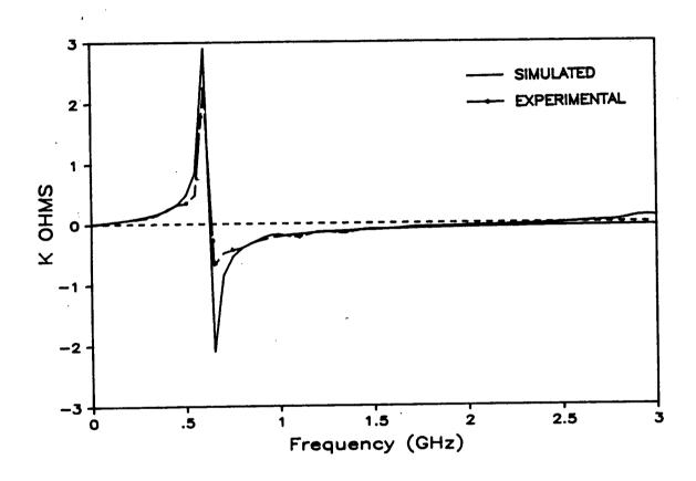
Figure (3.12). Comparison between the impedance imaginary components of the single layer coil and it's model.
