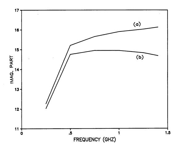
Figure (4.26). Relative magnetic loss  $\mu''_r$ , (a) measured  $\mu''_r$  and (b) verified  $\mu''_r$ .
