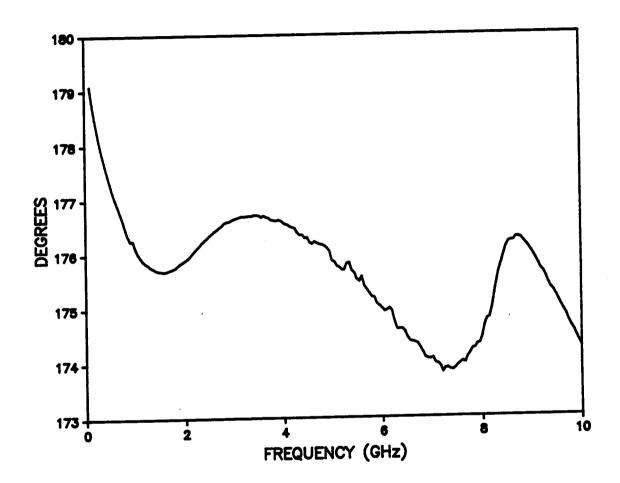
Figure (4.12). Phase of  $S_{11}(j\omega)$ .
