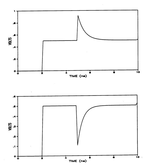
Figure (3.6). Reflected waveform from (a) inductive discontinuity (b) capacitive discontinuity.
