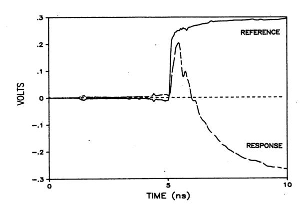
Figure (3.7). Reference and response waveforms for a single layer coil.
