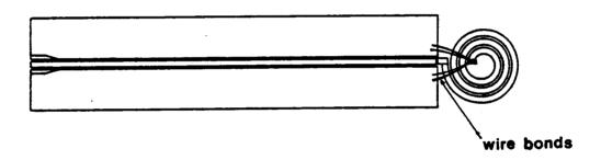
Figure (3.2). Top view of multilayer inductor.
