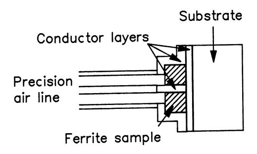
Figure (4.1). The coaxial cavity structure.
