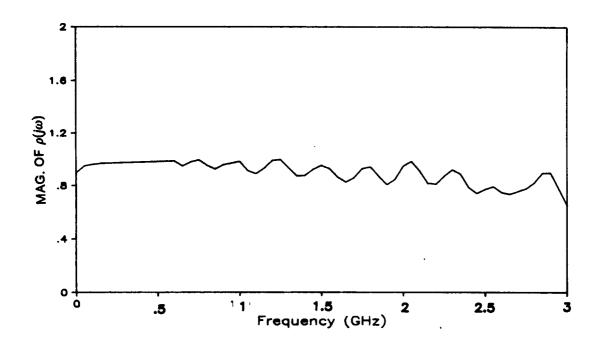
Figure (3.8). Magnitude of  $\rho(J\omega)$  from the response waveform shown in Figure (3.7).
