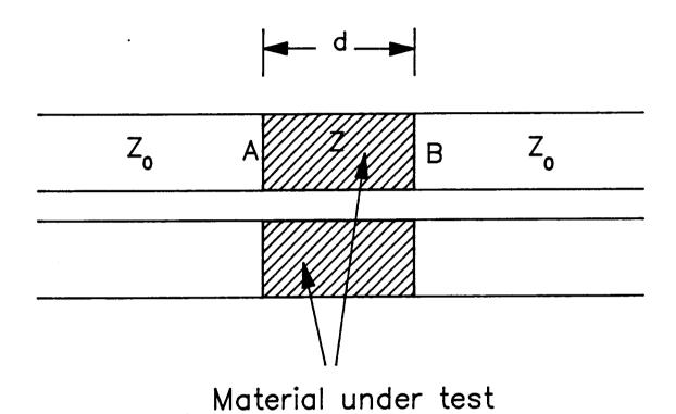
Figure (2.3). A coaxial line with annular disk of material to be measured inserted.
