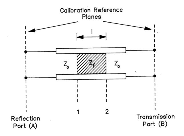
Figure (2.1). Transmission line section containing ferrite material.
