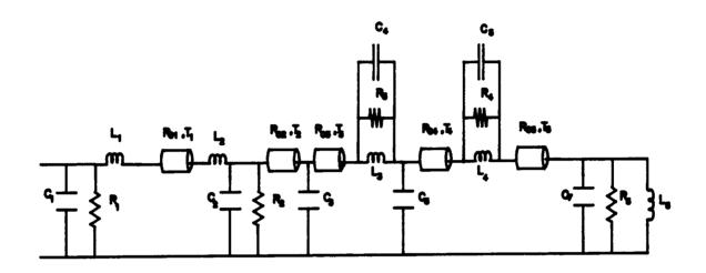
Figure (3.15). Electrical model for the multilayer inductor with ferrite material.
