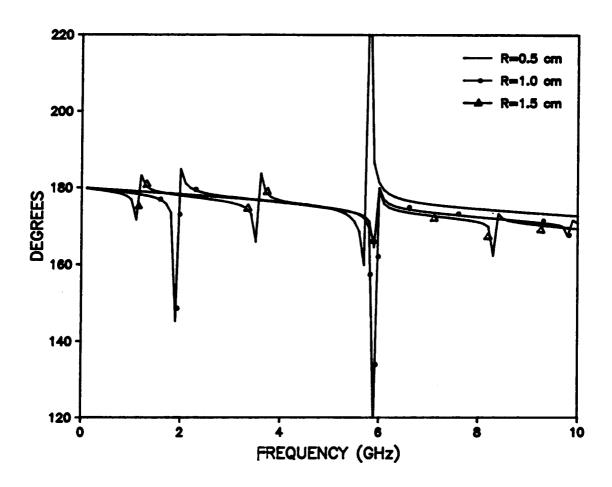
Figure (4.7). Effect of varying the outer radius of the cavity on the phase of  $S_{11}$
