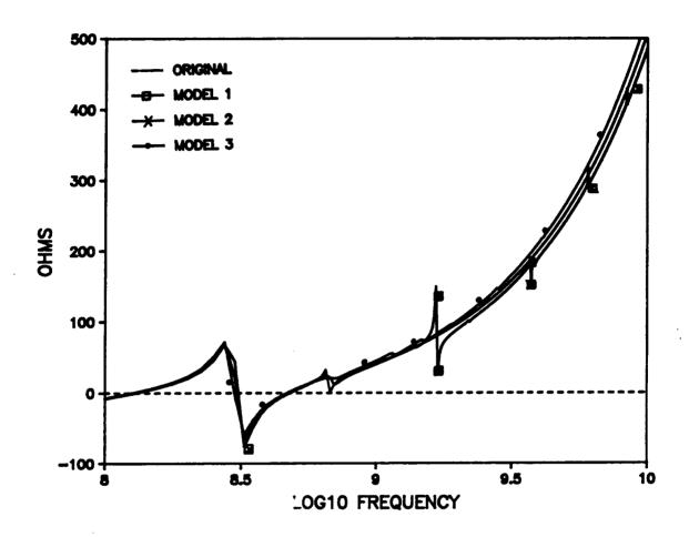
Figure (3.28). Comparison between the impedance imaginary component of the original circuit with the impedance imaginary components of the models.
