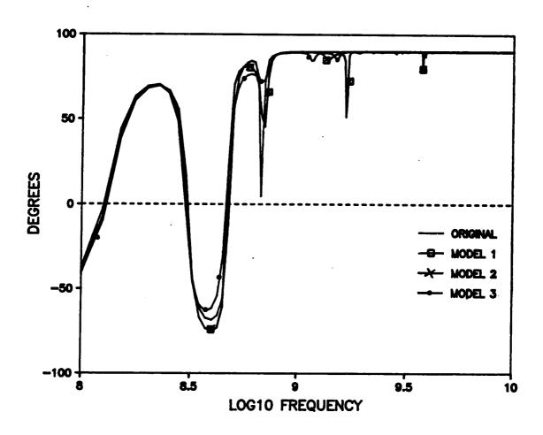
Figure (3.30). Comparison between the phase of the impedance of the original circuit with the phase of the impedances of the models.
