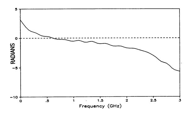
Figure (3.9). Phase of  $\rho(j\omega)$  from the response waveform shown in Figure (3.7).
