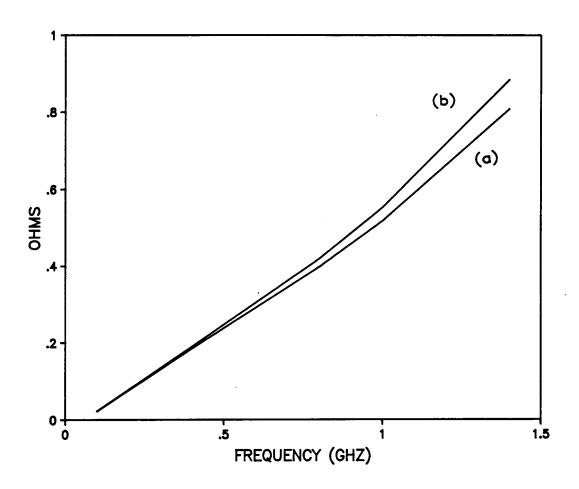
Figure (4.22). Real part of impedances from (a) measured  $S_{11}$  and (b) measured  $\mu_r^*$ .
