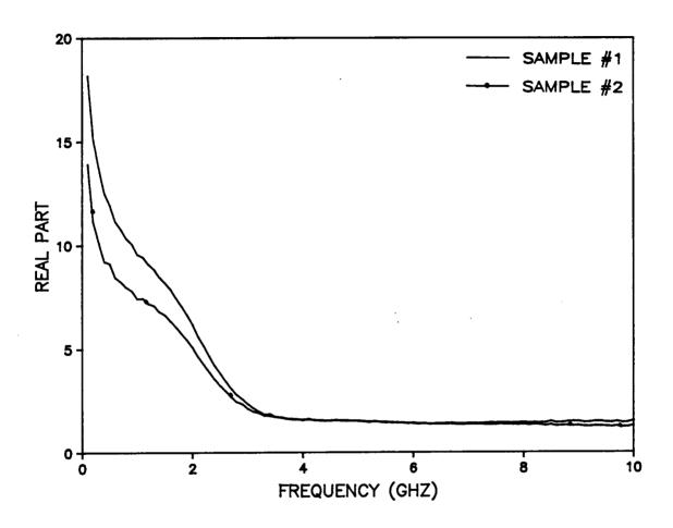
Figure (4.16). Real part of relative permeability,  $\mu'_r$ , of two different samples where ESL EX-2000 ferrite paste was used.
