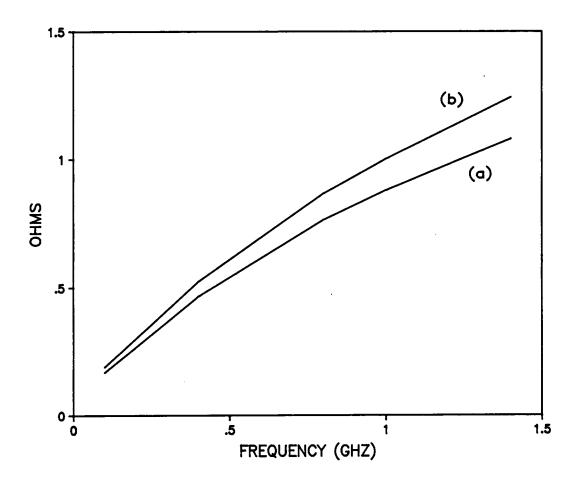
Figure (4.24). Sensitivity of the second computed impedance to change in  $\mu'_r$ , (a) measured  $\mu'_r$ , and (b) 1.1 measured  $\mu'_r$ .
