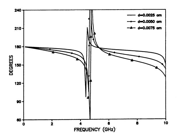
Figure (4.8). Effect of varying the sample thickness on the phase of  $S_{11}$
