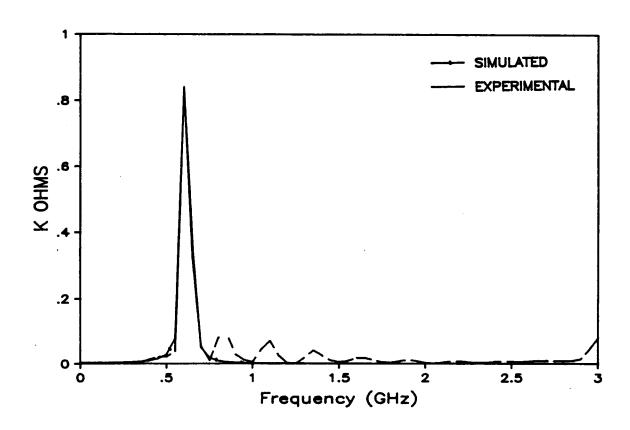
Figure (3.11). Comparison between the impedance real components of the single layer coil and it's model.
