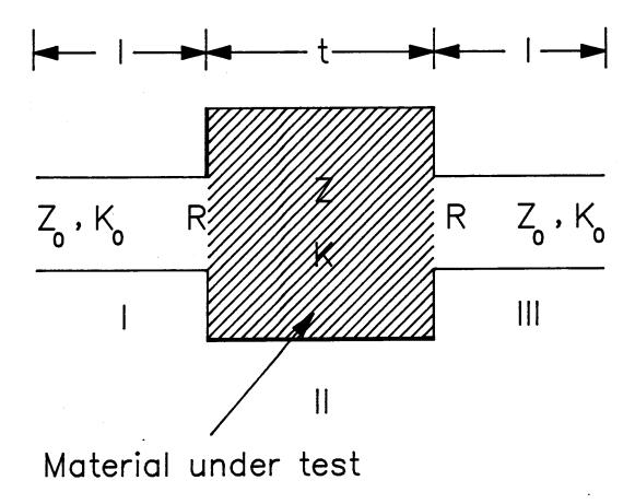
Figure (2.2). Strip transmission line loaded with the material under test.
