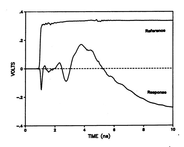
Figure (3.4). Reference and response waveforms for a multilayer inductor separated by dielectric material.
