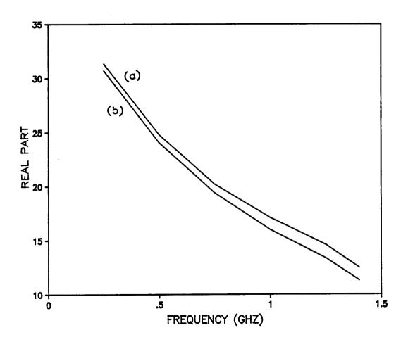
Figure (4.25). Real part of relative permeability  $\mu'_{r}$ , (a) measured  $\mu'_{r}$ , and (b) verified  $\mu'_{r}$ .
