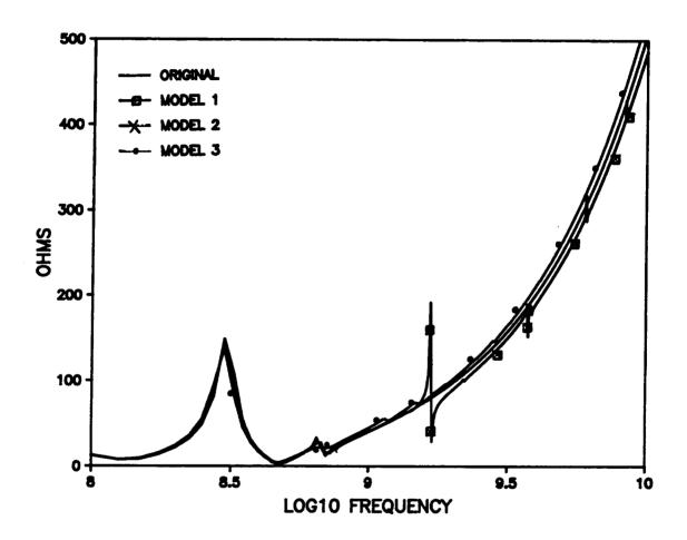
Figure (3.29). Comparison between the magnitude of the Impedance of the original circuit with the magnitude of the impedances of the models.
