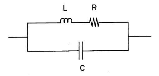
Figure (3.10). Single layer coil electrical model.
