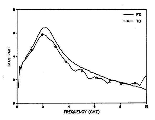
Figure (4.15). Relative magnetic loss,  $\mu''_{, i}$ , of the ESL EX-2000 thick film ferrite paste.
