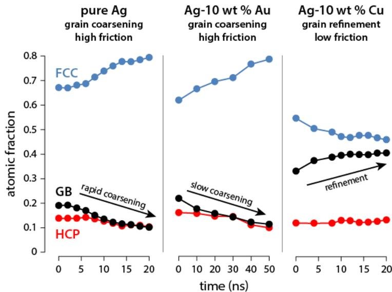
**Fig. 8.** Evolution in grain boundary density for slabs of (left) pure, (middle) soluble alloy and (right) insoluble alloy after sliding at 300 MPa normal stress. Grain growth and high friction was found to occur in the pure and soluble alloy contacts where sliding occurs along FCC slip planes, but the immiscible alloy contact exhibited grain refinement (GB stability) and deformation was primarily accommodated via GB sliding with concomitant low friction.
