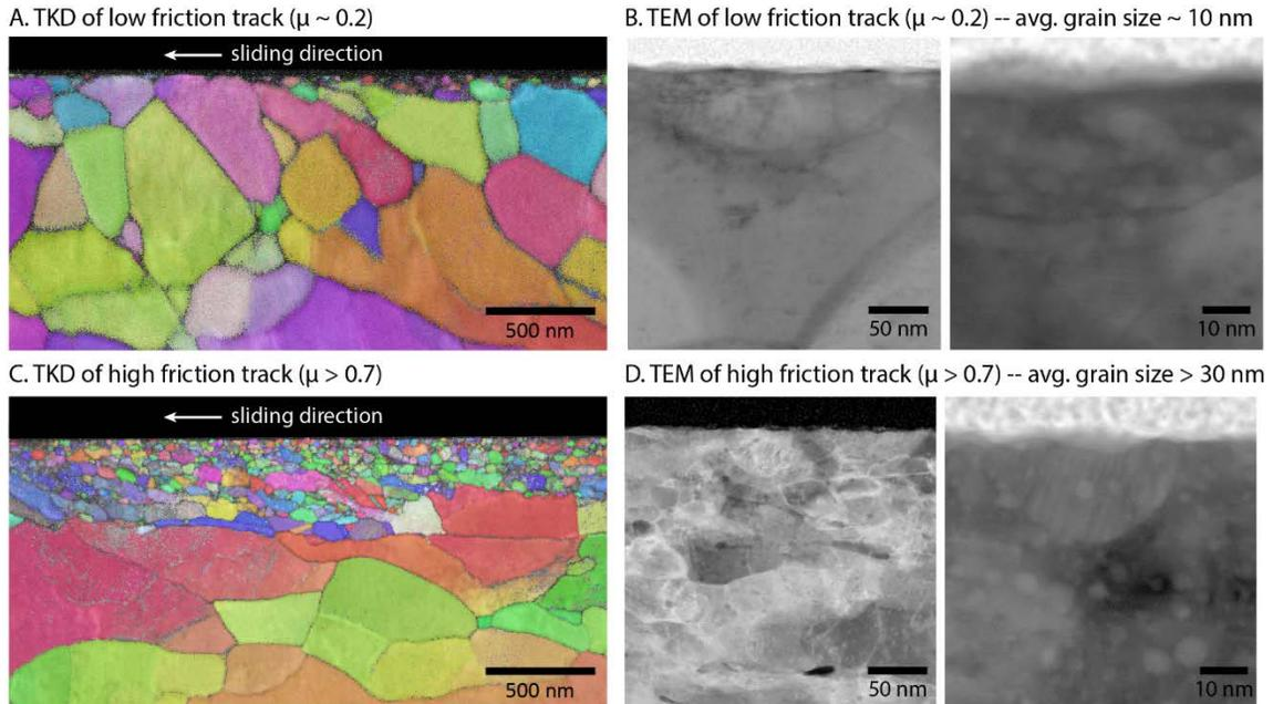
**Fig. 5.** (A and C) Grain orientation maps via TKD in SEM; color defines grain orientation. Low and high friction wear tracks correspond to experiments for which friction data is shown in Fig. 2, upon completion
