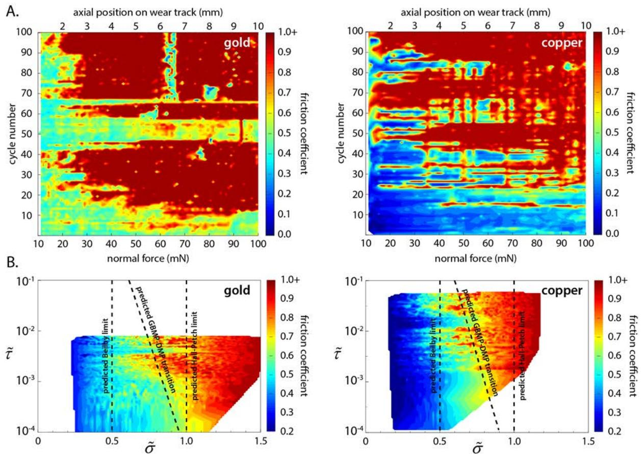
**Fig. 11.** (A) Ramped normal force friction coefficient data for self-mated copper and gold contacts and (B) the same data processed into phase space maps of friction behavior for Au and Cu sliding contacts with calculated predictions of regime bounds overlaid using dotted lines.
