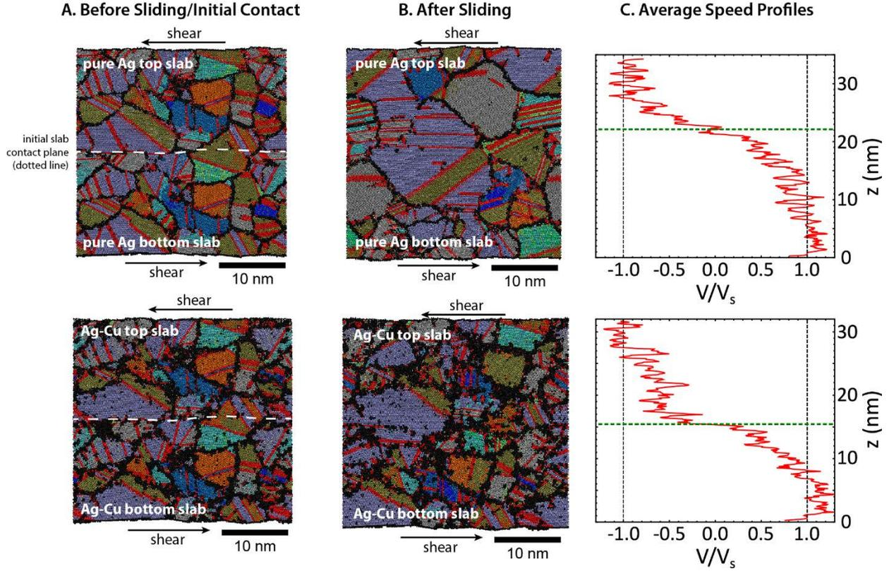
**Fig. 6.** Snapshots of sliding contact simulations between two pure Ag and two Ag-Cu slabs at (A) initial contact before sliding and (B) after sliding. White dashed lines in (A) approximately indicate the location of the initial interface between the two slabs. In (C) we show the average velocity through the thickness in the sliding direction; the red lines are the velocities in the sliding direction.
