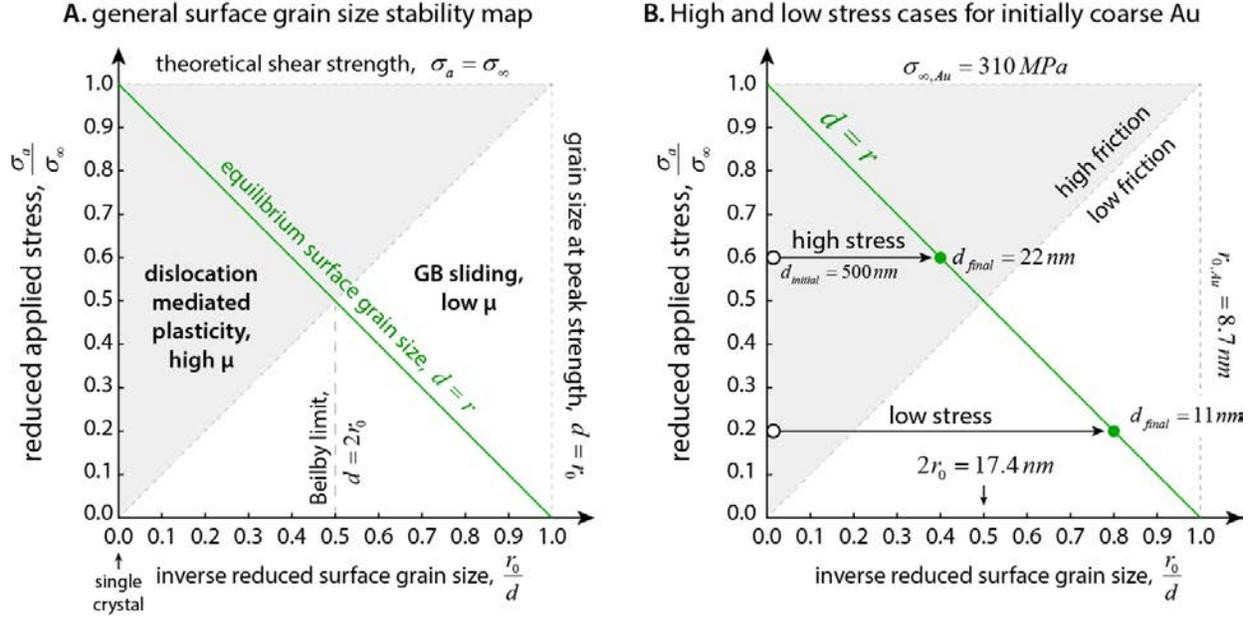
**Fig. 9. (A)** Friction regimes and dominant plasticity mechanisms map as a function of reduced stress and grain size, adapted and evolved from Yamakov et al. [66]. **(B)** Friction regimes and dominant plasticity mechanisms map showing two possible cases of time-dependent evolution of an Au-Au contact at low ( $\sigma/\sigma_\infty = 0.2$ ) and high ( $\sigma/\sigma_\infty = 0.6$ ) reduced stresses with an initial grain size of 500 nm.
