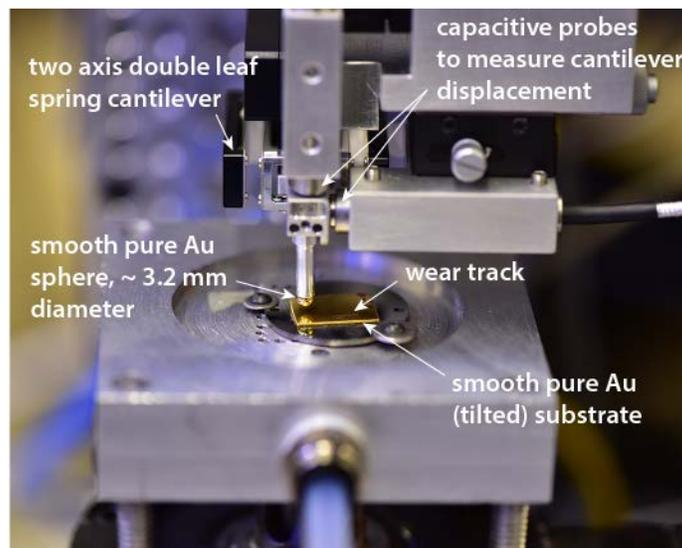
**Fig. 2.** Annotated photograph of tribometer showing a sliding experiment between a smooth pure Au ball and a pure Au substrate.
