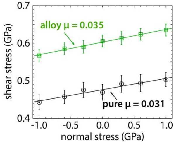
**Fig. 7.** Friction vs. normal stresses for (A) the self-mated elastic slab-slab contacts of pure Ag (circles) and Ag-Cu alloy (squares) and (B) for rigid plate sliding over an elastic slab cases of pure Ag (circles) and Ag-Cu alloy (squares).
