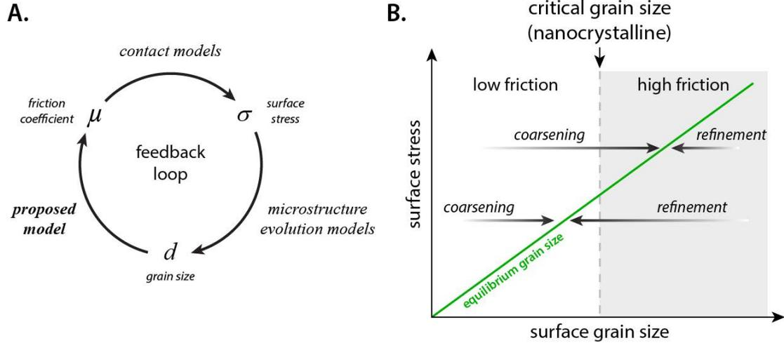
**Fig. 1.** (A) A diagram illustrating the feedback loop between maximum surface stress,  $\sigma$ , surface grain size,  $d$ , and friction coefficient,  $\mu$ , and (B) the concept that there is a stress-dependent equilibrium grain size toward which surface grain size evolves, and a critical grain size differentiating between low and high friction behavior.
