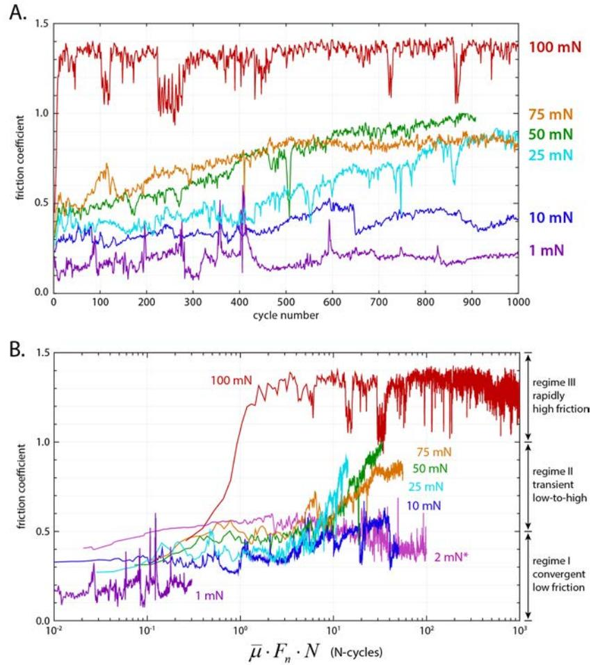
**Fig. 3.** Friction evolution data for a hard Au spherically tipped pin sliding against a flat pure Au coupon in dry nitrogen at constant normal forces as a function of (A) cycles and (B) the product of average friction coefficient for each experiment, normal force and cycles, analogous to accumulated plastic strain due to shear; the 2 mN data corresponds to a longer, 100k cycle experiment that was performed using uni-directional sliding in a rotating pin-on-disk tribometer.
