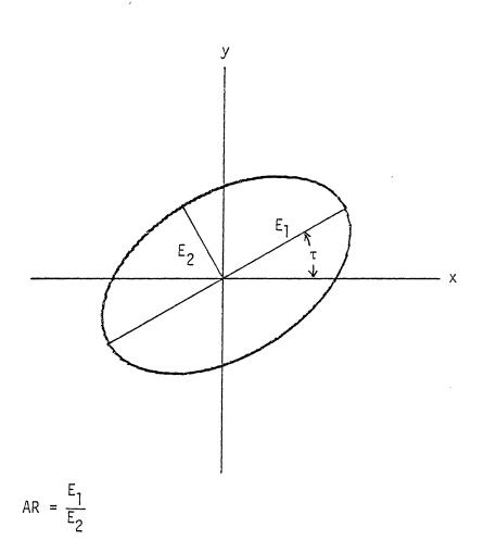
Figure 4.2-1. Polarization ellipse.
