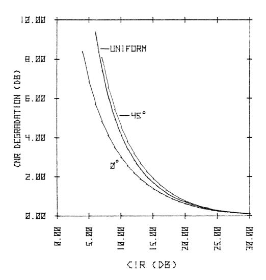
Figure 2.3-1. QPSK CNR Degradation with QPSK interference for 0, and 45° relative phase shift and for uniformly distributed phase shift.
