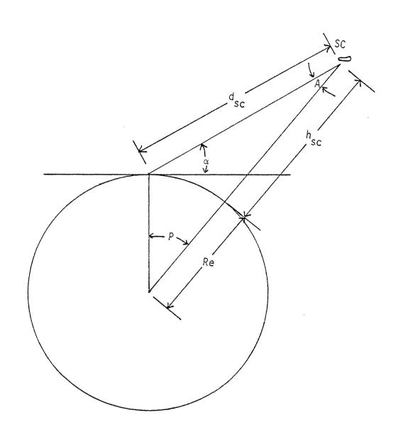
Figure A-1. Satellite orbit geometry.
