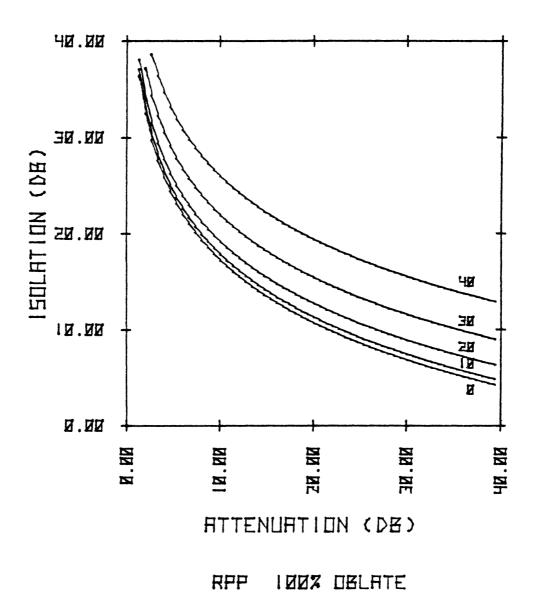
Figure 3.2-2. Isolation vs attenuation for canting angle standard deviations of 0, 10, 20, 30 and 40 degrees. f = 20 GHz. Circular polarization. Path length 8.2 km.
