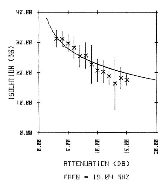
Figure 3.2-10. Isolation vs attenuation measured at VPI&SU using the Comstar D2 satellite. August 1977. Linear polarization.
