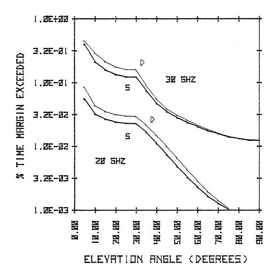
Figure 5.3-2. Percent of time a 15 dB at 5° elevation angle margin will be exceeded.
