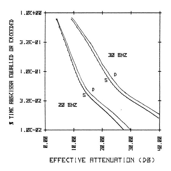
Figure 5.2-7. Percent of time a given A<sub>eff</sub> is exceeded for dual (D) and single (S) polarized systems. Elevation angle is 45°.
