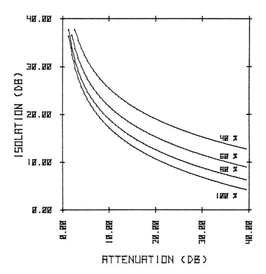
Figure 3.2-1. Isolation vs attenuation for 40, 60, 80 and 100% oblate raindrops. f = 20 GHz. Circular polarization. Path length 8.2 km.
