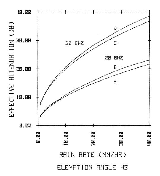
Figure 5.2-3. Effective attenuation  $(A_{eff})$  for a dual (D) and single (S) polarized system as a function of rain rate.
