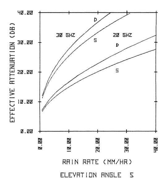
Figure 5.2-1. Effective attenuation  $(A_{eff})$  for a dual (D) and single (S) polarized system as a function of rain rate.
