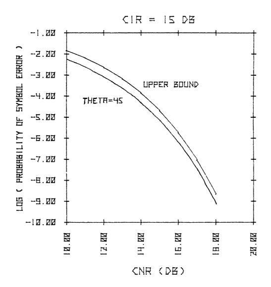
Figure 2.2-1. QPSK Probability of error; upper bound and exact.
