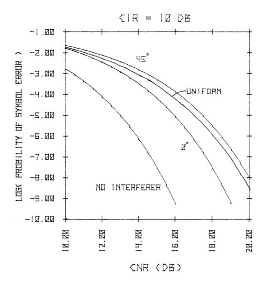
Figure 2.1-3. QPSK Probability of symbol error vs CNR.
