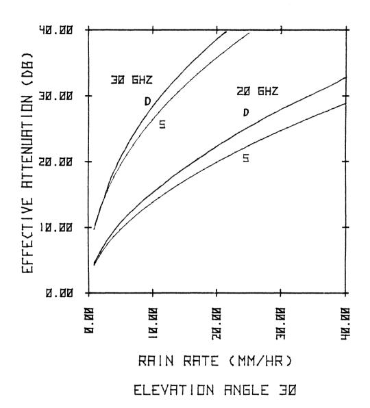
Figure 5.2-2. Effective attenuation ( $A_{eff}$ ) for a dual (D) and single (S) polarized system as a function of rain rate.
