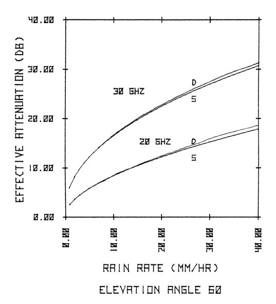
Figure 5.2-4. Effective attenuation ( $A_{eff}$ ) for a dual (D) and single (S) polarized system as a function of rain rate.
