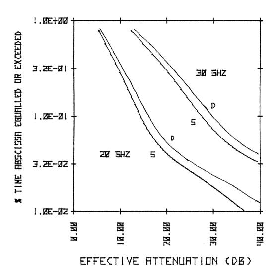
Figure 5.2-6. Percent of time a given A<sub>eff</sub> is exceeded for dual (D) and single (S) polarized systems. Elevation angle is 30°.
