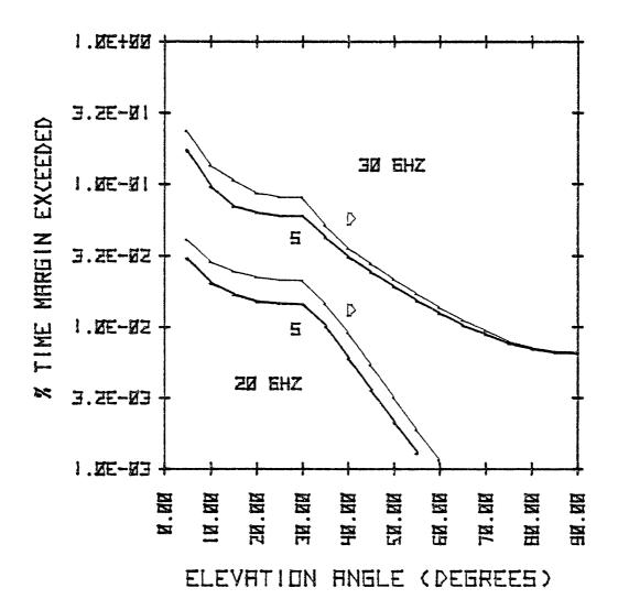
Figure 5.3-3. Percent of time a 20 dB at 5° elevation angle margin will be exceeded.
