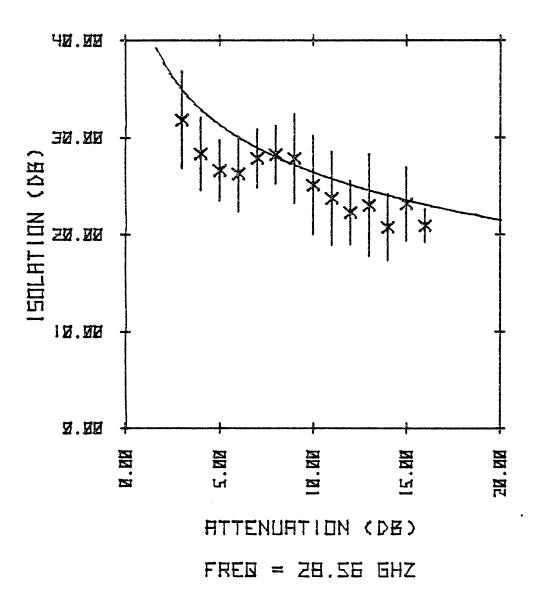
Figure 3.2-9. Isolation vs attenuation measured at VPI&SU using the Comstar D2 satellite. August 1977. Linear polarization.
