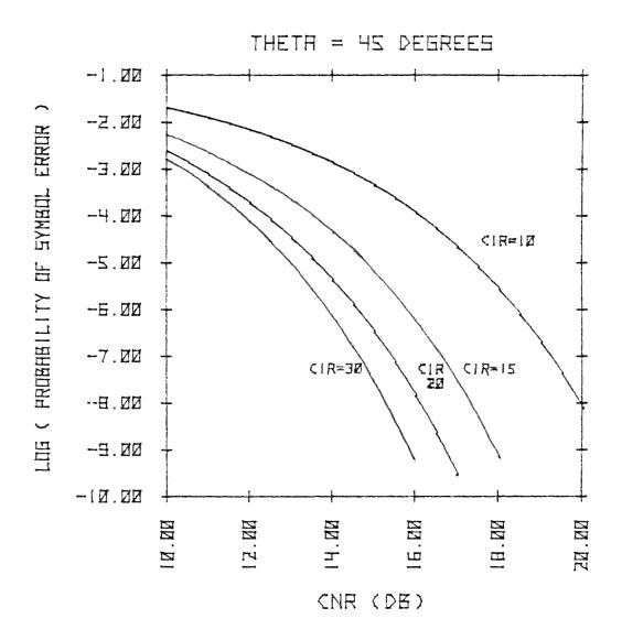
Figure 2.1-4. QPSK Probability of symbol error vs CNR for various CIR values.
