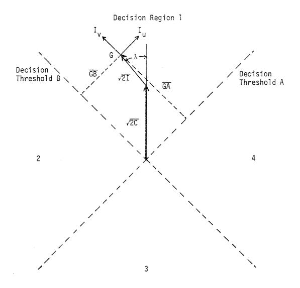
Figure 2.1-1. Phasor diagram of a QPSK signal and interference.
