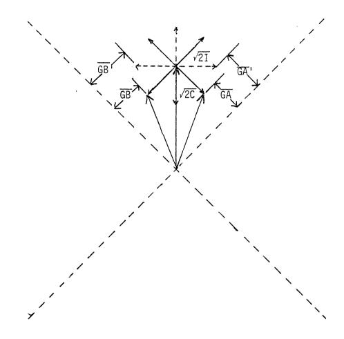
Figure 2.1-2. QPSK signal with interference.
