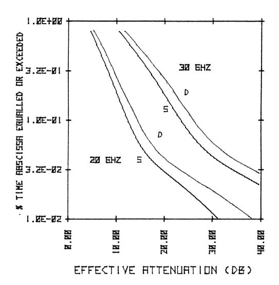
Figure 5.2-5. Percent of time a given  $A_{\mbox{eff}}$  is exceeded for dual (D) and single (S) polarized systems. Elevation angle is 5°.
