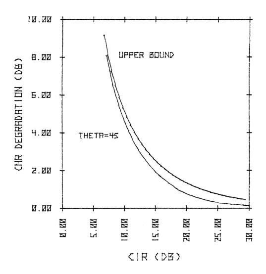
Figure 2.3-2. CNR Degradation: Exact for relative phase shift of 45° and upper bound.
