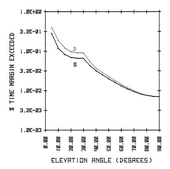
Figure 5.3-4. Percent of time a 10 dB margin at an elevation angle of 5° will be exceeded in the MWCE transponder mode.
