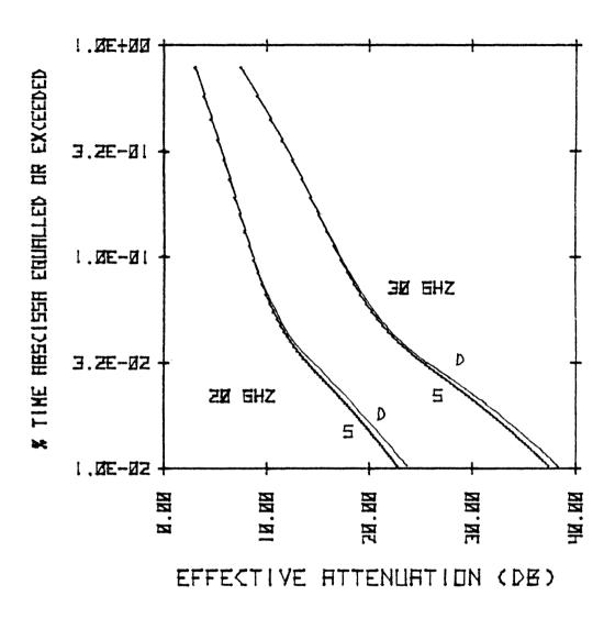
Figure 5.2-8. Percent of time a given A<sub>eff</sub> is exceeded for dual (D) and single (S) polarized systems. Elevation angle is 60°.
