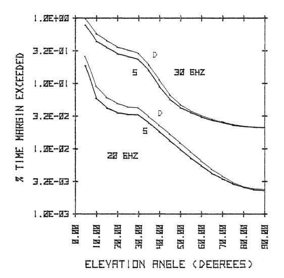
Figure 5.3-1. Percent of time a 10 dB at 5° elevation angle margin will be exceeded.
