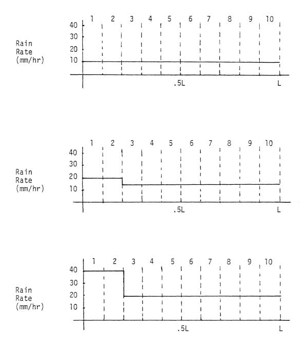
Figure 3.2-5. Synthetic storm algorithm.
