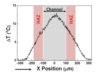
**Fig. 6** Thermal profile obtained along the scan line indicated in Fig. 5(b) that corresponds to the intra-channel temperature rise induced for an electrical field of 500 V cm $^{-1}$  and a flow rate of 2  $\mu$ L min $^{-1}$ . The extension of the electroporation channel (200  $\mu$ m in length) is indicated together with the Heat Affected Zones created at both sides (HAZ).
