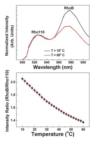
Fig. 2 (a) Emission spectra of the solution containing both Rhodamine B and Rhodamine 110 as obtained at two different temperatures (10 and 60 °C). (b) Temperature evolution of the ratio between the emitted intensities generated from Rhodamine B and Rhodamine 110. Dots are experimental data and the solid line is the polynomial fit that is used for temperature sensing.
