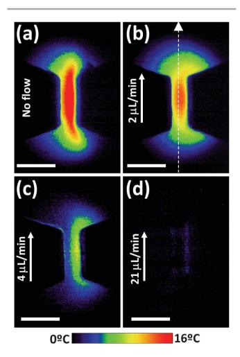
**Fig. 5** Thermal images of one of the narrow sections of the structure depicted in Fig. 1(a) in the presence of an applied electric field of 500 V cm $^{-1}$  as obtained for different flow rates. Arrow indicates the direction of the flow. Scale bar is 200  $\mu$ m in all the cases. Results obtained with the epi-fluorescence microscope described in the text.
