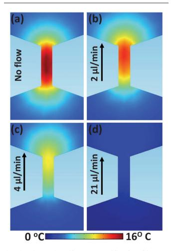
**Fig. 8** Thermal images obtained from COMSOL modelling of one of the narrow sections of the structure depicted in Fig. 1(a) under an applied electric field of 500 V cm<sup>-1</sup> as obtained for different flow rates. Arrow indicates the direction of the flow.
