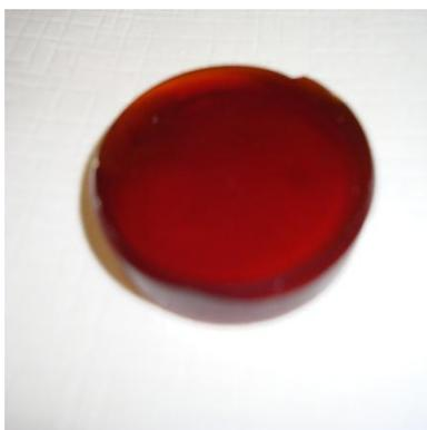
**Figure 5.1.** Acid-base catalyzed Fe/silica xerogel monolith.
