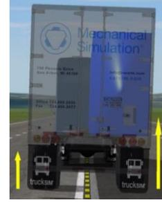
Figure 5. Back view of the truck model with shifted load in TruckSim
