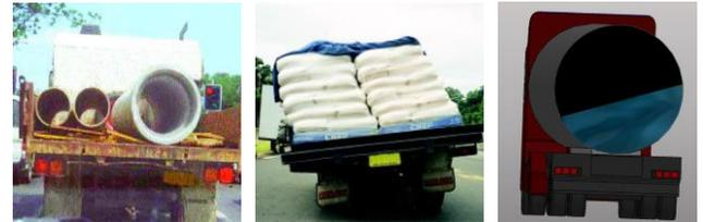
Figure 1. (a) Free rolling pipes [4]; (b) slippery bags shifting [4]; (c) liquid slosh occurrence
