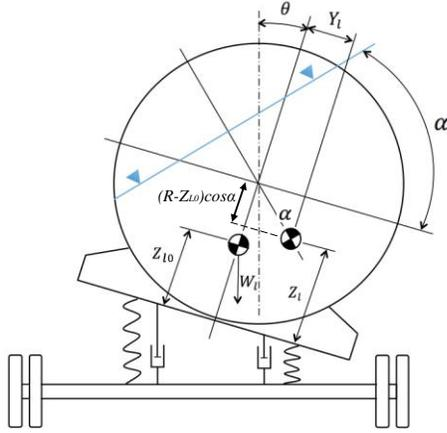
Figure 11. Roll-plane schematic of a partially-filled circular tank
