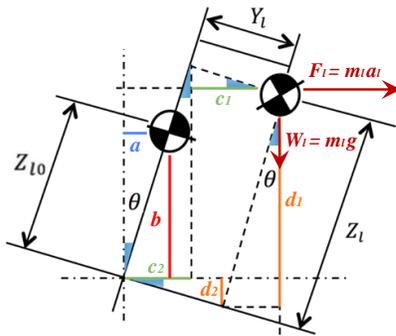
Figure 12. Instantaneous CG position of the liquid cargo
