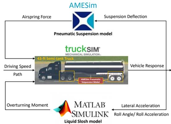
Figure 10. Co-simulation scheme for roll dynamics analysis of a 43-ft partially-filled tank truck
