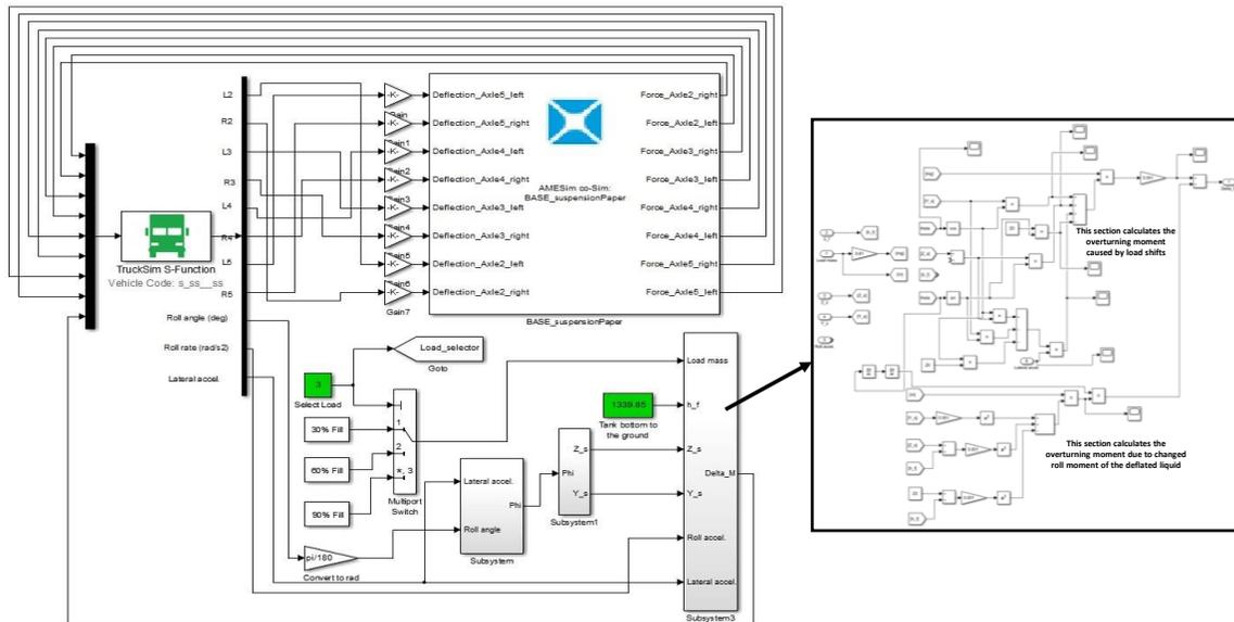
Figure A2. Co-simulation model established in Simulink for dynamic analysis of the tank truck
