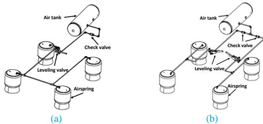
Figure 3. Plumbing configurations of (a) single and (b) dual leveling valve suspensions on the tractor's tandem axles or trailer's axles
