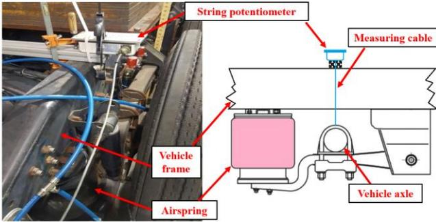
Figure 7. Installation of the string potentiometer
