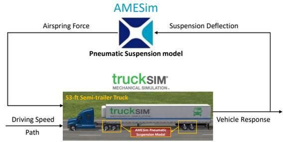
Figure 9. Co-simulation scheme for the roll dynamics analysis of the semi-trailer truck with a rigid off-center load
