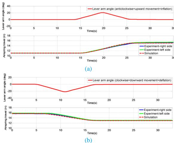
Figure 8. Comparison of simulation and experiment results of airspring displacement for (a) the supply and (b) purge tests
