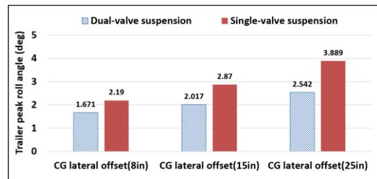
Figure 17. Summary results of trailer peak roll angle for 8-, 15-, and 25-in off-center loads
