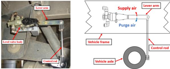
Figure 2. Installation and working process of the leveling valve
