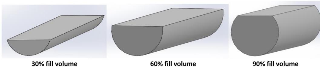
Figure A3. CAD models for determining the parameters for the slosh simulation
