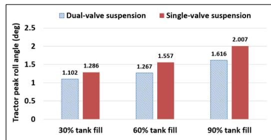
Figure 20. Summary results of tractor peak roll angle for 30%, 60%, and 90% fill volumes
