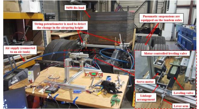
Figure 6. The pictorial view of a tractor static test setup
