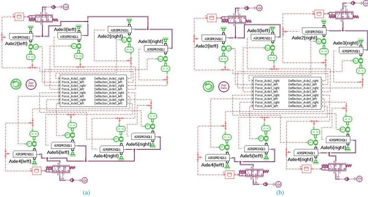
Figure A1. Pneumatic suspension models in AMESim: (a) single and (b) dual leveling valves
