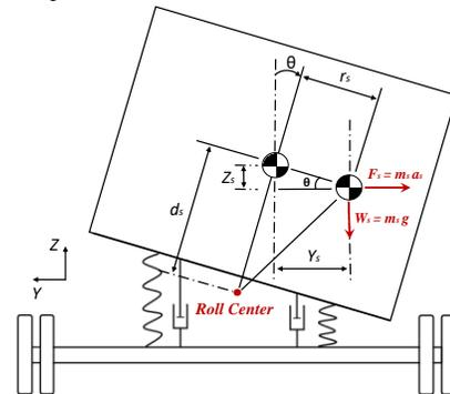
Figure 4. Roll-plane schematic of the truck with a rigid shifted load
