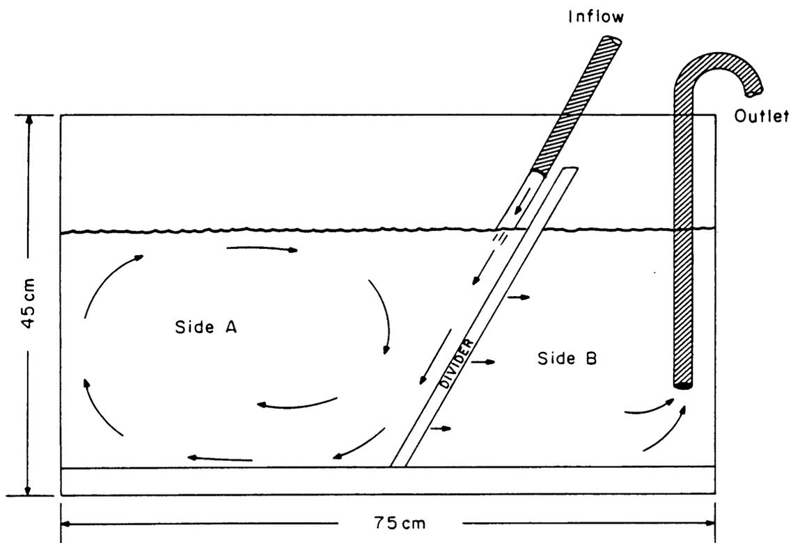
**Figure 5.** Profile of experimental chamber used to subject larval fish to high velocity water flows.
