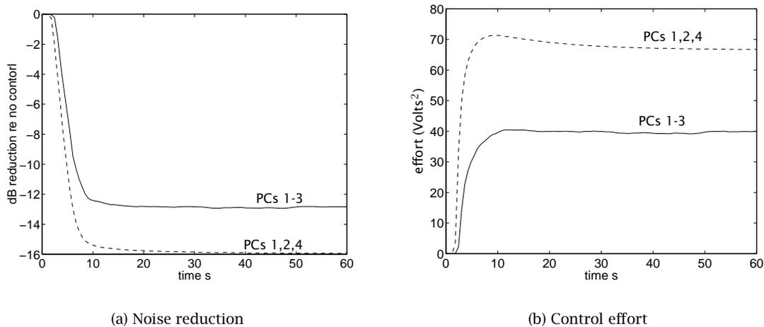
Figure 8.20: Noise reduction and control input for two PC subsets, 138 Hz
