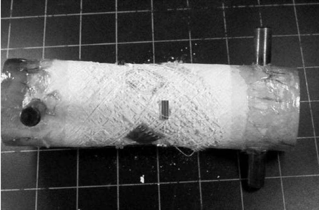
**Figure 3-7. Sample 7-6-16-C after tensile strength test.**
