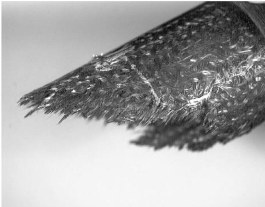
**Figure 3-23. Sample CVI 1219 failure surface with pullout**
