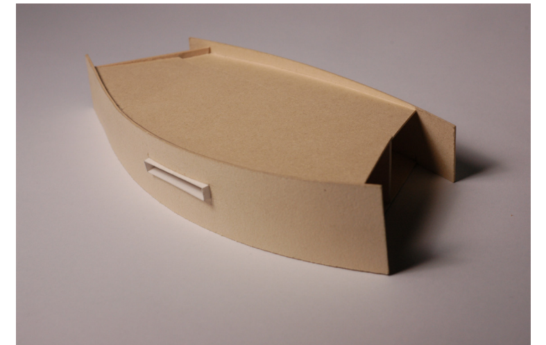
These photos show early design models to study the mass and the relationship of the outer walls to the roof and to the main central dividing wall. Studies show the slicing through the roof or varying the heights of the roof to control how much light comes into the main chapel space and the back wall of the altar.
