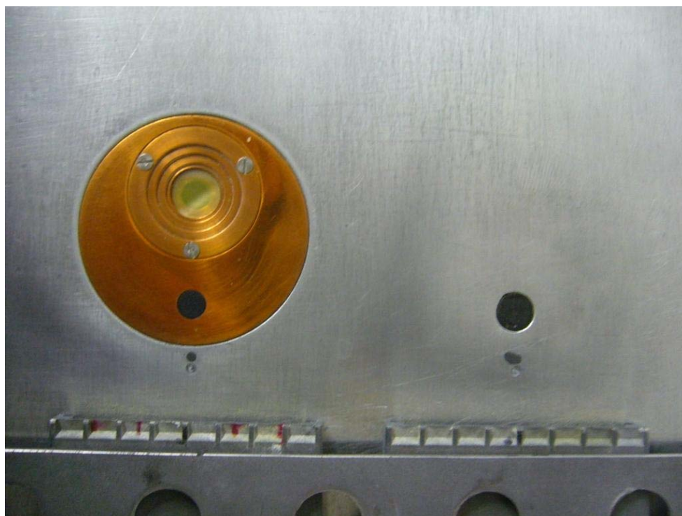
Figure 3.25: Picture of the plate for the 1.5 in. SB gages, showing the thermocouples mounted close to the SB and HFM (right).
