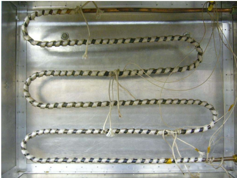
Figure 3.12: Interior view of the air heater: Copper coil with heater tape.
