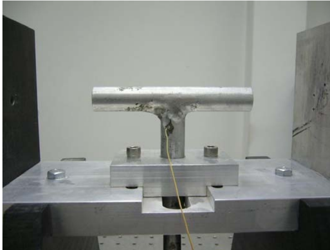
Figure 3.29: Thermocouple location to measure the air temperature.
