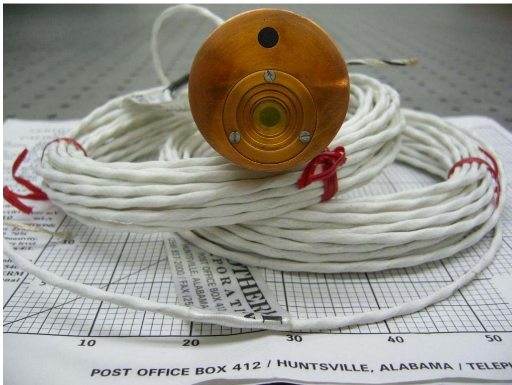
Figure 3.8: Front view of a 1.5 in. SB gage. The black area is the heat flux sensing area. The black area behind the window is the heat flux sensing area for radiation.
