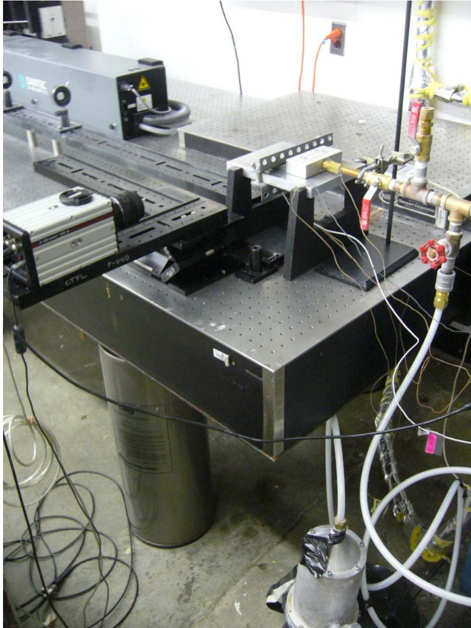
Figure A19: Photo of the PIV Experiment Setup in the CTFS at the VT ME department. Laser, lenses, camera, shear stand and seeder.
