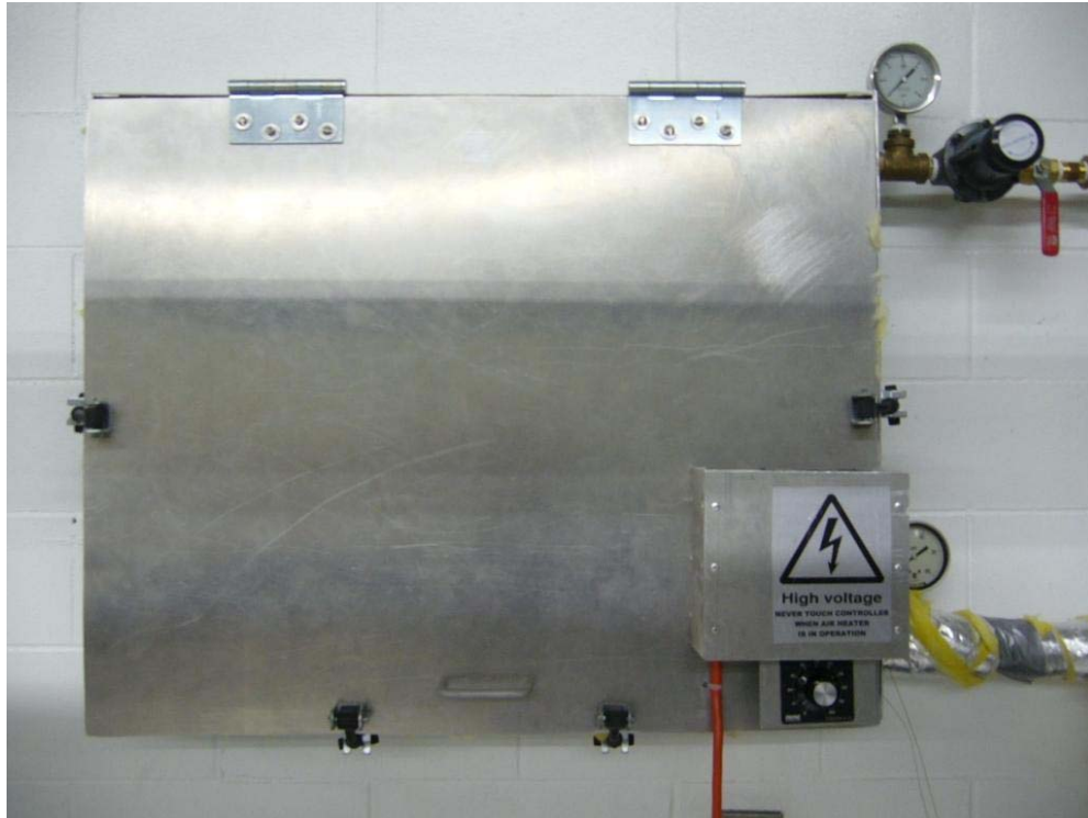
Figure 3.11: Exterior view of the air heater with power module and control potentiometer.
