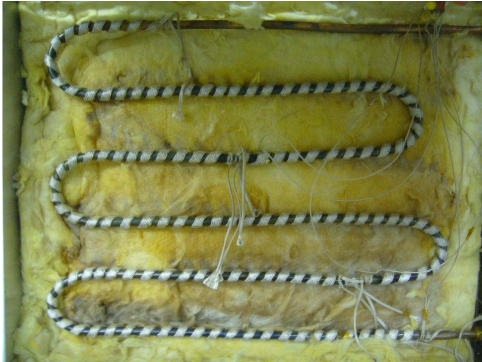
Figure 3.13: Heater interior with glass fiber foam.
