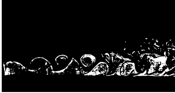
Figure A4: Streamwise flow visualization for a forced jet. Transition from Laminar to turbulent flow can be seen [14].
