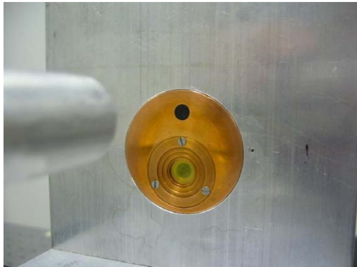
Figure 3.32: Thermocouple location for the 1.5 in. SB gage plate.
