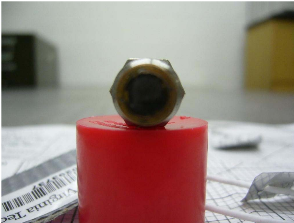
Figure 3.10: Front view of the HFM. The black area is the heat flux sensing area
