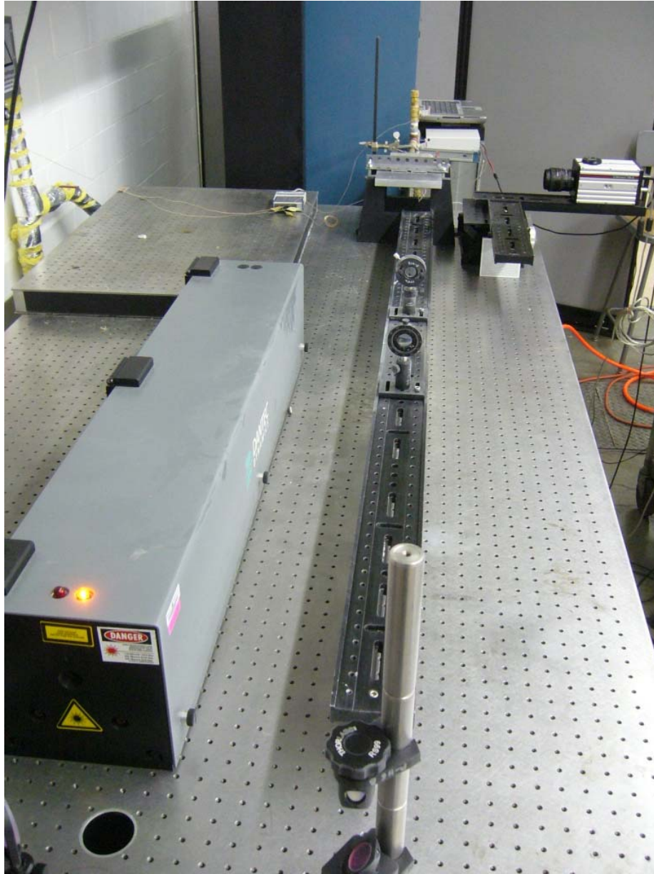
Figure A18: Photo of the PIV Experiment Setup in the CTFS at the VT ME department. Laser, lenses, camera and shear stand.
