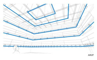
Figure 4: ICAT Cube's HDLA split into layers, including the ceiling raster. Space render courtesy of ARUP Inc.
