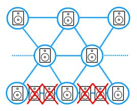
Figure 3: VBAP's selective use of loudspeakers in irregular layered loudspeaker configurations.
