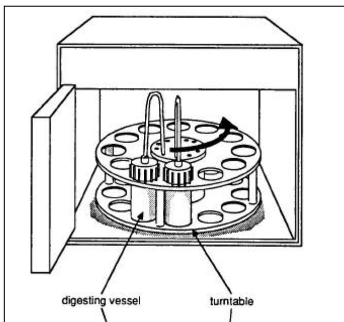
**Figure 13:** Schematic of a Closed-Vessel System (46)
