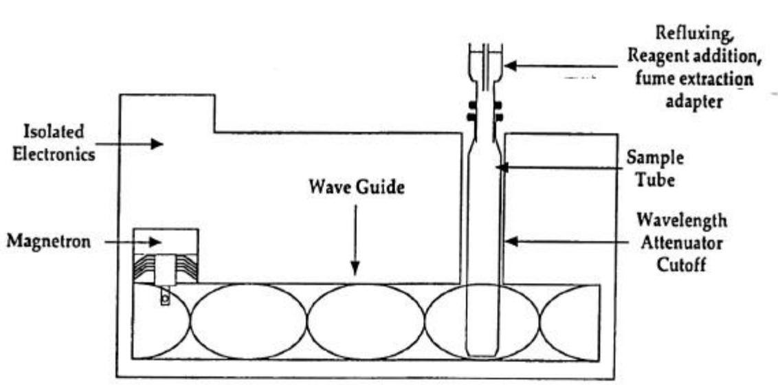
**Figure 14:** Schematic of a Focused Microwave System (48)
