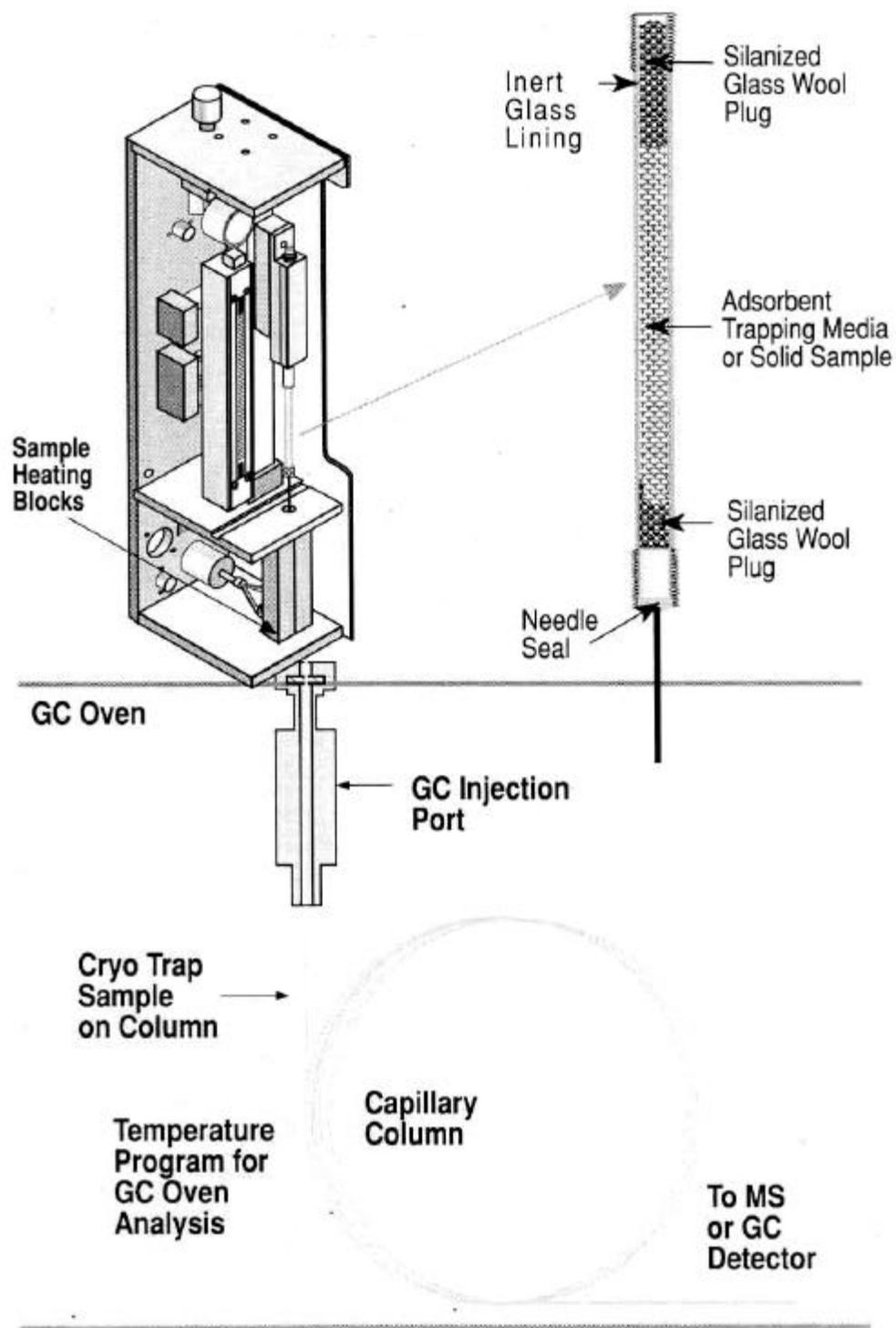
**Figure 10:** Schematic of Thermal Desorption Unit (23)
