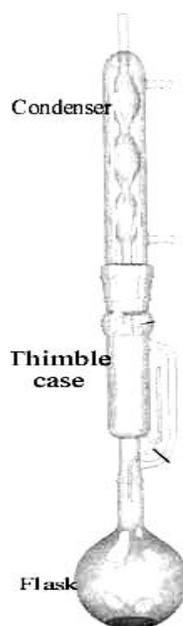
**Figure 9:** Schematic of Soxhlet Extraction Apparatus (19)
