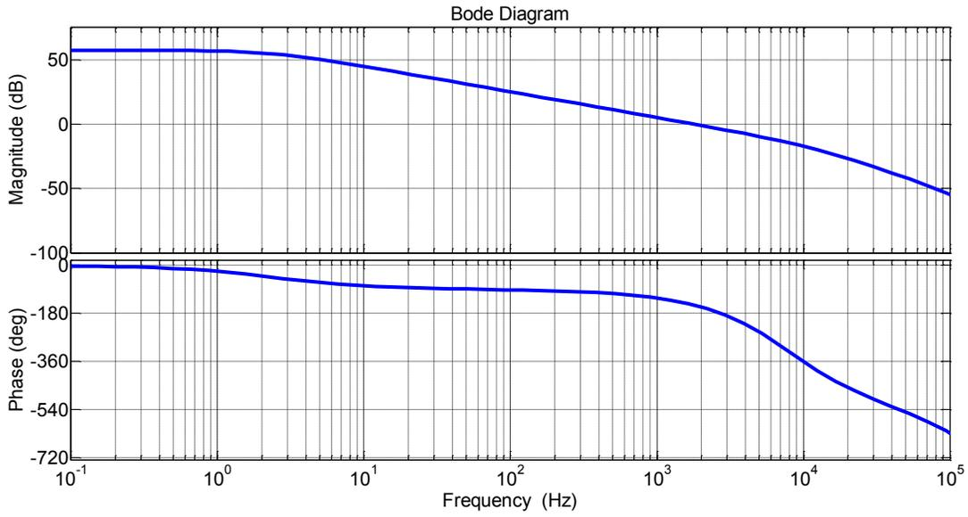
**Figure 6-8: Bode diagram of the current loop gain transfer function  $T_{ilt}(s)$**
