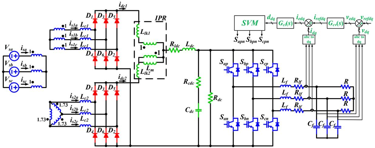
**Figure 4-7: Twelve-pulse diode rectifier feeding an actively controlled three-phase VSI**
