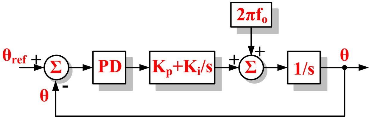
**Figure 2-13: Block diagram of the linearized model of SRF PLL**
