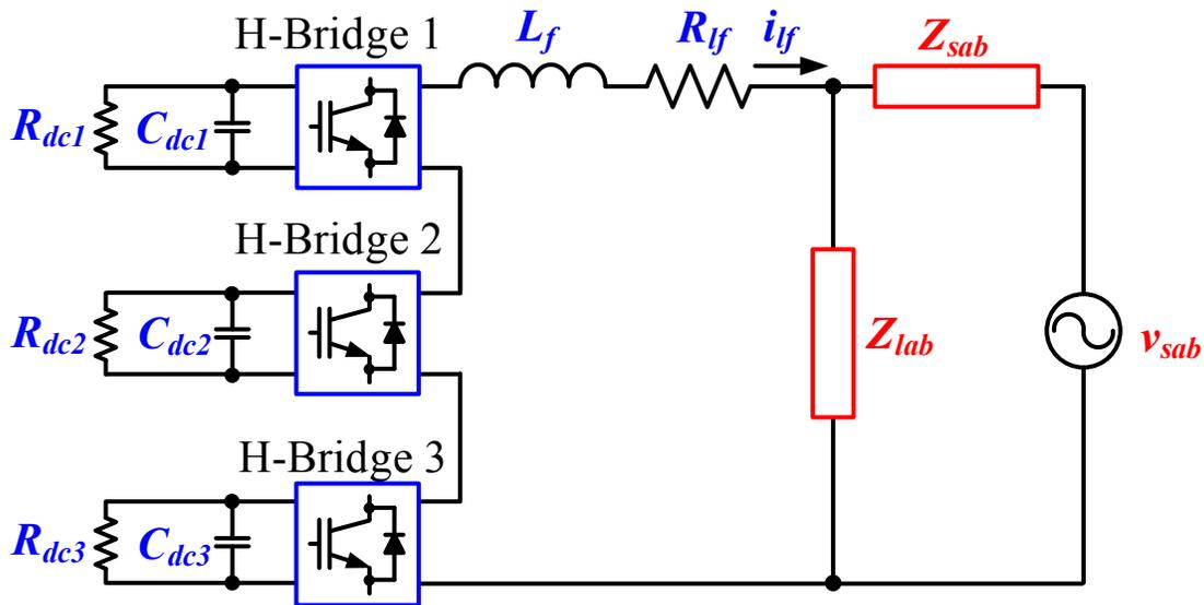
**Figure 5-5: Equivalent switching model multi-level cascaded H-bridge circuit**
