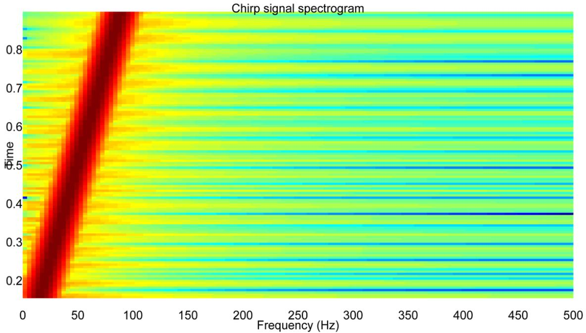
**Figure 2-5: Spectrogram of a chirp signal**
