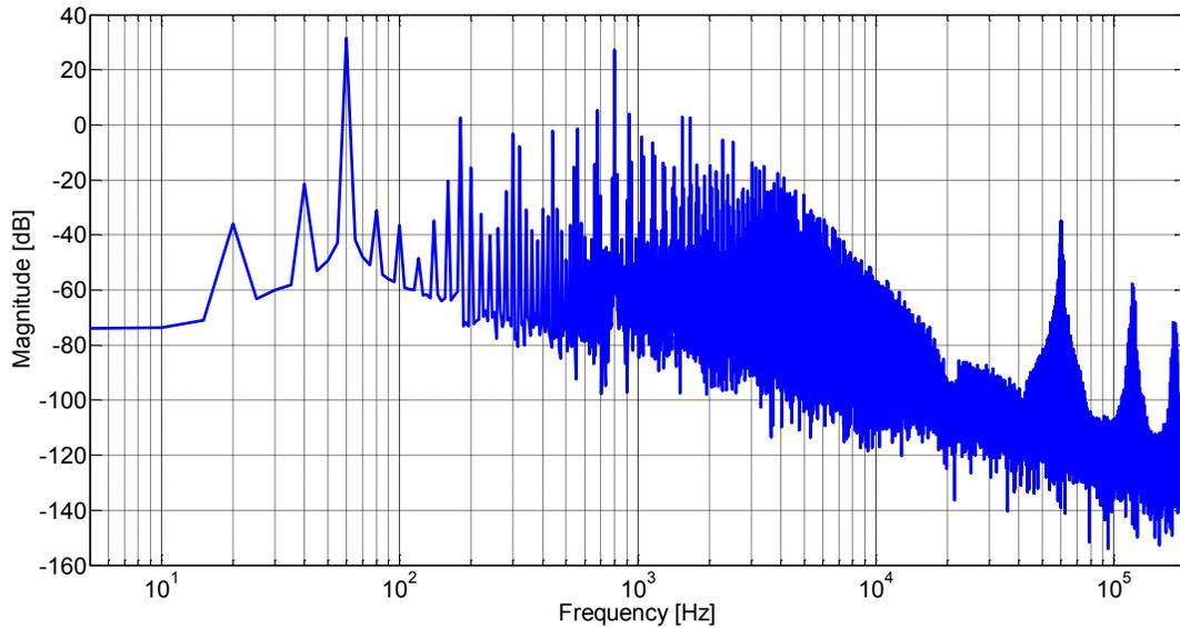
**Figure 6-22: Harmonic spectrum of the capacitor injection voltage  $v_{c}(t)$**
