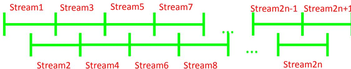
**Figure 2-22: Splitting of a signal into the overlapping stream of sections**
