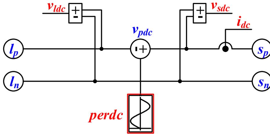
Figure 2-11: Series voltage injection dc measurement block
