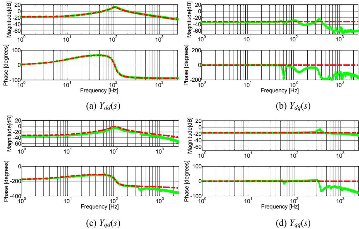
**Figure 4-5: Small-signal input dq admittance of twelve-pulse diode rectifier: obtained from switching simulation model (green line with squares), analytical expression of modified AAVM (red dashed line).**
