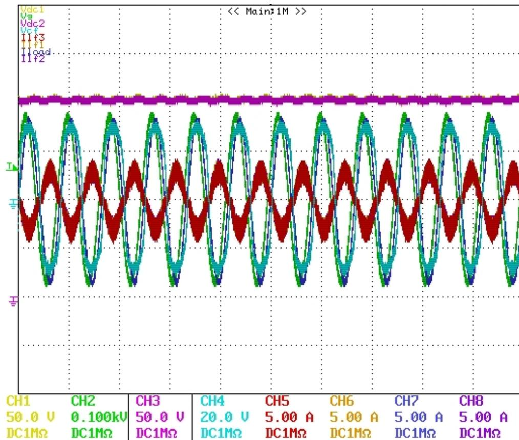
Figure 6-24: Experimental scope waveforms of source voltage  $v_s(t)$ , load system current  $i_{load}(t)$ , inductor currents  $i_{f1}(t)$ ,  $i_{f2}(t)$ ,  $i_{f3}(t)$ , and dc voltages  $v_{dc1}(t)$ ,  $v_{dc2}(t)$  and injection voltage  $v_c(t)$
