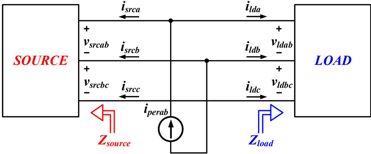
Figure 7-1: Ideal Single-Phase Shunt Current Injection
