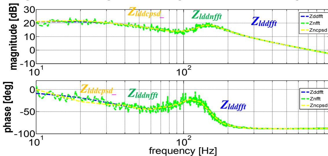
Figure 2-25: Load impedance  $Z_{ldd}$  comparison for FFT and CPSD algorithms
