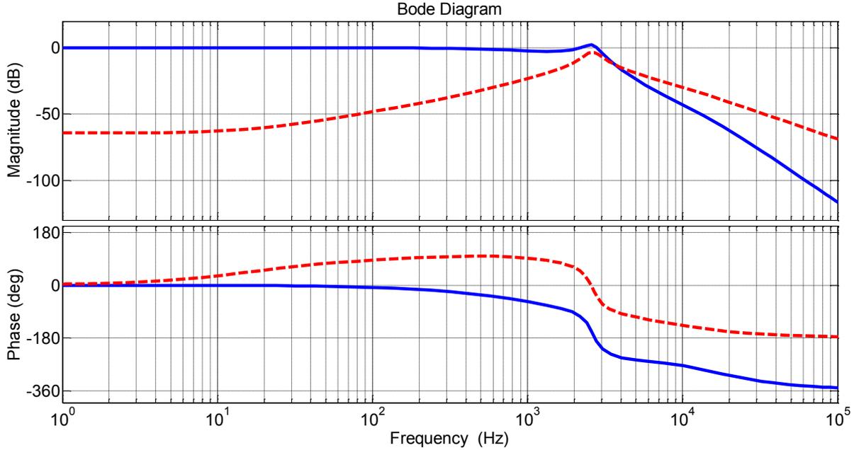
**Figure 6-9: Bode diagrams of the closed loop transfer function (a)  $G_{clvcf1}(s)$  (straight blue line) (b)  $G_{clvcf2}(s)$  (dashed red line)**
