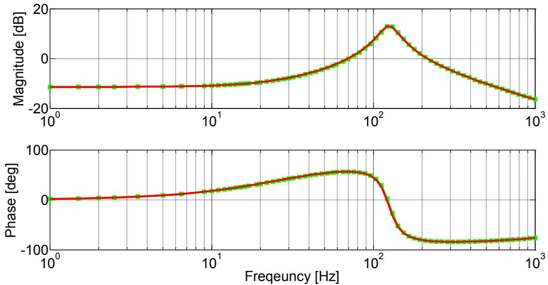
**Figure 3-4: Small-signal output DC impedance of six-pulse diode rectifier: obtained from switching simulation model (green line with squares) and analytical expression of AAVM (red dashed line)**
