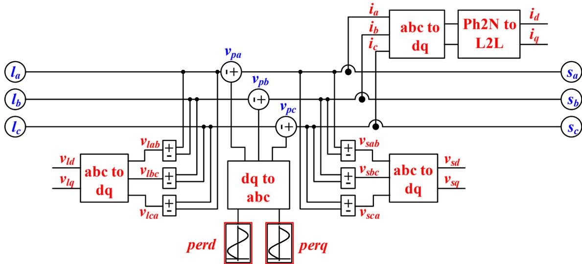
**Figure 2-9: Series voltage injection dq measurement block, which provides phase to neutral dq impedances**
