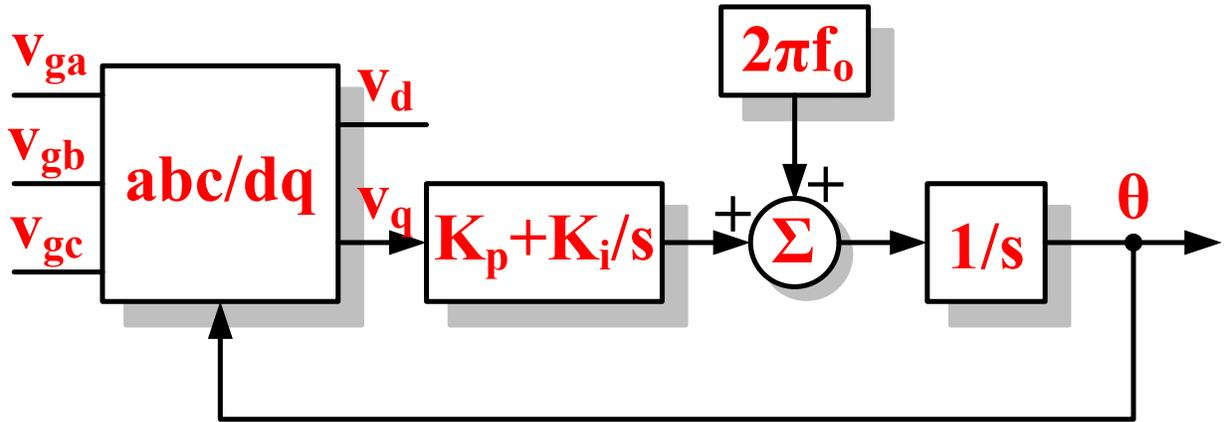
**Figure 2-12: Block diagram of the realized SRF PLL block**
