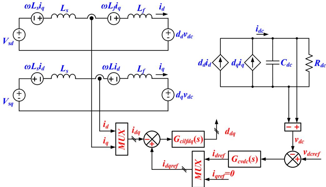
**Figure 2-19: Classical dq averaged model of three-phase boost rectifier**
