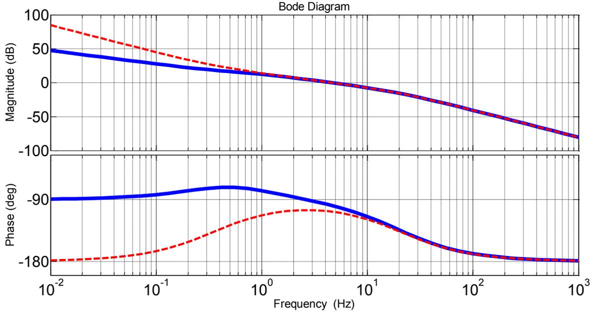
**Figure 6-11: Bode diagram of dc the voltage loop gain transfer function  $T_{vdc}(s)$ : (a) With  $R_{dc}=1 \text{ k}\Omega$  (straight blue line) (b) Without dc resistors (dashed red line)**
