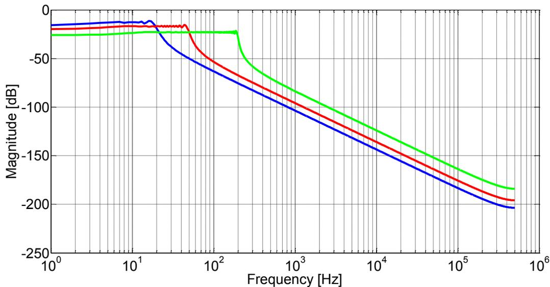
**Figure 2-7: Comparison of magnitude characteristics of three chirp signals:  $f_0=10$  Hz,  $f_1=20$  Hz and  $T=1$  s (blue straight line),  $f_0=10$  Hz,  $f_1=50$  Hz and  $T=1$  s (red dashed line),  $f_0=10$  Hz,  $f_1=200$  Hz and  $T=1$  s (green dotted line)**
