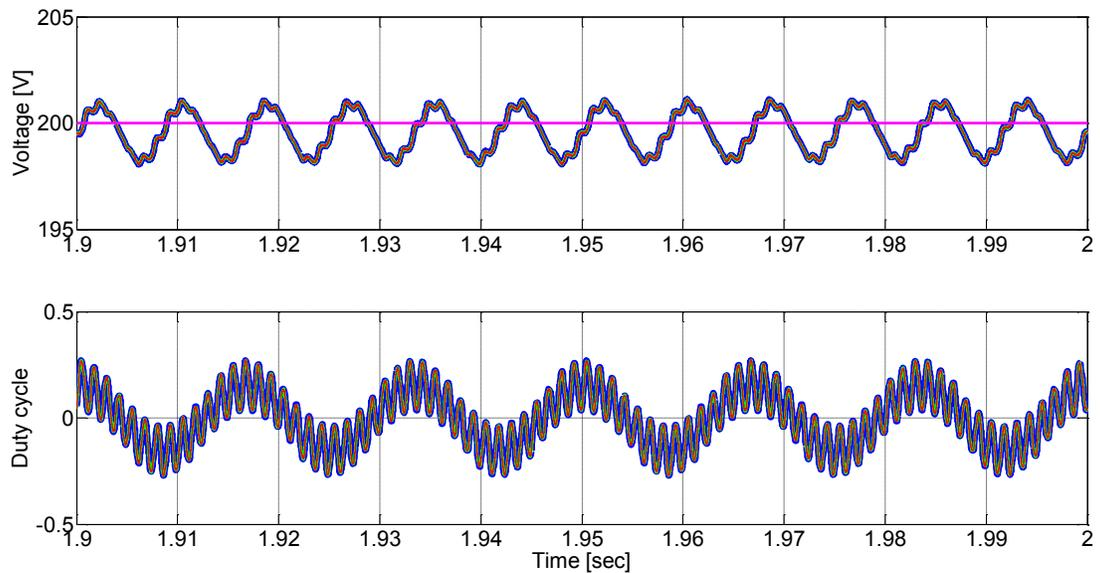
**Figure 6-21: Steady state simulation waveforms for high frequency (800Hz) injection: (top) dc voltages  $v_{dc1}(t)$ ,  $v_{dc2}(t)$ ,  $v_{dc3}(t)$  and dc reference voltage  $v_{dcref}(t)$  (bottom) H-bridge duty cycles  $d_1(t)$ ,  $d_2(t)$  and  $d_3(t)$**
