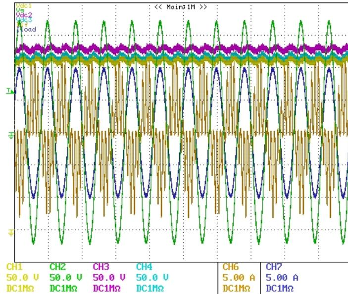
**Figure 5-16: Experimental waveforms of converter current  $i_{lf}(t)$ , load current  $i_{load}(t)$ , dc voltages  $v_{dc1}(t)$ ,  $v_{dc2}(t)$ ,  $v_{dc3}(t)$ , and source voltage  $v_g(t)$ .**
