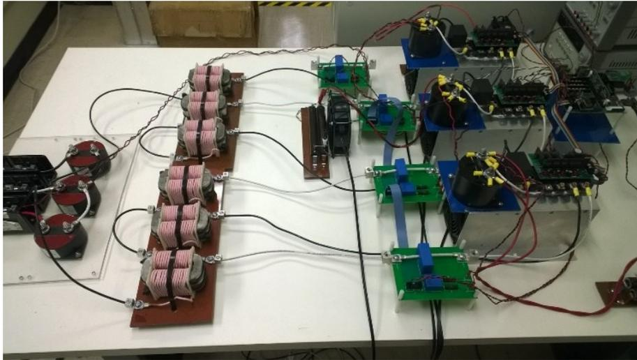
**Figure 5-15: Hardware prototype of the designed multi-level single-phase shunt current injection converter.**
