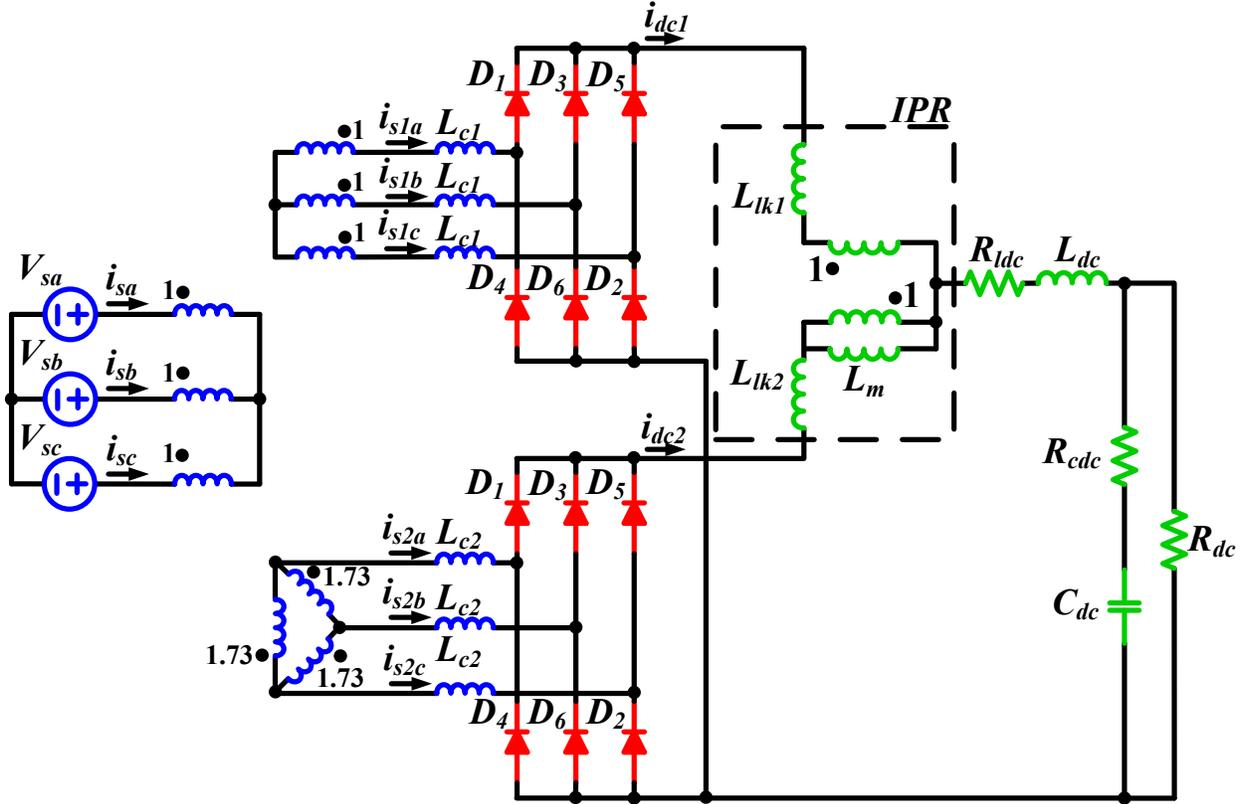
Figure 4-1: Switching model of twelve-pulse diode rectifier with resistive load.
