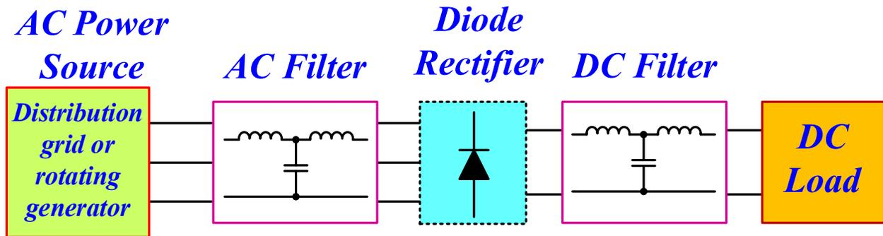
**Figure 1-2: Electrical schematic of commonly used front-end diode rectifier unit**
