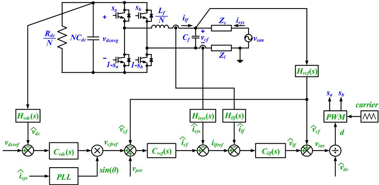
**Figure 6-5: The equivalent reduced order single-module model of SVI converter**
