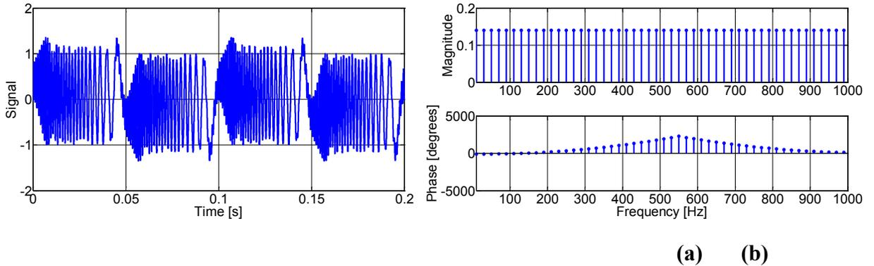
**Figure 2-2: Multi-tone signal (a) time-domain waveform (b) magnitude and phase characteristics in frequency domain**
