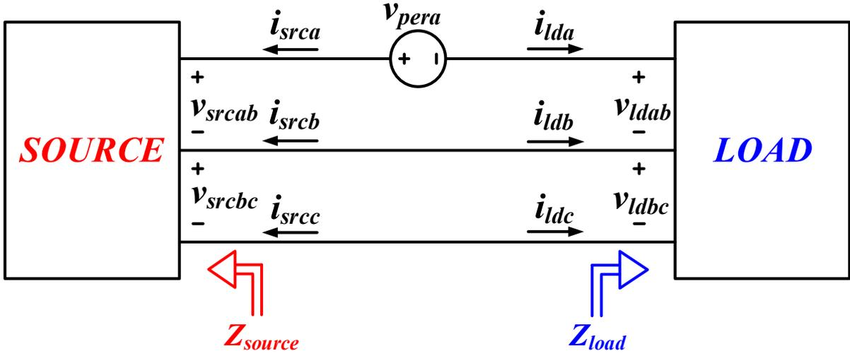
Figure 7-2: Ideal Single-Phase Series Voltage Injection
