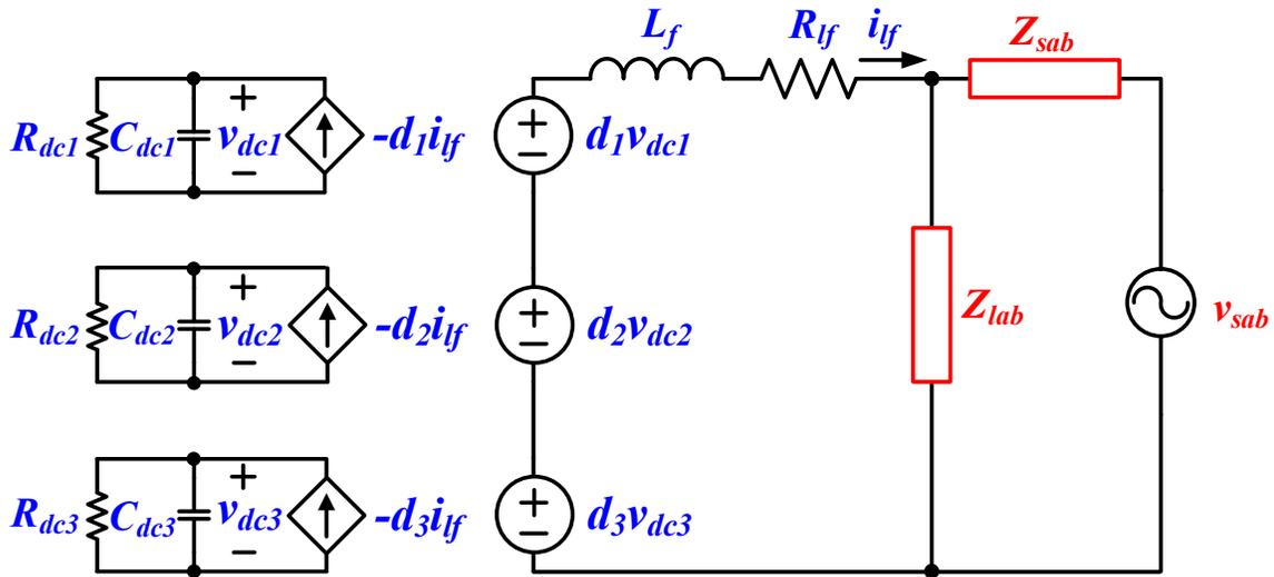
Figure 5-6: Equivalent multi-level cascaded H-bridge circuit
