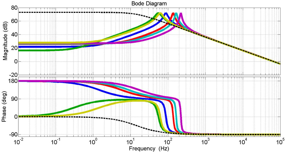
**Figure 5-8: Family of bode plots of control duty-cycle to inductor current plant transfer functions: straight lines represent bode diagram of  $G_{ifd}(s)$ , dashed line is bode diagram of  $G_{ifdcommon}(s)$**
