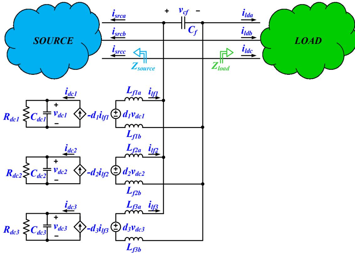
**Figure 6-3: Equivalent averaged model of single-phase interleaved series voltage injection converter, which is connected in series with a power system**
