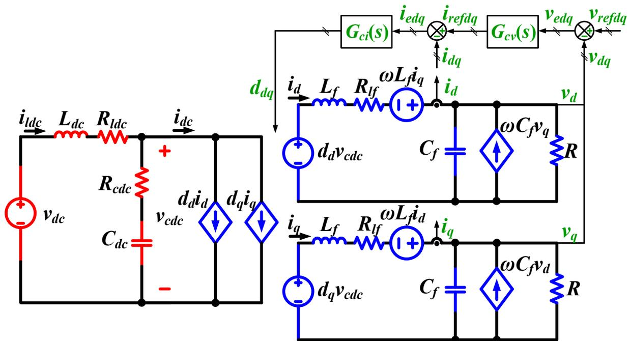
**Figure 2-15: Equivalent dq averaged model schematic of three-phase VSI**
