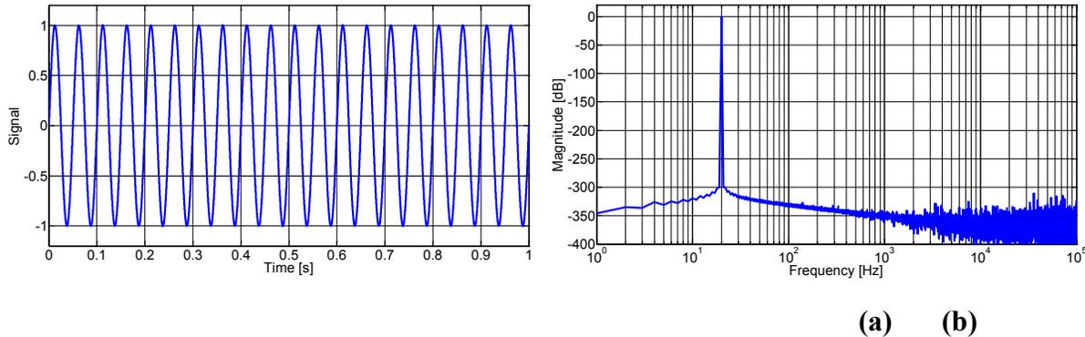
**Figure 2-1: Ideal sinusoidal signal (a) time-domain waveform (b) magnitude characteristic in frequency domain**
