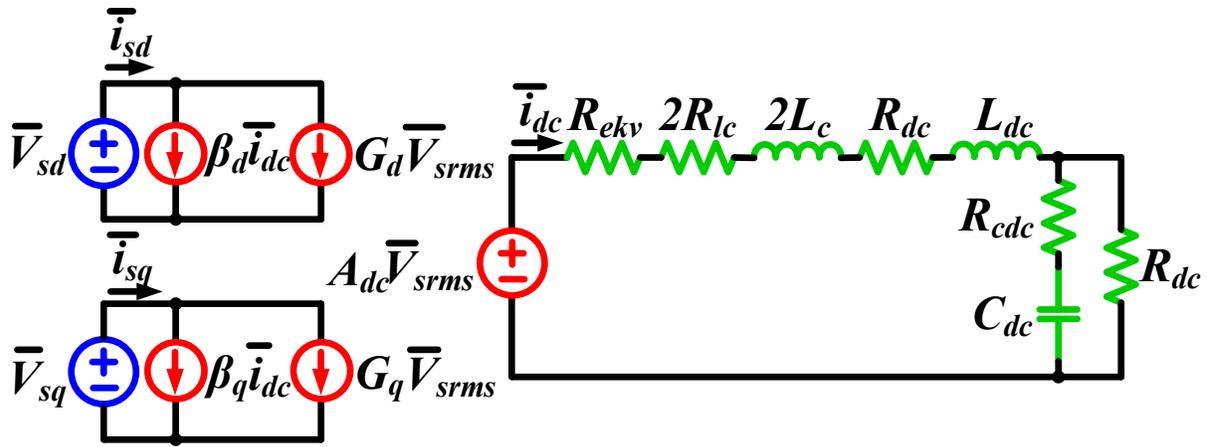
Figure 3-2: Equivalent averaged circuit schematic of AAVM.
