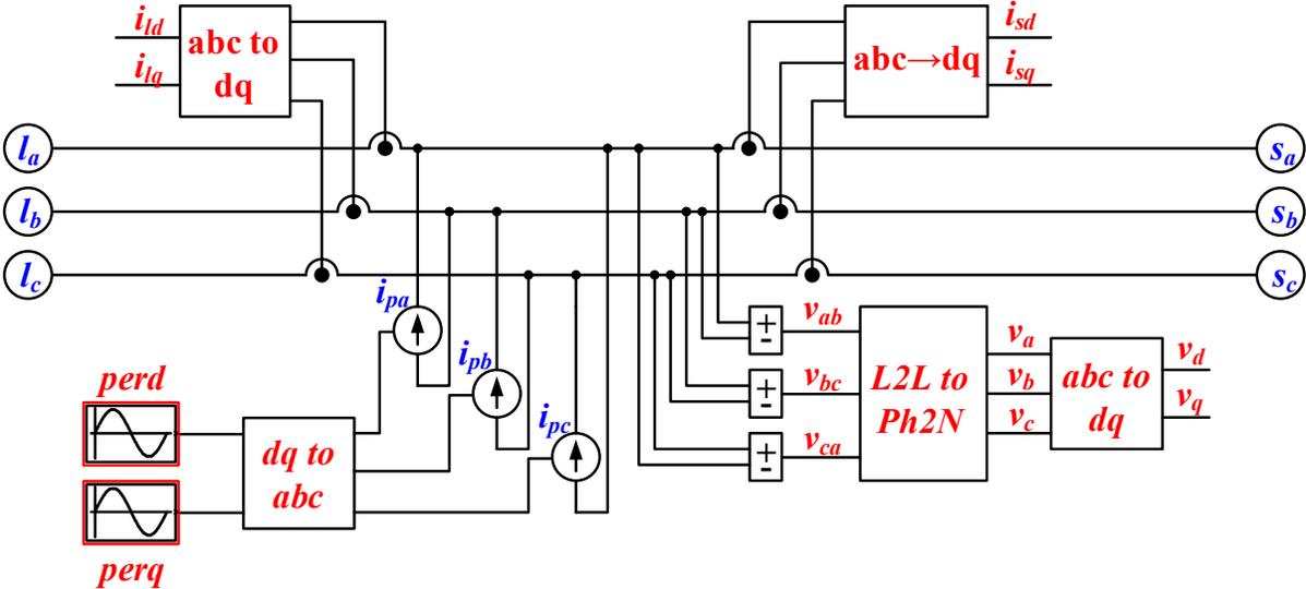
Figure 2-8: Shunt current injection dq measurement block, which provides phase to phase dq impedances
