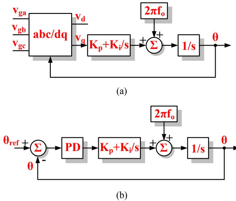
**Figure 5-3: Block diagrams of the realized SRF PLL block (a) Equivalent schematic (b) Equivalent small-signal linearized model**
