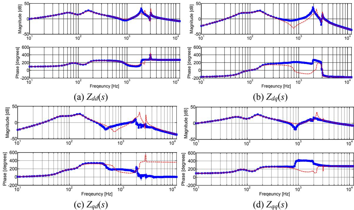
**Figure 2-16: Comparison of VSI output dq impedances obtained by switching model (squared blue line) and dq averaged model (dashed red line) (a)  $Z_{dd}(s)$  (b)  $Z_{dq}(s)$  (c)  $Z_{qd}(s)$  (d)  $Z_{qq}(s)$**
