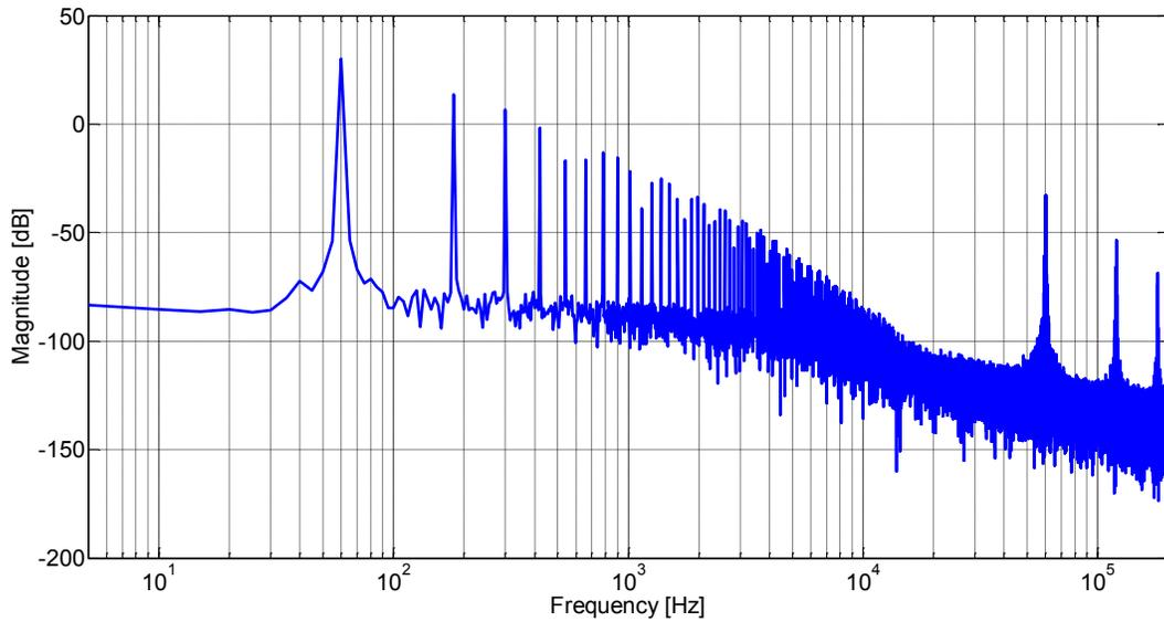
**Figure 6-14: Harmonic spectrum of the capacitor injection voltage  $v_{cf}(t)$**
