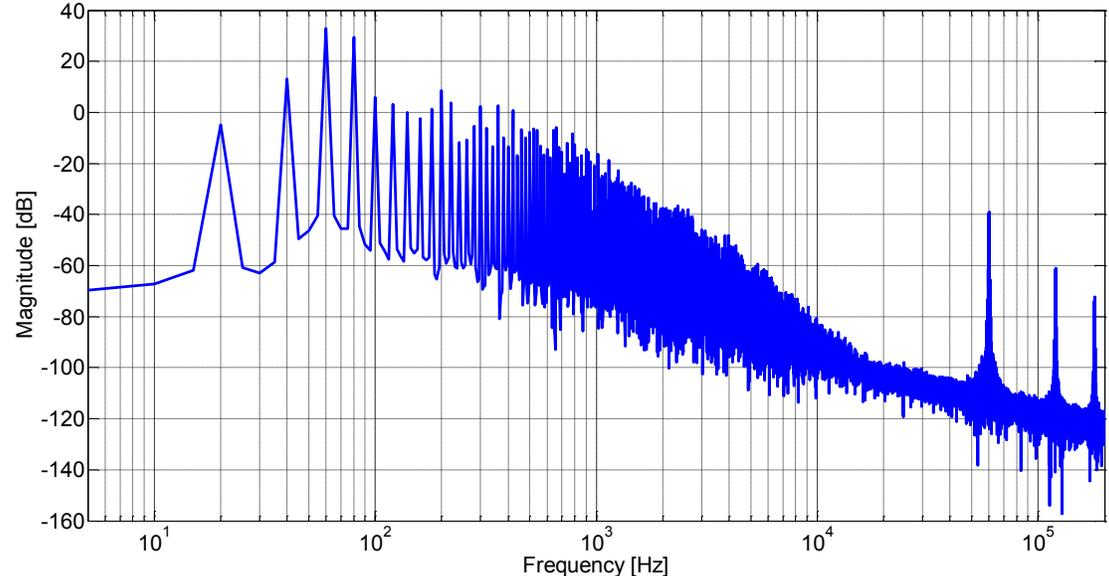
**Figure 6-18: Harmonic spectrum of the capacitor injection voltage  $v_{cf}(t)$**
