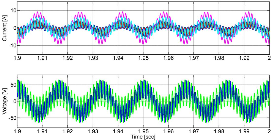
**Figure 6-20: Steady state simulation waveforms for high frequency (800 Hz) injection: (top) Inductor currents  $i_{f1}(t)$ ,  $i_{f2}(t)$ ,  $i_{f3}(t)$ , reference current  $i_{ref}(t)$  and system current  $-i_{sys}(t)$  (bottom) injection voltage  $v_{cf}(t)$  and reference voltage  $v_{ref}(t)$**
