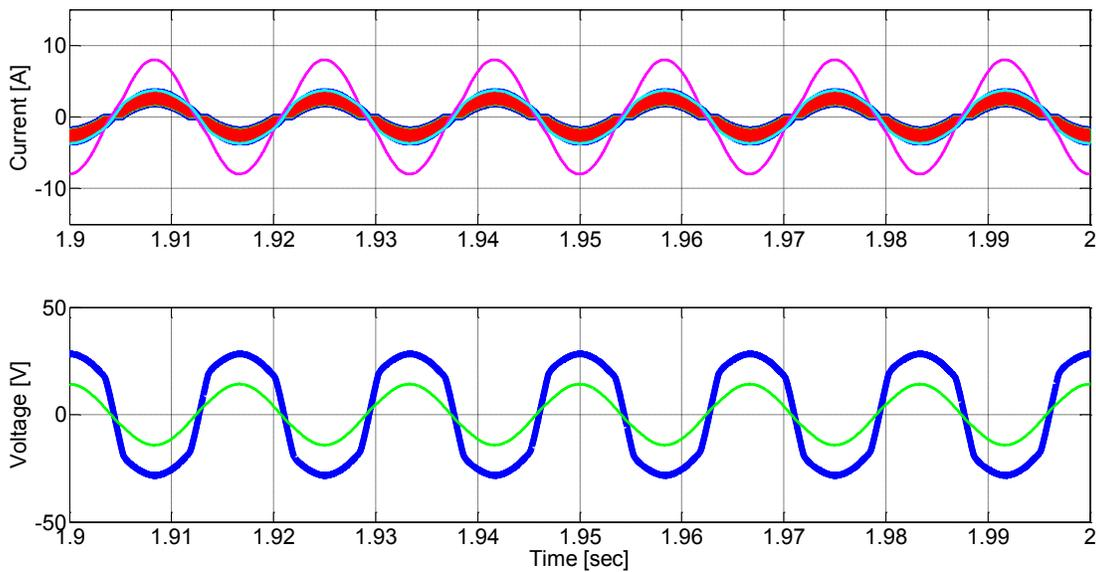
**Figure 6-12: Steady state simulation waveforms: (top) Inductor currents  $i_{l1}(t)$ ,  $i_{l2}(t)$ ,  $i_{l3}(t)$ , reference current  $i_{ref}(t)$  and system current  $-i_{sys}(t)$  (bottom) injection voltage  $v_{cf}(t)$  and reference voltage  $v_{ref}(t)$**
