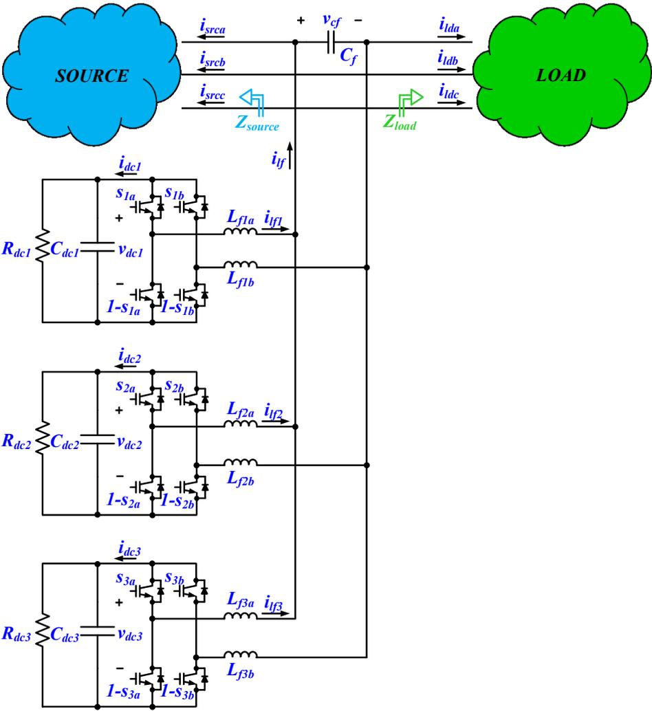
**Figure 6-1: Interleaved single-phase series voltage injection converter with H-bridge modules**
