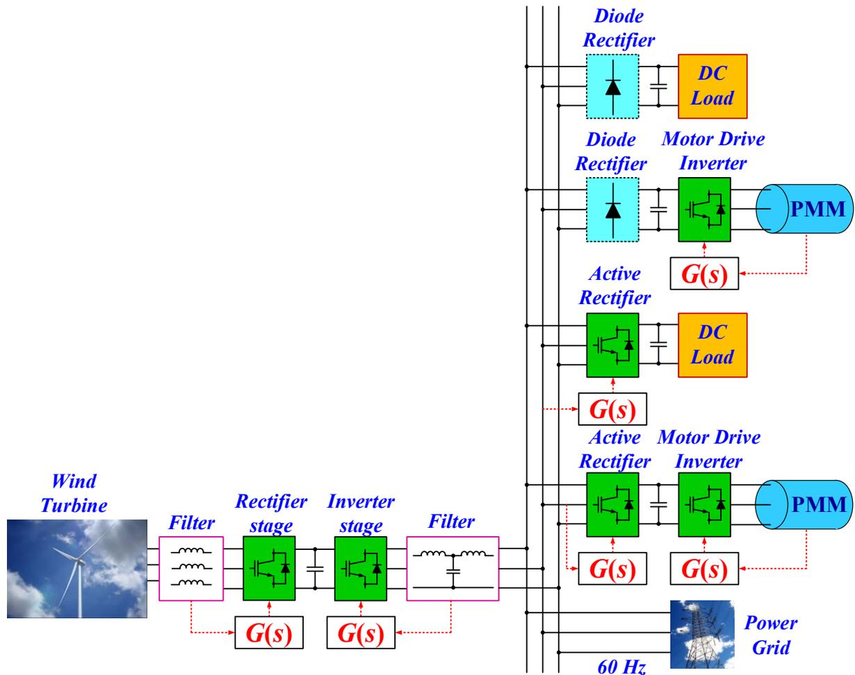
**Figure 1-1: Electrical schematic of modern power grid with majority of source and load power electronics converters**
