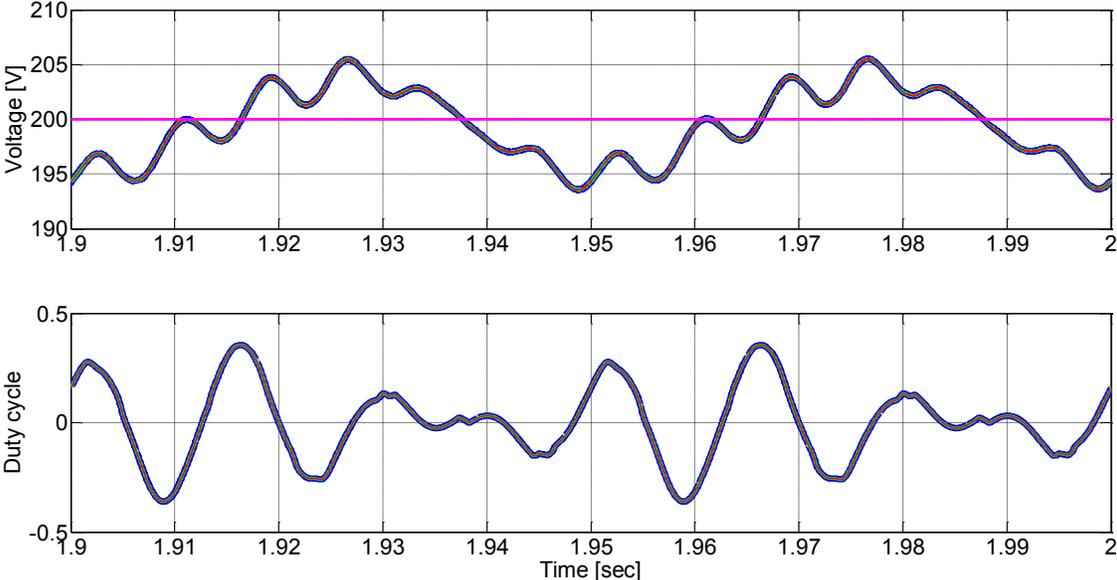
**Figure 6-17: Steady state simulation waveforms: (top) dc voltages  $v_{dc1}(t)$ ,  $v_{dc2}(t)$   $v_{dc3}(t)$  and dc reference voltage  $v_{dcref}(t)$  (bottom) H-bridge duty cycles  $d_1(t)$ ,  $d_2(t)$  and  $d_3(t)$**
