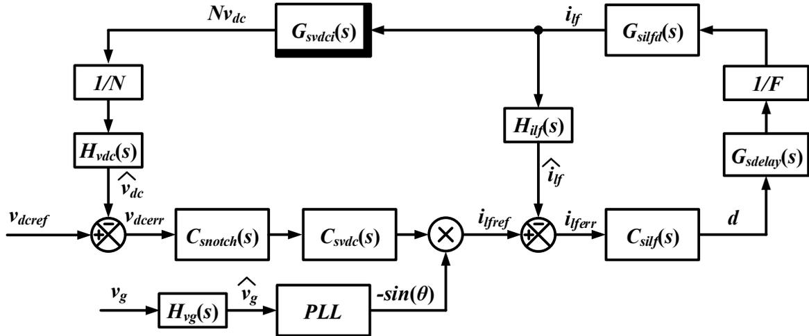
**Figure 5-9: Transfer function block diagram of proposed control**
