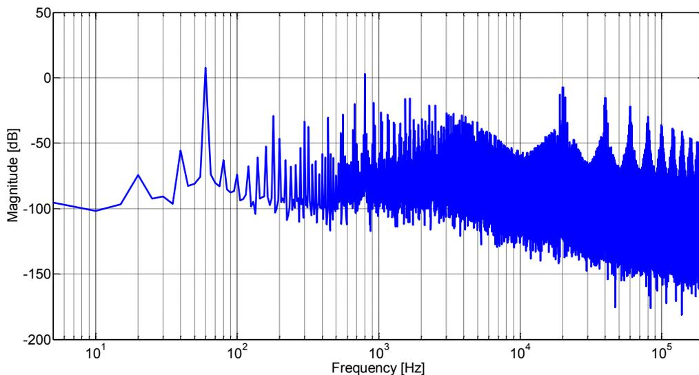
**Figure 6-23: Harmonic spectrum of the inductor current  $i_{l1}(t)$**
