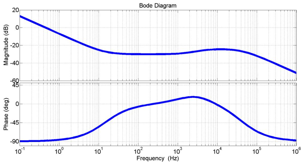
**Figure 5-10: Bode plot of the current controller transfer function**
