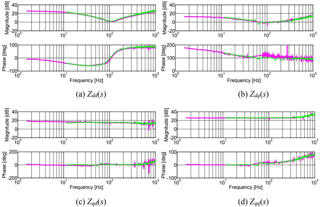
**Figure 4-6: Small-signal input dq impedance of twelve-pulse diode rectifier: obtained from switching simulation model (green line with squares), experimental measurements (purple line)**
