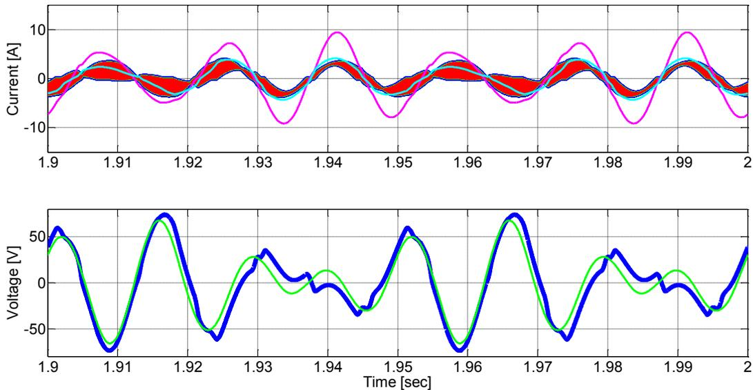
**Figure 6-16: Steady state simulation waveforms: (top) Inductor currents  $i_{lf1}(t)$ ,  $i_{lf2}(t)$ ,  $i_{lf3}(t)$ , reference current  $i_{ref}(t)$  and system current  $-i_{sys}(t)$  (bottom) injection voltage  $v_{cf}(t)$  and reference voltage  $v_{ref}(t)$**
