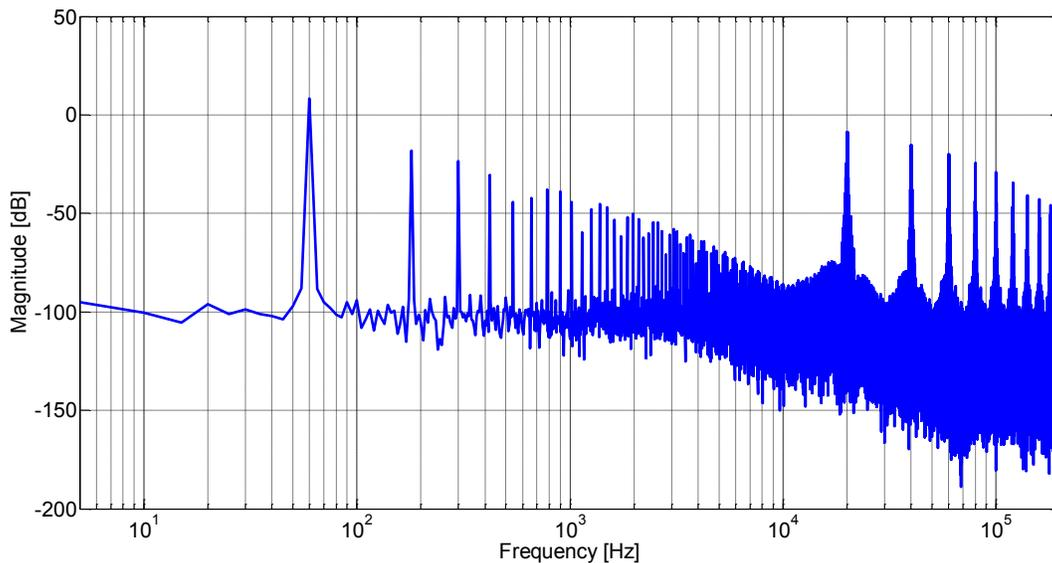
**Figure 6-15: Harmonic spectrum of the inductor current  $i_{lf1}(t)$**
