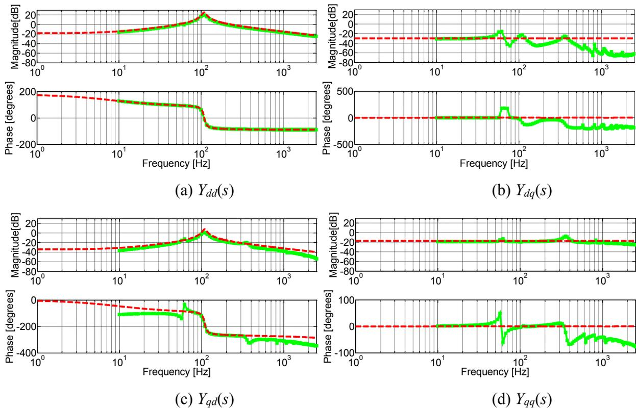
**Figure 4-9: Small-signal input dq admittance of twelve-pulse diode rectifier feeding a constant power load: switching simulation model (green line with squares), averaged model (dashed red line)**
