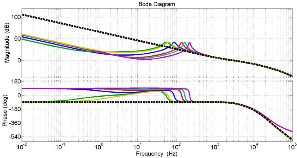
**Figure 5-11: Family of bode plots of current loop gain transfer functions**
