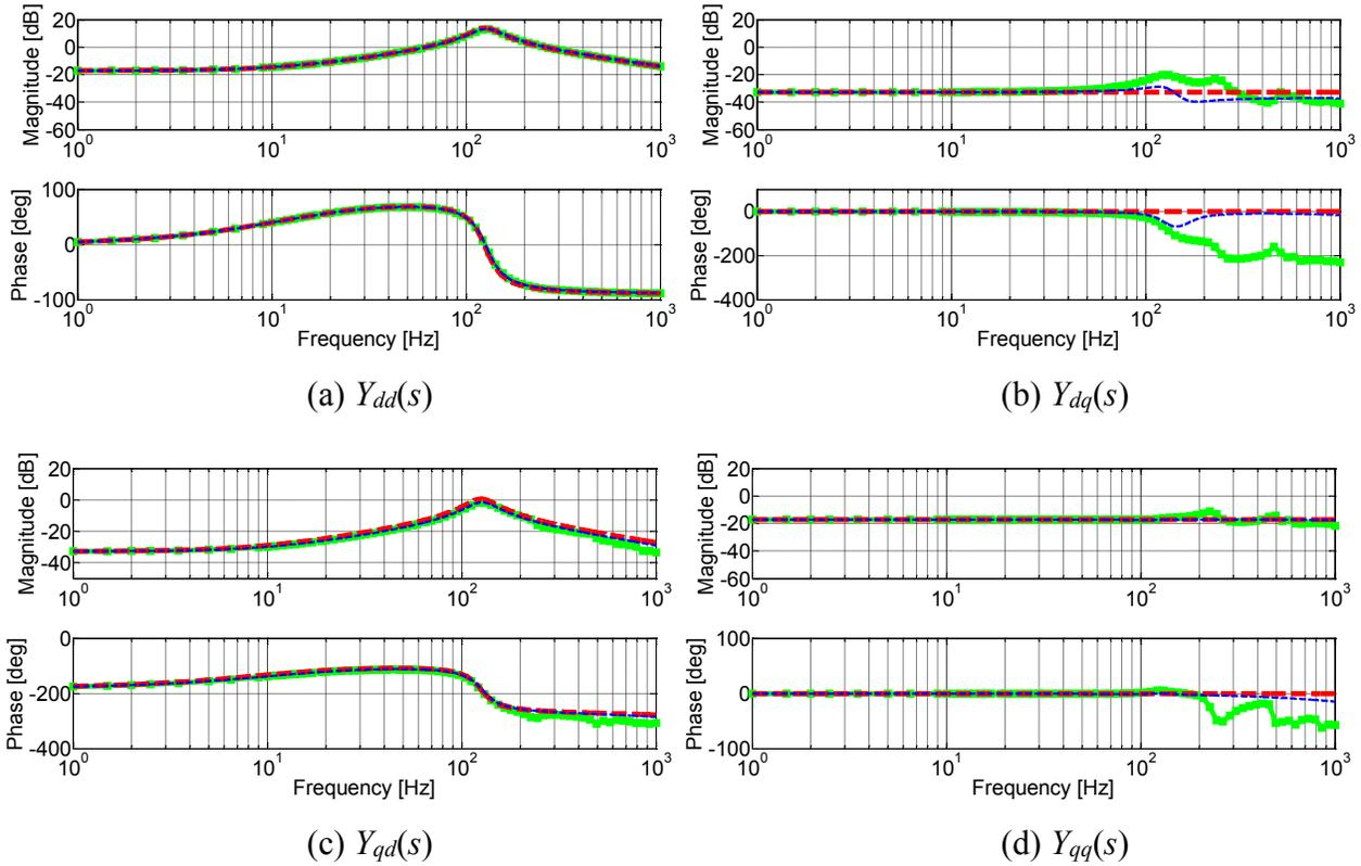
**Figure 3-7: Diode rectifier input dq admittances: switching model (green squared straight line), analytical expression of modified AAVM (red dashed line), analytical expression of PAVM (blue dashed line) (a)  $Y_{dd}(s)$  (b)  $Y_{dq}(s)$  (c)  $Y_{qd}(s)$  (d)  $Y_{qq}(s)$ .**
