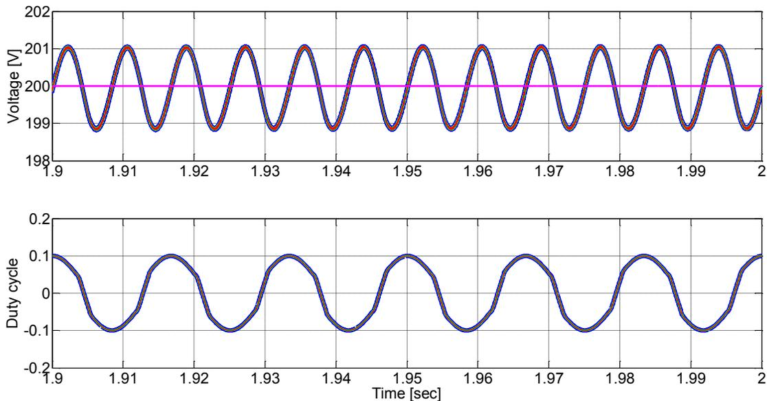
**Figure 6-13: Steady state simulation waveforms: (top) dc voltages  $v_{dc1}(t)$ ,  $v_{dc2}(t)$   $v_{dc3}(t)$  and dc reference voltage  $v_{dcref}(t)$  (bottom) H-bridge duty cycles  $d_1(t)$ ,  $d_2(t)$  and  $d_3(t)$**
