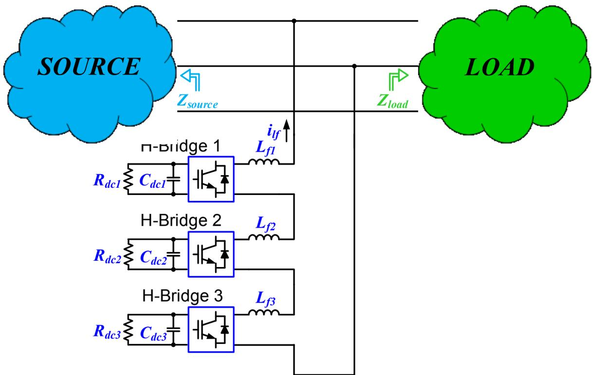
**Figure 5-1: Multi-level single-phase shunt current injection converter based on cascaded H-bridge topology**
