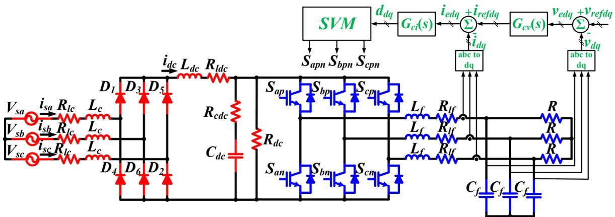
Figure 3-10: Circuit schematic of a six-pulse diode rectifier feeding a three-phase voltage source inverter
