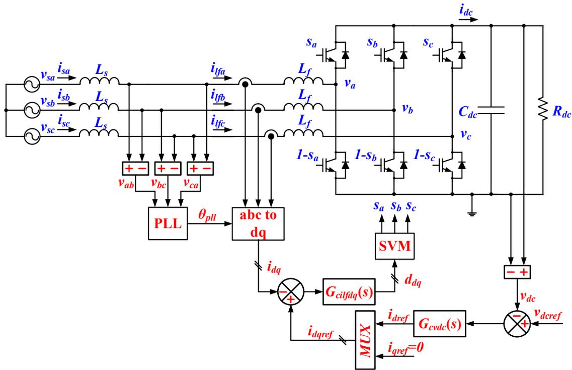
Figure 2-18: Switching model schematic of three-phase boost rectifier
