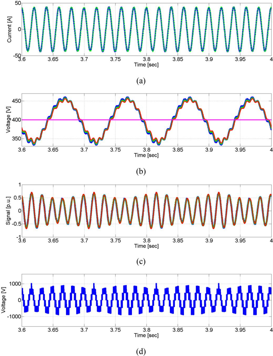
**Figure 5-13: Simulation waveform signals for 30A rms, 50 Hz sinusoidal current injection operating point (a) inductor current  $i_{ij}(t)$  and current reference  $i_{ref}(t)$  (b) dc voltages  $v_{dc1}(t)$ ,  $v_{dc2}(t)$ ,  $v_{dc3}(t)$  and dc voltage reference  $v_{dcref}(t)$  (c) duty cycles  $d_1(t)$ ,  $d_2(t)$ ,  $d_3(t)$  (d) switching voltage  $v_{dcsw}(t)$ .**
