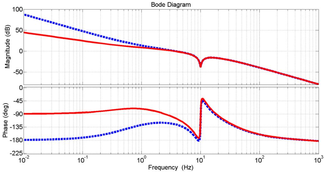
**Figure 5-12: Bode plots of dc voltage loop gain transfer functions:  $T_{vdc}(s)$  (straight red line) and  $T_{vdcdef}(s)$  (dashed blue line)**
