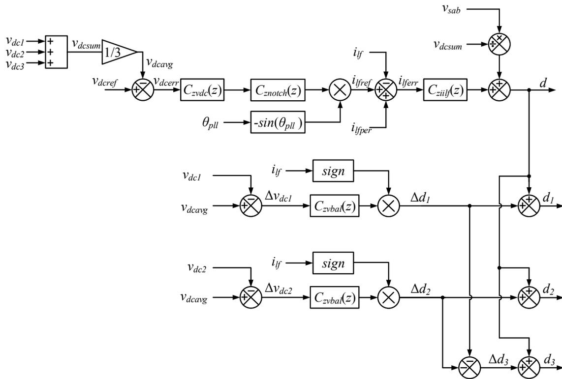
Figure 5-4: Block diagram of digital controller including high bandwidth current control, dc voltage regulation and voltage balancing among modules
