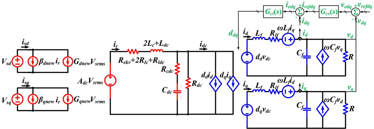
**Figure 3-11: Circuit schematic of AAVM of six-pulse diode rectifier feeding a three-phase voltage source inverter**
