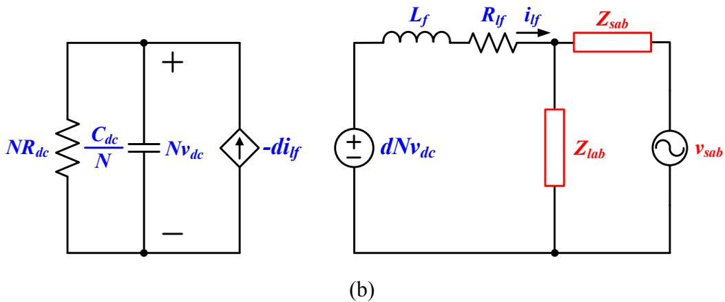
**Figure 5-7: Reduced order modeling of multi-level cascaded H-bridge converter (a) switching model (b) averaged model**
