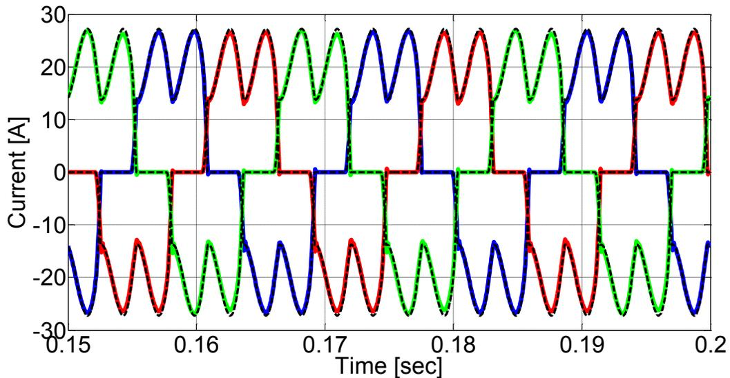
**Figure 3-8: Time-domain comparison of simulation model (dashed black line) with hardware waveforms (straight blue, red and green lines)**
