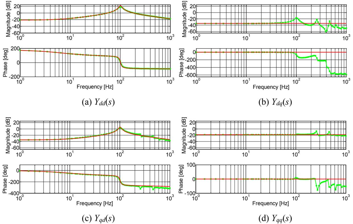
**Figure 3-12: Input dq admittance of diode rectifier feeding a constant power load obtained from the switching simulation model (green straight line with squares) and by linearization of averaged model (red straight line) (a)  $Y_{dd}(s)$  (b)  $Y_{dq}(s)$  (c)  $Y_{qd}(s)$  (d)  $Y_{qq}(s)$**
