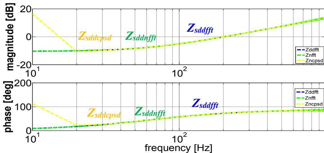
Figure 2-24: Source impedances  $Z_{sdd}$  comparison for FFT and CPSD algorithms
