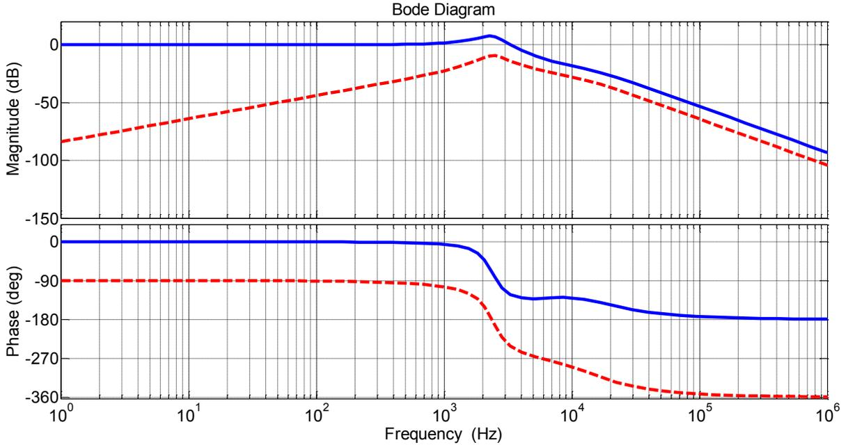
**Figure 6-7: Bode diagrams of the closed loop transfer function (a)  $G_{clif1}(s)$  (straight blue line) (b)  $G_{clif2}(s)$  (dashed red line)**
