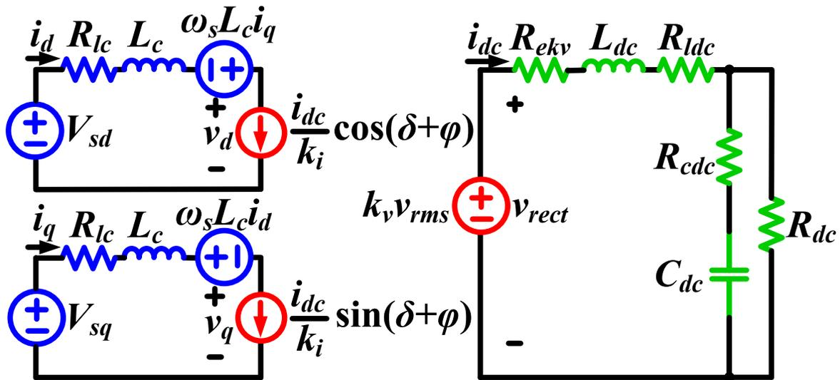
**Figure 3-5: Equivalent circuit schematic representation of PAVM**
