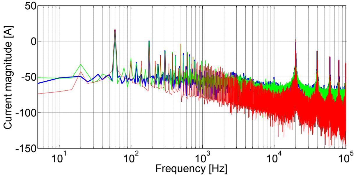
**Figure 6-25: Spectrum comparison of inductor current  $i_{l1}(t)$  no injection (blue line), 500 Hz injection (green line) and simulation current waveform (red line).**
