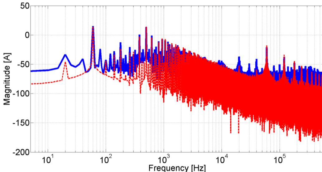
**Figure 5-17: Spectral content comparison of inductor current  $i_{lf}(t)$  obtained via simulation (dashed red line) and experiment (straight blue line).**
