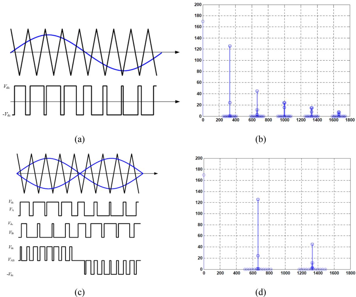
**Figure 5-2: Unipolar PWM technique (a) time-domain waveforms (b) frequency-domain content, and bipolar PWM technique (c) time-domain waveforms (d) frequency-domain**
