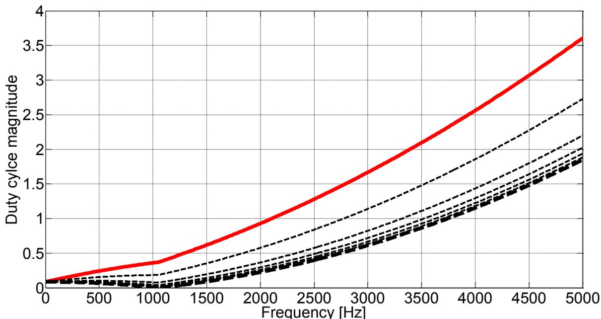
**Figure 6-4: Duty cycle injection magnitude versus injection frequency for different values of equivalent system impedance:  $Z_e=1 \Omega$  (red straight line),  $Z_e$  increases (black dashed lines)**
