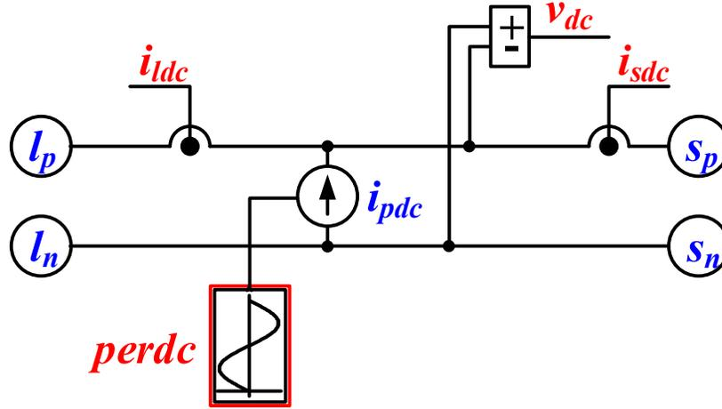
Figure 2-10: Shunt current injection dc measurement block
