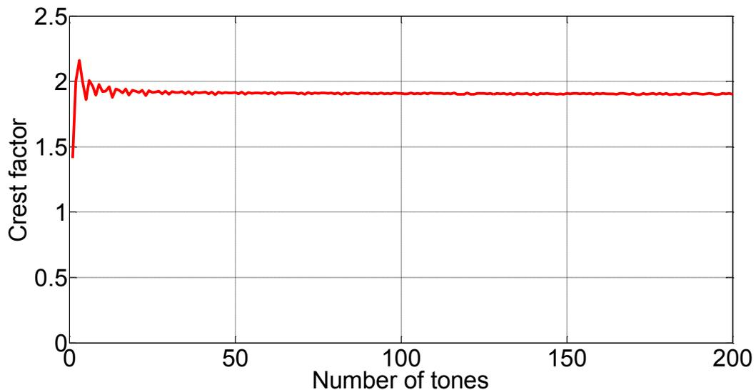
**Figure 2-3: Crest factor of the multi tone with respect to the number of frequency points**
