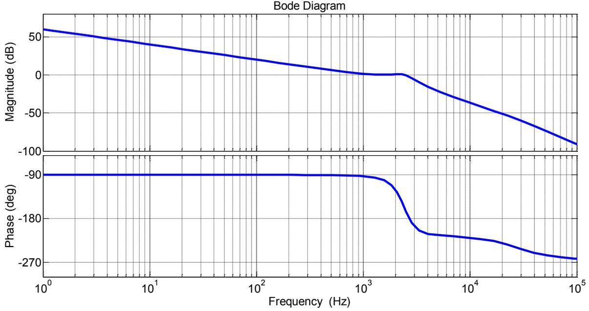
**Figure 6-10: Bode diagram of the voltage loop gain transfer function  $T_{vcf}(s)$**
