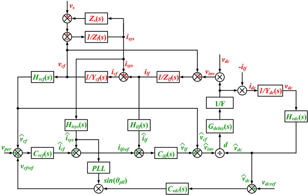
**Figure 6-6: The block transfer function diagram of the reduced order model of SVI converter**
