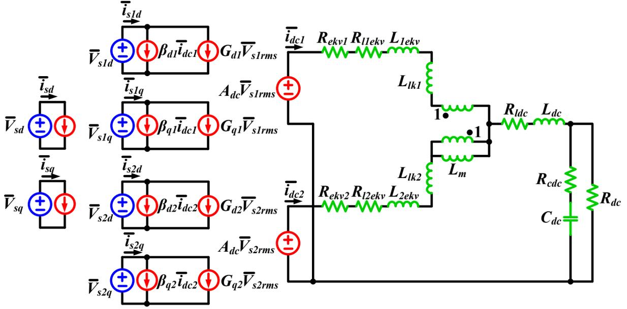
Figure 4-2: Averaged model of twelve-pulse diode rectifier with resistive load.
