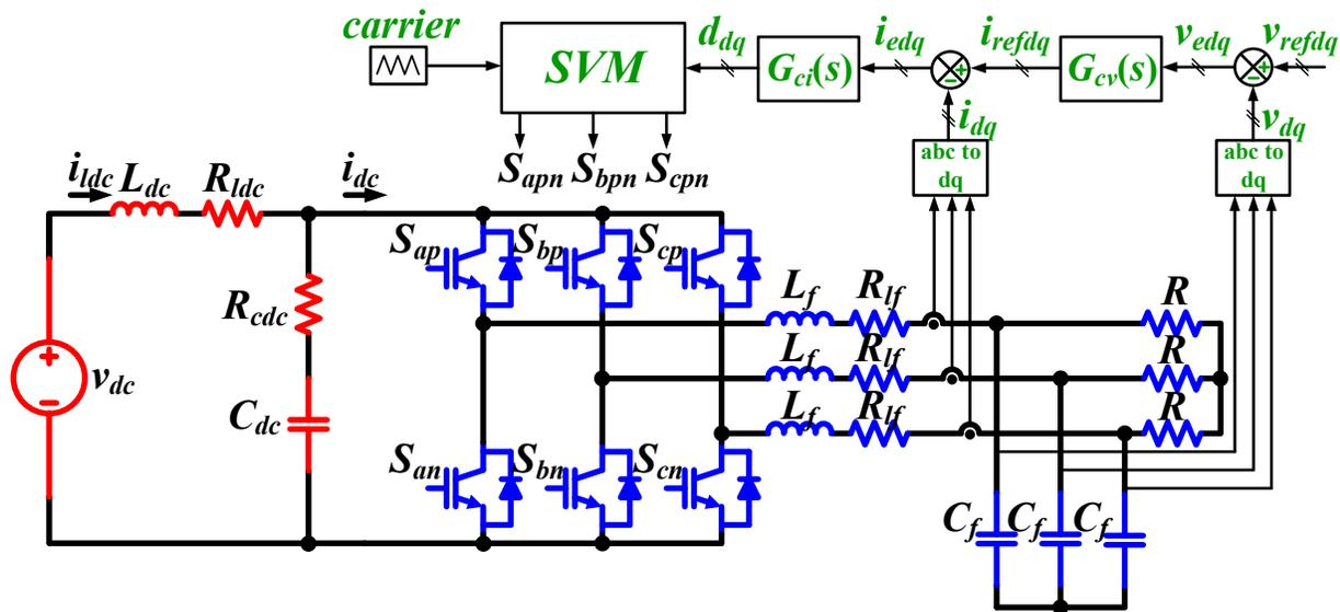
Figure 2-14: Switching model schematic of three-phase VSI
