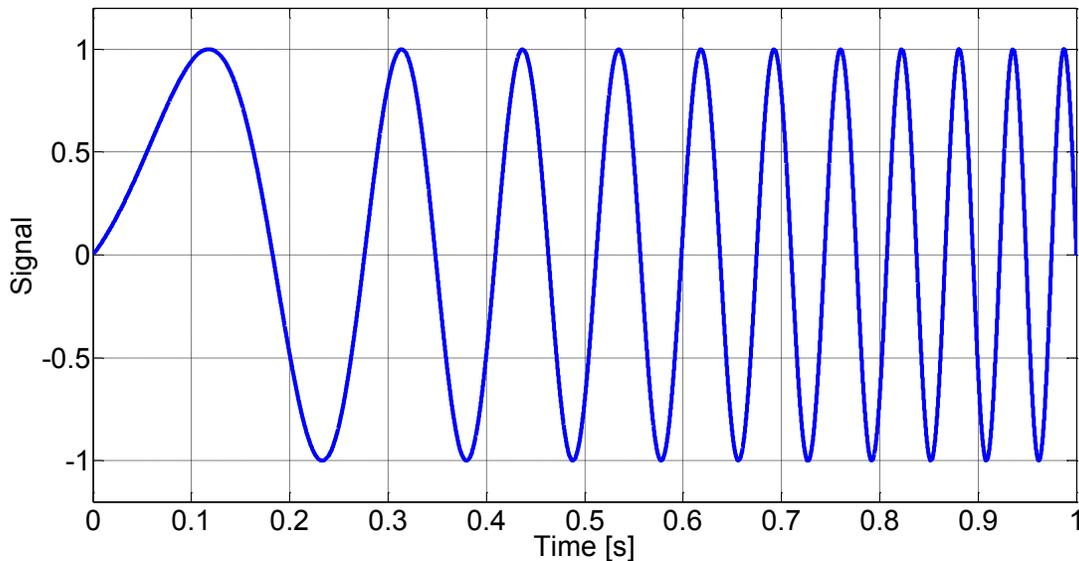
**Figure 2-4: Time domain waveform of chirp signal  $f_0=1, f_1=20, T=1$**
