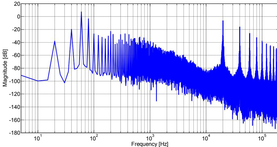
**Figure 6-19: Harmonic spectrum of the inductor current  $i_{lf1}(t)$**
