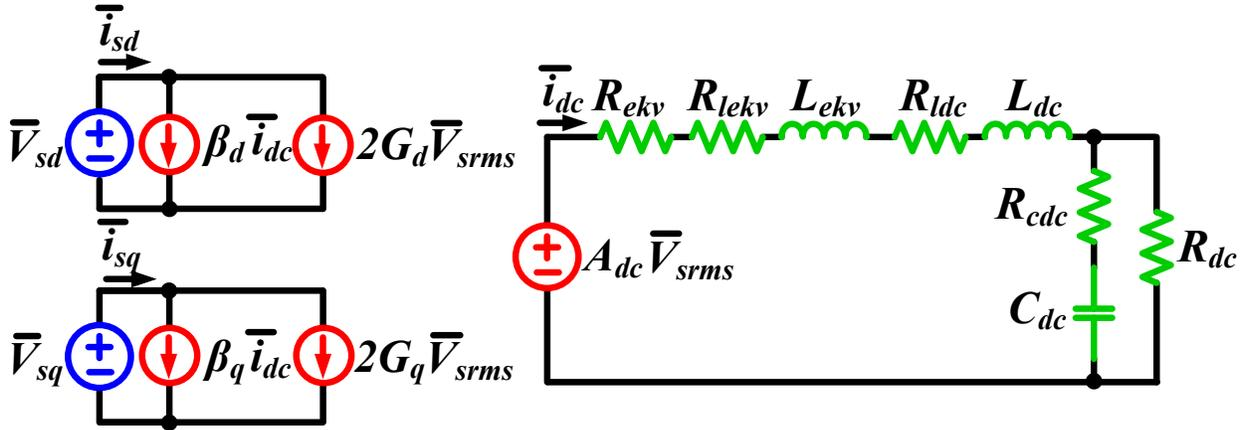
**Figure 4-4: Circuit schematic of further simplified AAVMs of twelve-pulse diode rectifier feeding a resistive load.**
