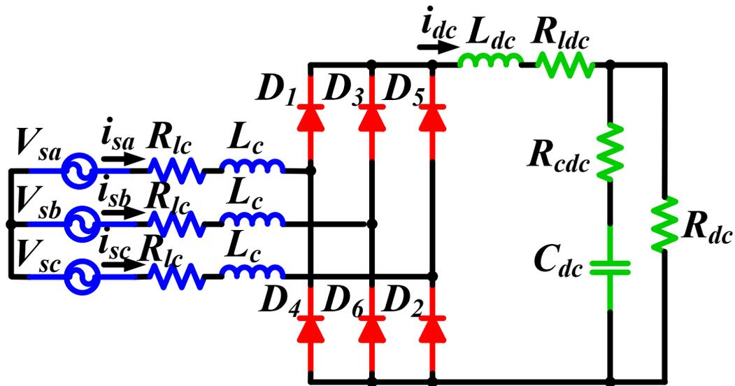
**Figure 3-1: Schematic of six-pulse diode rectifier with resistive load.**
