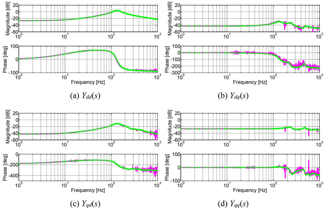
**Figure 3-9: Input dq admittance of six-pulse diode rectifier obtained from the switching simulation model (green squared line) and by hardware measurements (purple straight line) (a)  $Y_{dd}(s)$  (b)  $Y_{dq}(s)$  (c)  $Y_{qd}(s)$  (d)  $Y_{qq}(s)$ .**
