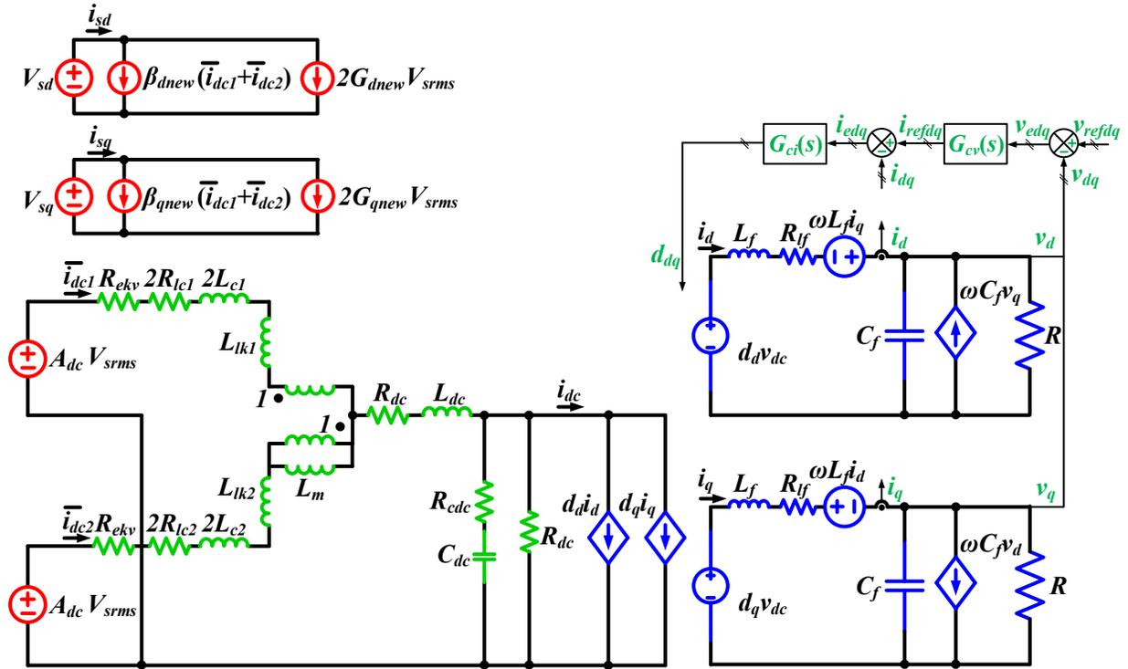
**Figure 4-8: Reduced order AAVMs of twelve-pulse diode rectifier feeding an actively controlled three-phase VSI**
