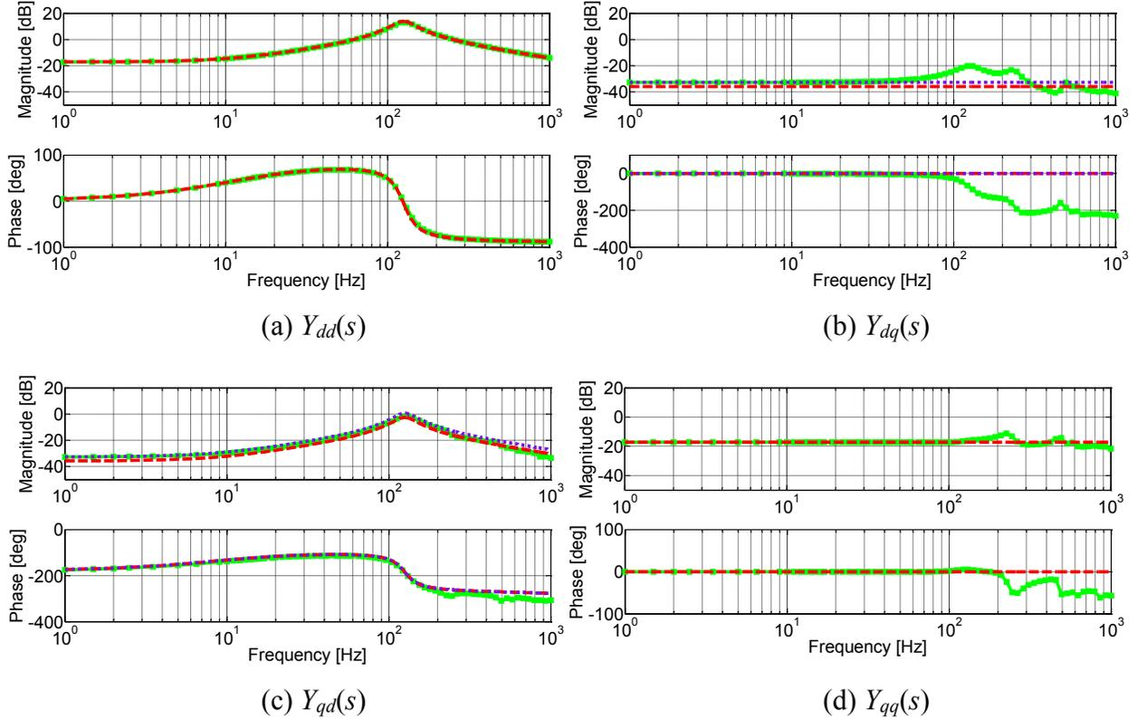
**Figure 3-3: Small-signal input dq admittance of six pulse diode rectifier: obtained from switching simulation model (green line with squares), analytical expression of modified AAVM (red dashed line) and scaled up expressions of modified AAVM (purple dashed line).**
