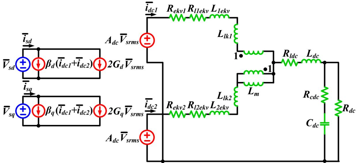
**Figure 4-3: Circuit schematic of simplified AAVMs of twelve-pulse diode rectifier feeding a resistive load.**
