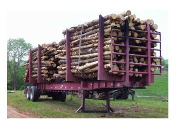
This truck is loaded with small-diameter pine tree logs called "pulpwood" that are headed to a pulpwood-using plant to make cardboard, paper, and other cellulose-based products
