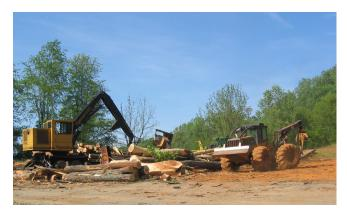
A log loader is stationed on the log deck and is used to load the sorted logs onto trucks. Sometimes logs are sorted for going to different mills, and the loader may also be equipped to delimb trees and cut them to length.
