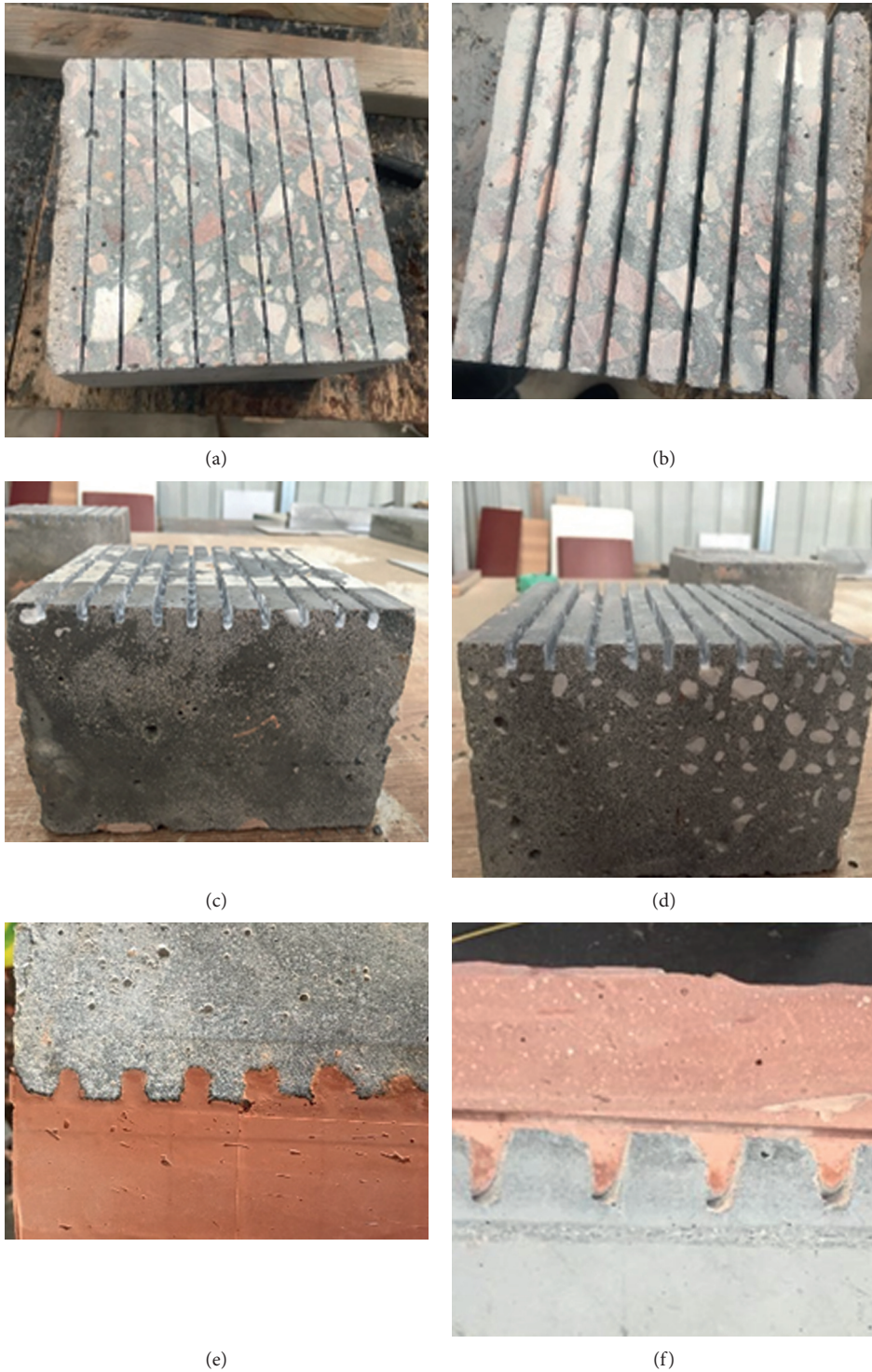
FIGURE 4: Different parallel groove depths and the geopolymer coating: (a) (b) (c) (d) 5 mm depth groove; (e) 5 mm depth parallel groove with geopolymer coating; (f) 8 mm depth parallel groove with geopolymer coating.
