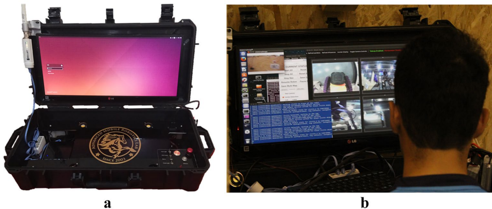
Fig. 15 a The operator control unit of the robot, and b the operating controlling the robot
