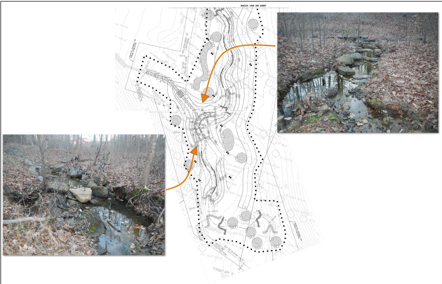
Figure 4.3 Design plan drawings and field pictures of a step pool structure in Project 25. The orange arrows indicate the direction the photographer was facing.
