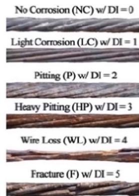
Figure 2.6. Strand damage conditions (Naito et al., 2011)
