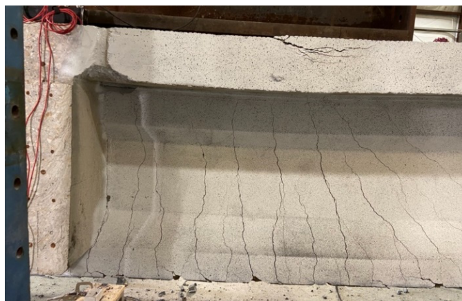
Figure 5.19. Concrete Crushing Failure Mode and Cracking Pattern
