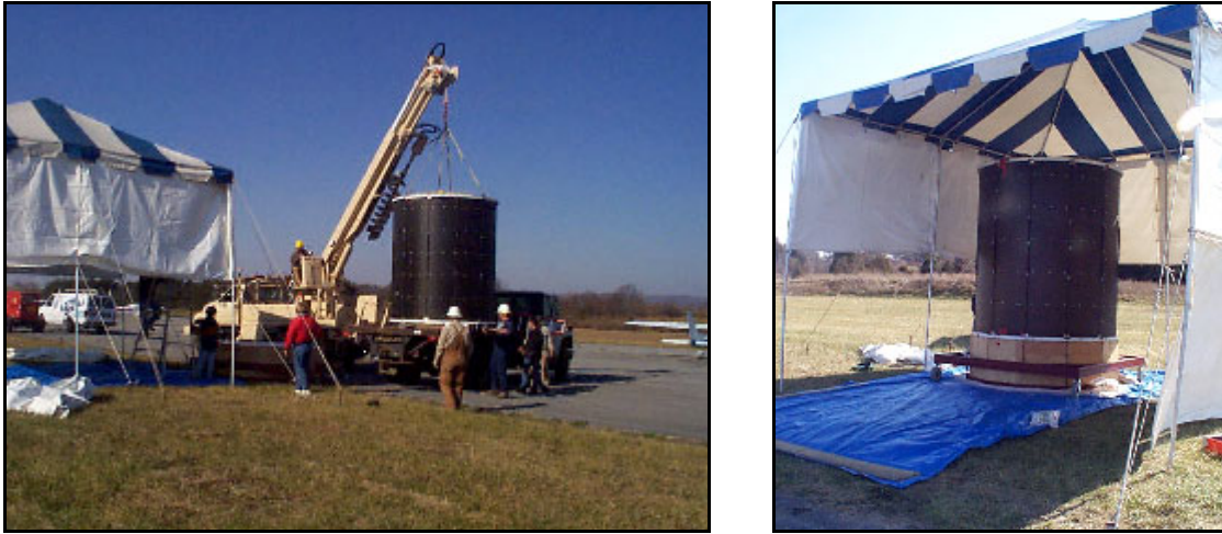
Picture 4.1 Cylinder being craned onto the base and then placed under the large tent at the outdoor test site.
