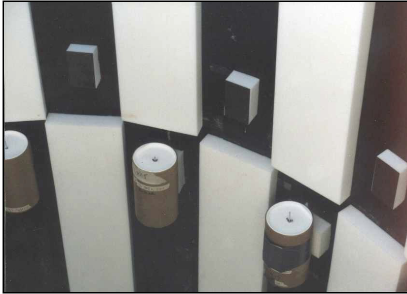
Picture 4.7 HR/DVAs and DVAs spaced every 24^\circ around the mid point up the cylinder
