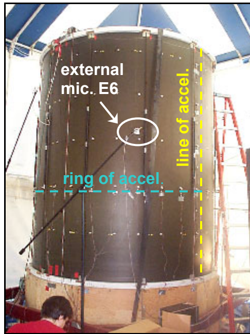
Picture 4.3 Instrumented cylinder showing the accelerometers and one of the external monitoring microphones
