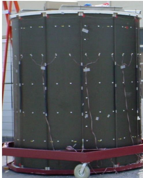
Figure 3.10 Boeing composite cylinder on its dolly with the 5 rings of 30 accelerometers.
