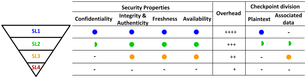
Fig. 4. Proposed levels for checkpoint security with an decreasing overhead for securing checkpoint and decreasing guarantees for security properties from SL1 to SL4. The decreasing overhead corresponds to the decreasing size of plaintext input in checkpoint partition, where larger plaintext input to AEAD increases overhead from encryption and decryption.
