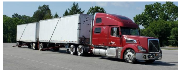
Figure 14. 33-ft A-double used for straight-line stopping tests
